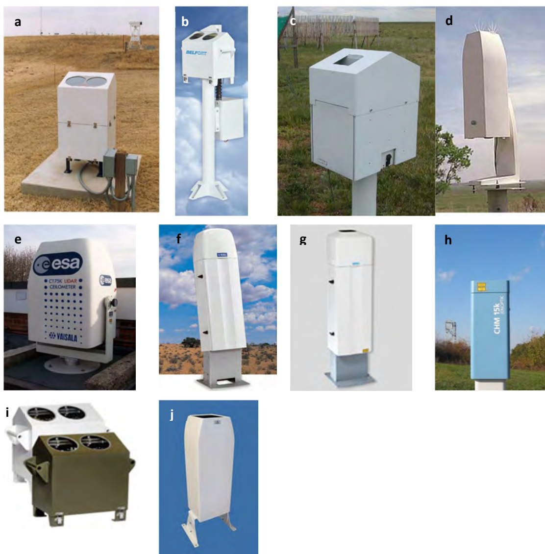
Figure 10. Different brands and models of ceilometers: a) Belfort Laser Ceilometer 7013C (U.S. DOE's ARM Program), b) 80171 Cloud Ceilometer (Belfort Instruments website), c) Vaisala CT12K Laser Ceilometer, d) Vaisala CT25K (U.S. DOE's ARM Program), e) Vaisala CT75K (British atmosphere datacenter website), f) Vaisala CL-31 (Vaisala website), g) Vaisala CL-51 (Vaisala website), h) Jenoptik CHM15K (Jenoptik website), i) Eliasson CBME80 ceilometers (Eliasson Engineering website), and j) ceilometer 8200-CHS (MTECH systems website).
