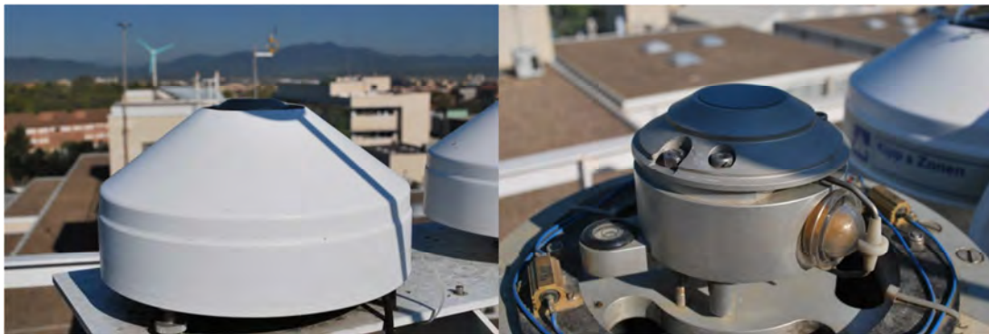
Figure 14. CG1 Kipp & Zonen pyrgeometer, which is mounted over a sun-tracker (Kipp & Zonen 2AP) with a sunblocker. It measures the infrared irradiance (spectral response between 0.3-2.2 \mu\text{m} ) and has an incidence field of view (IFOV) of 150°. This instrument is installed in Girona, Spain.
