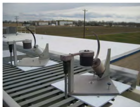
Figure 17. Multi-Filter-Rotating Shadowband Radiometers (MFRSR) installed at PNNL (Richland, WA).
