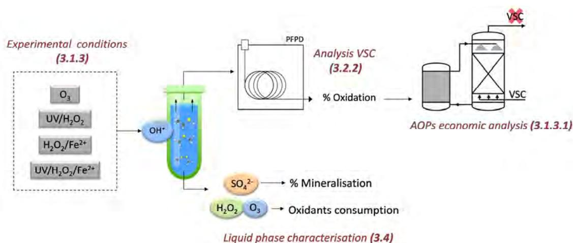
Figure 6.1 Diagram of methodology used in AOPs for VSC removal.
