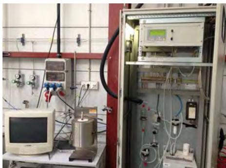
**Figure 3.14** Picture of infrared adsorption analyser
