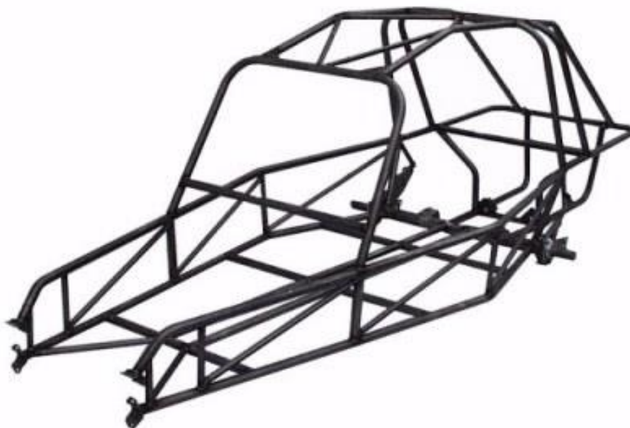
Figura B.3: Xassís tubular (Font: http://mudcars.com )
