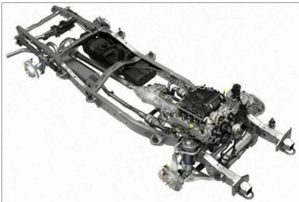
Figura B.1: Xassís independent (Font: http://www.elchapista.com )
