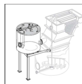
BOTH THE LT (ILLUSTRATED) AND LS CAN BE EQUIPPED WITH A FLOCCULATION TANK.
