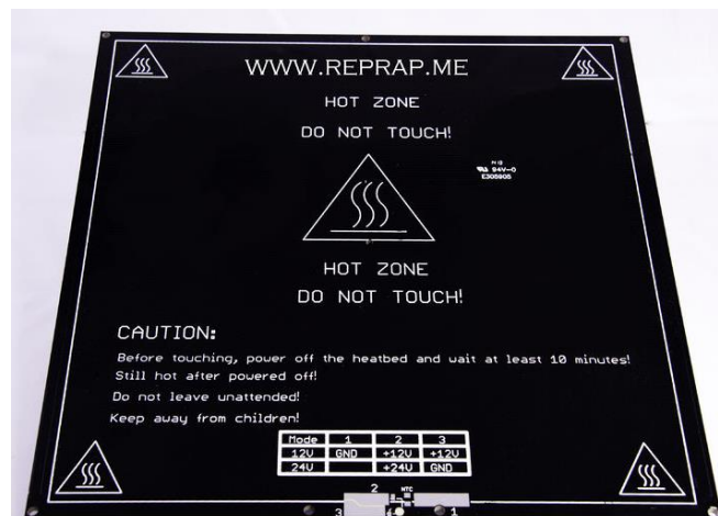
Figura. 56 Placa PCB MK3 Alu 200x200mm dual voltage
