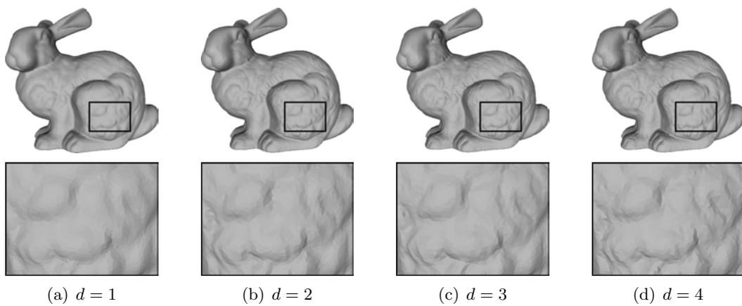
Figure 6.6: Stanford Bunny. Reconstructed surfaces with a gradual increase of the degree of the splats.
