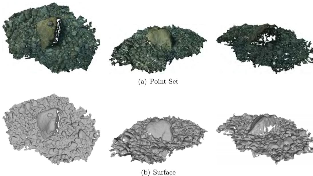
Figure 6.15: Shallow Water dataset, 863,162 points, (a) obtained through PMVS [84], and (b) the reconstructed surface using our method.
