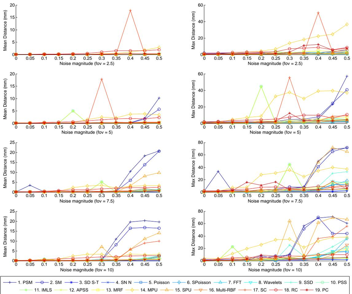
Figure 8.10: Individual results for the noise test on the **Max Planck** dataset. The laser beam's field of view is incremented from top to bottom. Line charts on the left show the mean distance results and the maximum distance on the right.
