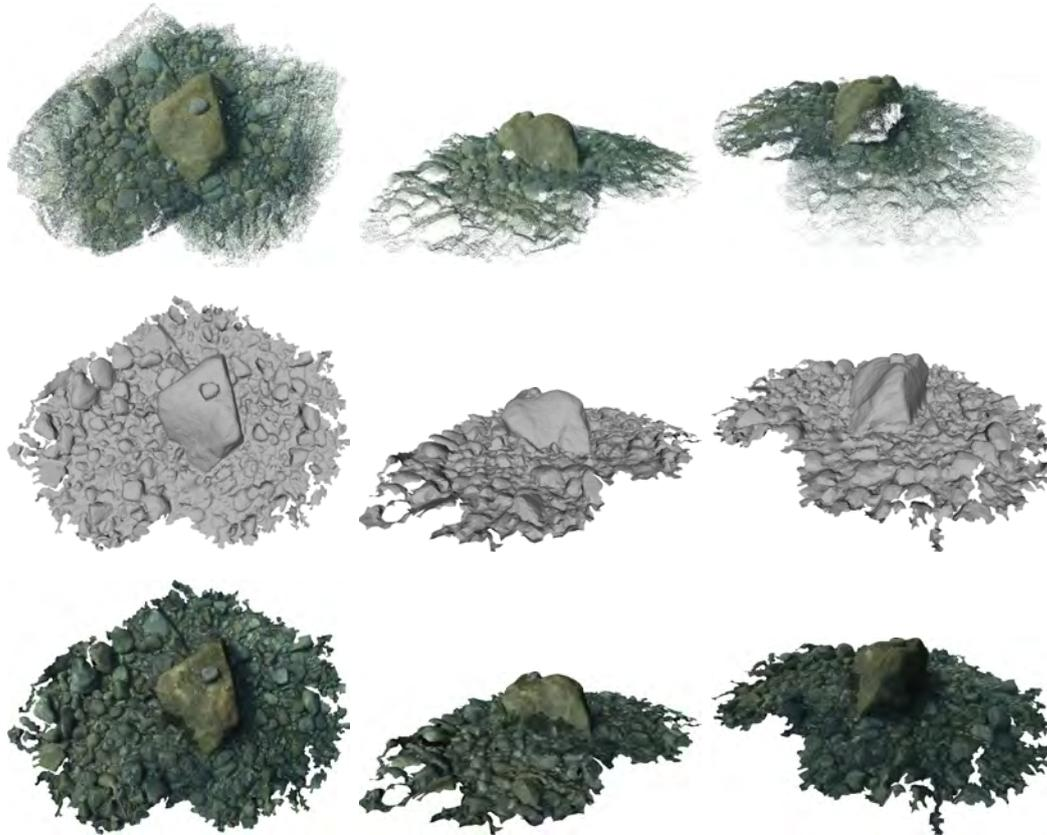
Figure 5.14: Shallow Water dataset reconstruction. From first to last row: point set (1,856,271 points), meshed surface, and textured surface.
