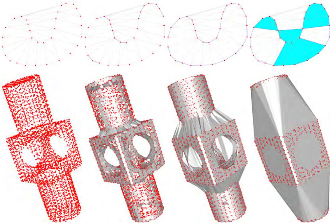
Figure 4.2: The  $\alpha$ -shapes [72] results for different values of  $\alpha$ , increasing from left to right (first row for 2D and second for 3D). In the 2D case, the Delaunay triangulation is marked in light gray, in order to show that the alpha shape is a subset of it. Note how alpha equals the point set itself for a sufficiently small  $\alpha$ , and converges to the convex hull of the points for a sufficiently large value.
