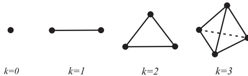
Figure 3.4: Examples of a  $k$ -simplex for  $k$  ranging from 0 to 3.
