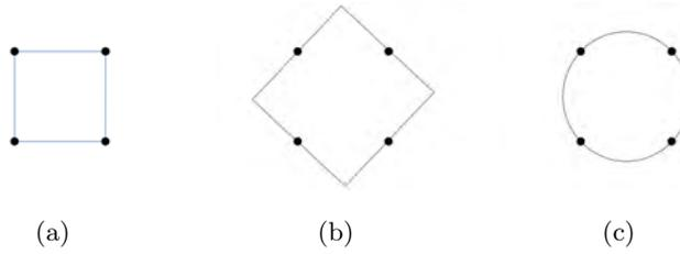
Figure 1.2: Illustrative example of the surface reconstruction problem being ill-posed. For easiness of depiction, the example is a curve reconstruction, the equivalent problem in 2D. Note how, given the set of points shown in black, one may define several curves passing on or near the points that might have generated this sampling.
