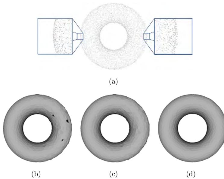
Figure 5.7: The noise corrupted version of the Torus dataset (a), causes the surface recovered by our method (b) to be bumpy and defected with holes. The hole filling (c) and smoothing (d) procedures allow the recovery of a more faithful approximation of the original object.
