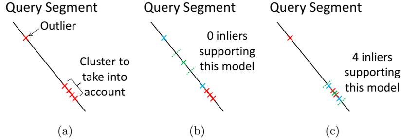
Figure 6.3: Robust intersection. (a) The splats that are coherent among each other generate a cluster of intersection points, while a non-coherent splat generates an isolated intersection point, classified as an outlier. (b) and (c) illustrate two possible iterations of the RANSAC algorithm, centroids (green) generated from outliers have weaker support than the ones generated from inliers.
