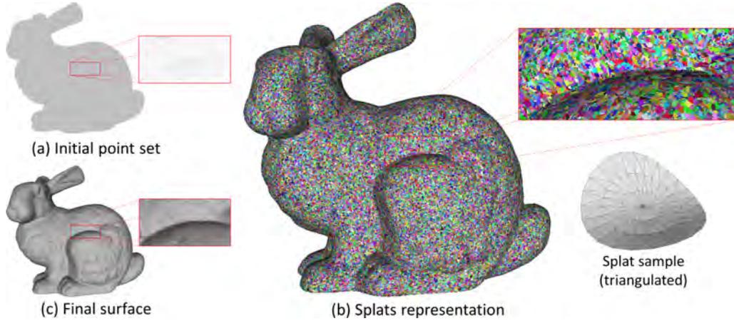
Figure 6.1: Overview of our method. (a) Input raw point set. (b) Splat representation (discretized using triangle fans for visual depiction). (c) Output surface triangle mesh generated through RDT Delaunay refinement.
