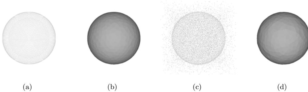
Figure 5.5: The Sphere dataset (10,242 points) shown in (a) is corrupted in (c) by adding a Gaussian displacement of  $\sigma = 0.01$  (w.r.t. the bounding box diagonal) to all the points and adding 100% of randomly uniform distributed outliers inside its slightly enlarged bounding box. The surface for the clean version and the corrupted one are shown in (b) and (d) respectively.
