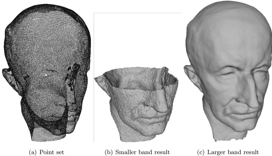
Figure 7.5: Relevance of the  $\sigma$  band size for the Normalized Cut method. When applied to a narrower  $\sigma$  band (b), the Normalized cut may be minimized by a cut that does not pass through the minimum of the UDF. By enlarging the  $\sigma$  band (c), the weight of the edges on each side of the partition increases, forcing the cut to pass through the minimum in UDF.
