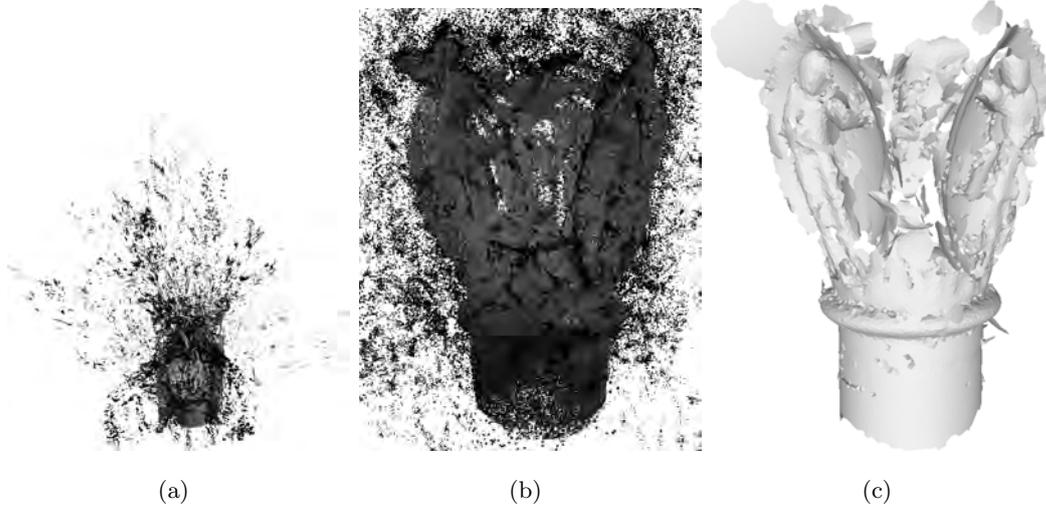
Figure 6.18: Column Capital optical dataset, 419,488 colored points. (a) Shows the full set of input points, (b) a closeup of the inlier area and (c) the surface obtained by our method.
