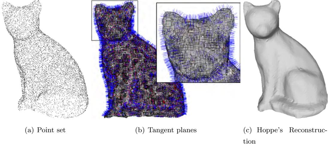
Figure 4.11: Hoppe's method [104] applied to the Cat dataset. From left to right, the input point set, a visualization of the tangent planes (as small patches, the blue vector denoting the normal direction) and the reconstruction result.
