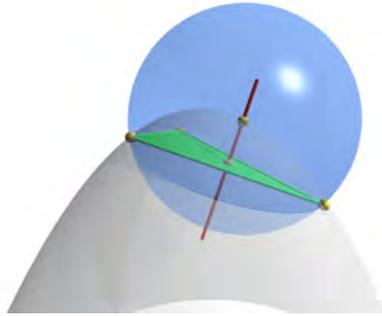
Figure 3.7: Example of a surface Delaunay ball.
