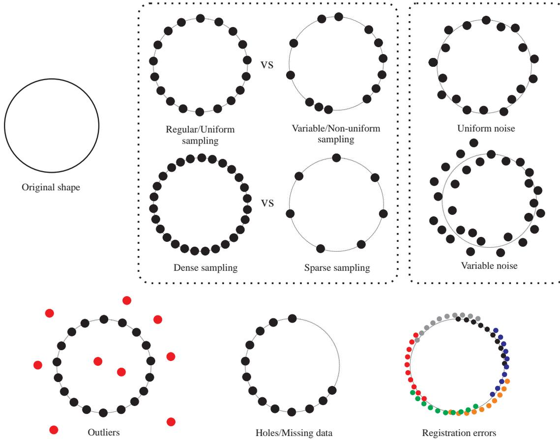
Figure 4.1: Common challenges in real point based datasets to be handled by surface reconstruction approaches.
