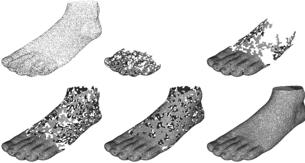
Figure 4.6: Various iterations of the Smooth Greedy algorithm [54]. Top-left corner shows the original point cloud, and then from left to right, top to bottom, different steps of the evolution of the greedy surface are presented.
