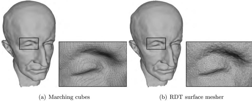
Figure 7.7: Comparison between Marching cubes (a) and RDT surface mesher (b) for the extraction of a surface. Note in (a) how the number of triangles is larger and their shape highly non-uniform, while they are better shaped (i.e., closer to regular) when using the RDT surface mesher. In both cases, the SDF used to extract the surface was constructed using the Normalized Cut method.
