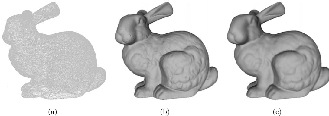
Figure 5.11: In (a), the Stanford Bunny dataset (362,272 points) is presented. Note in (b) how the recovered surface is quite bumpy near noisier areas. In (c), one can see the usefulness of the smoothing step in these cases.
