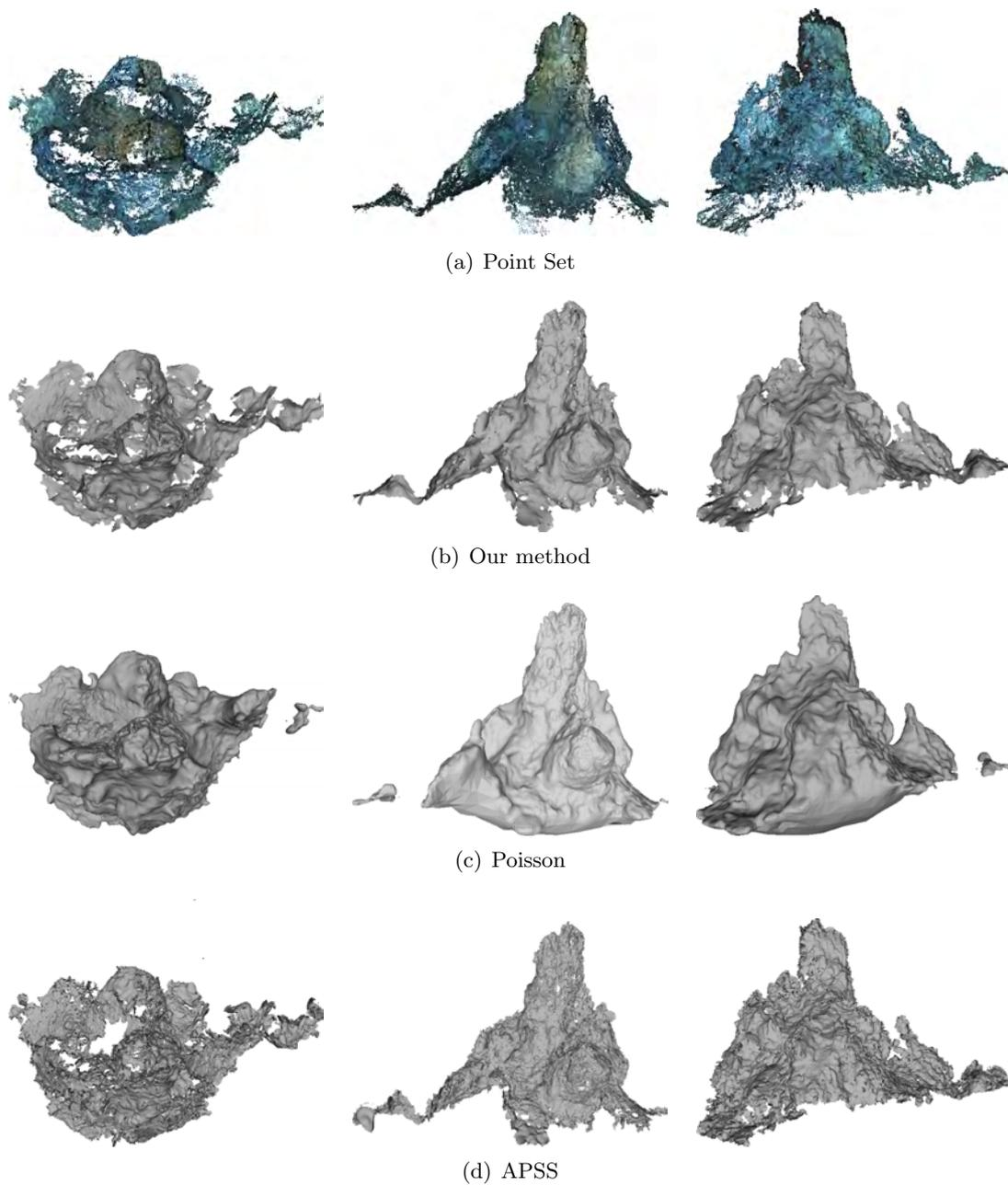
Figure 6.17: Tour Eiffel dataset, 168,502 colored points, (a) obtained using PMVS [84]. We used the point set in (a) with our method (b) and with Poisson [118] (c) and APSS [97]. One can observe that our method provides a smooth representation like Poisson, while recovering boundaries as with APSS.
