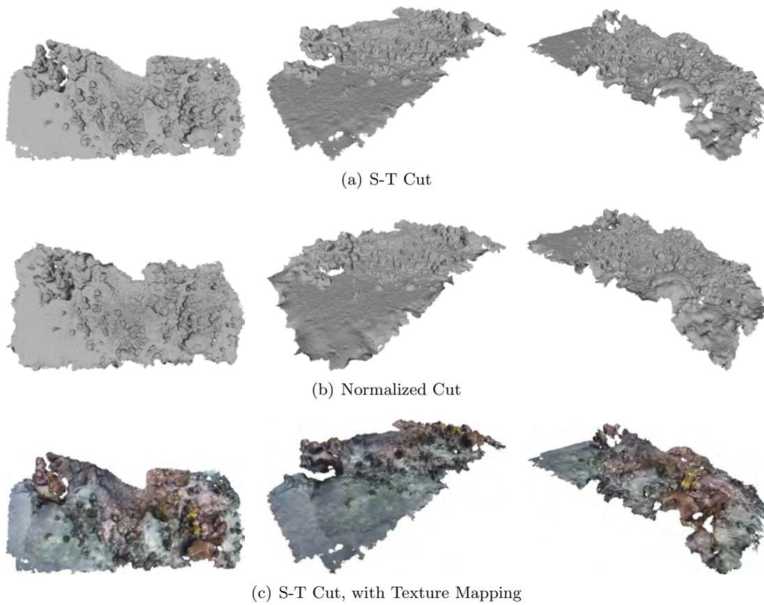
Figure 7.16: Coral Reef dataset, using S-T cut (a) and Normalized cut (b) algorithms. A texture mapped version of the S-T cut result is shown in (c).
