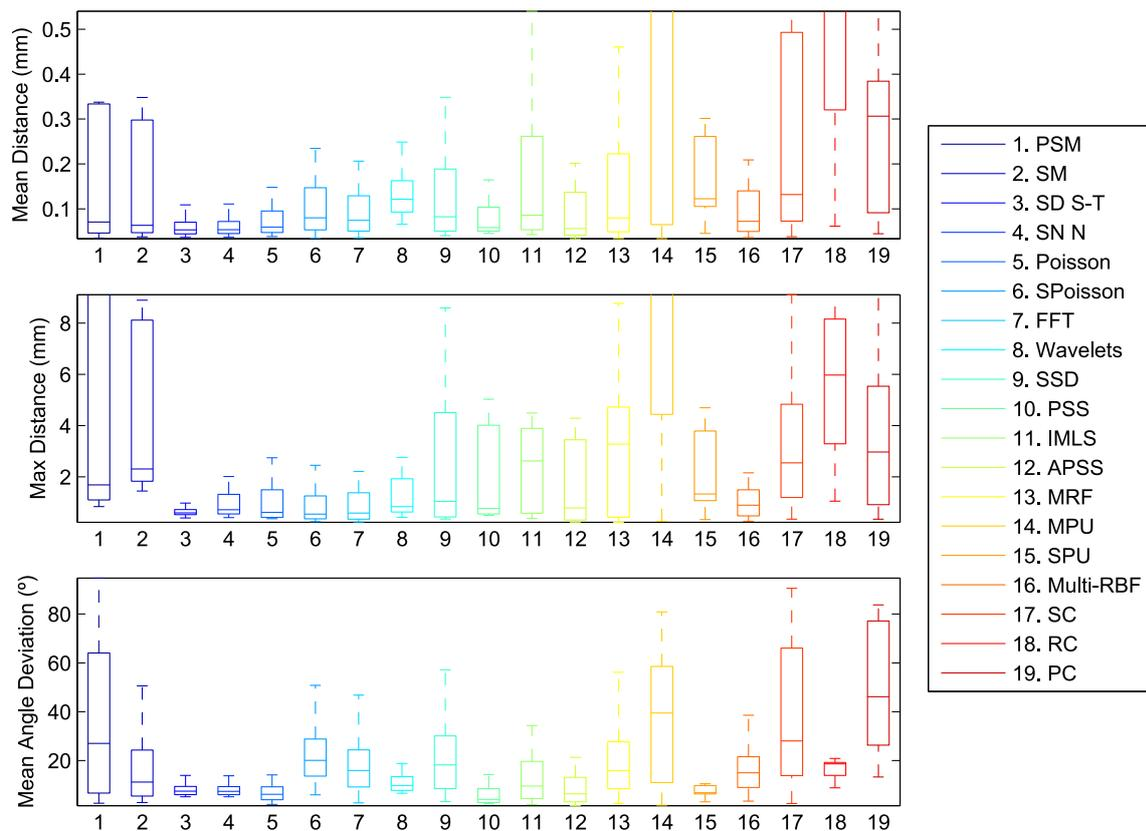
Figure 8.9: Error distribution plots for the noise test of the **Max Planck** dataset, using the benchmark by Berger et al.[22]. We show the mean and maximum (i.e., Hausdorff) distances, and the mean angle deviation for each method when applied to 44 synthetic scans with varying noise scales.
