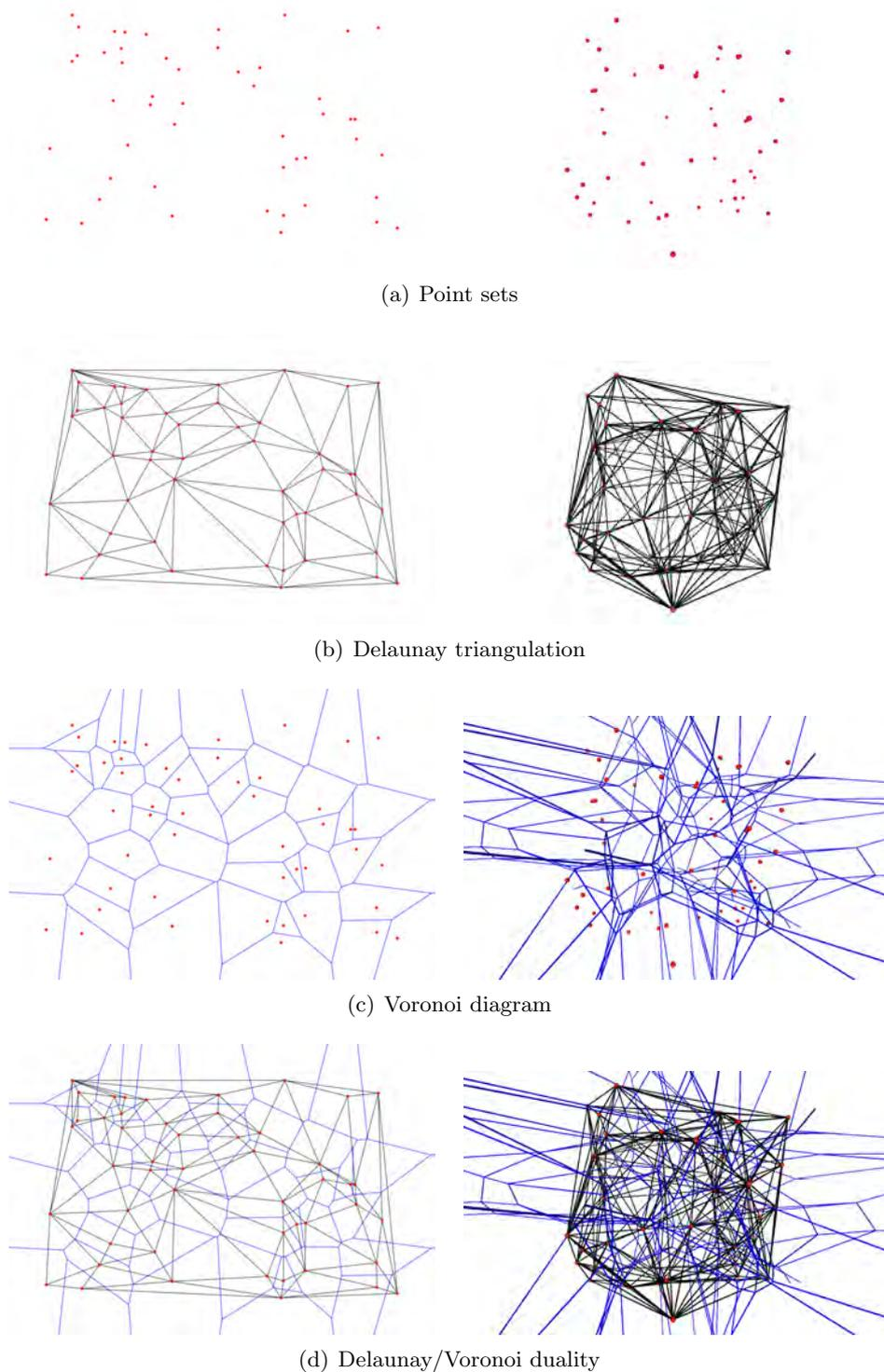
Figure 3.6: Sample of the Delaunay/Voronoi decompositions, with its duality relationships (left column in 2D and right column in 3D). From first to last row, we find the input point set, its Delaunay triangulation, the corresponding Voronoi diagram, and both constructions together (in order to show their duality).
