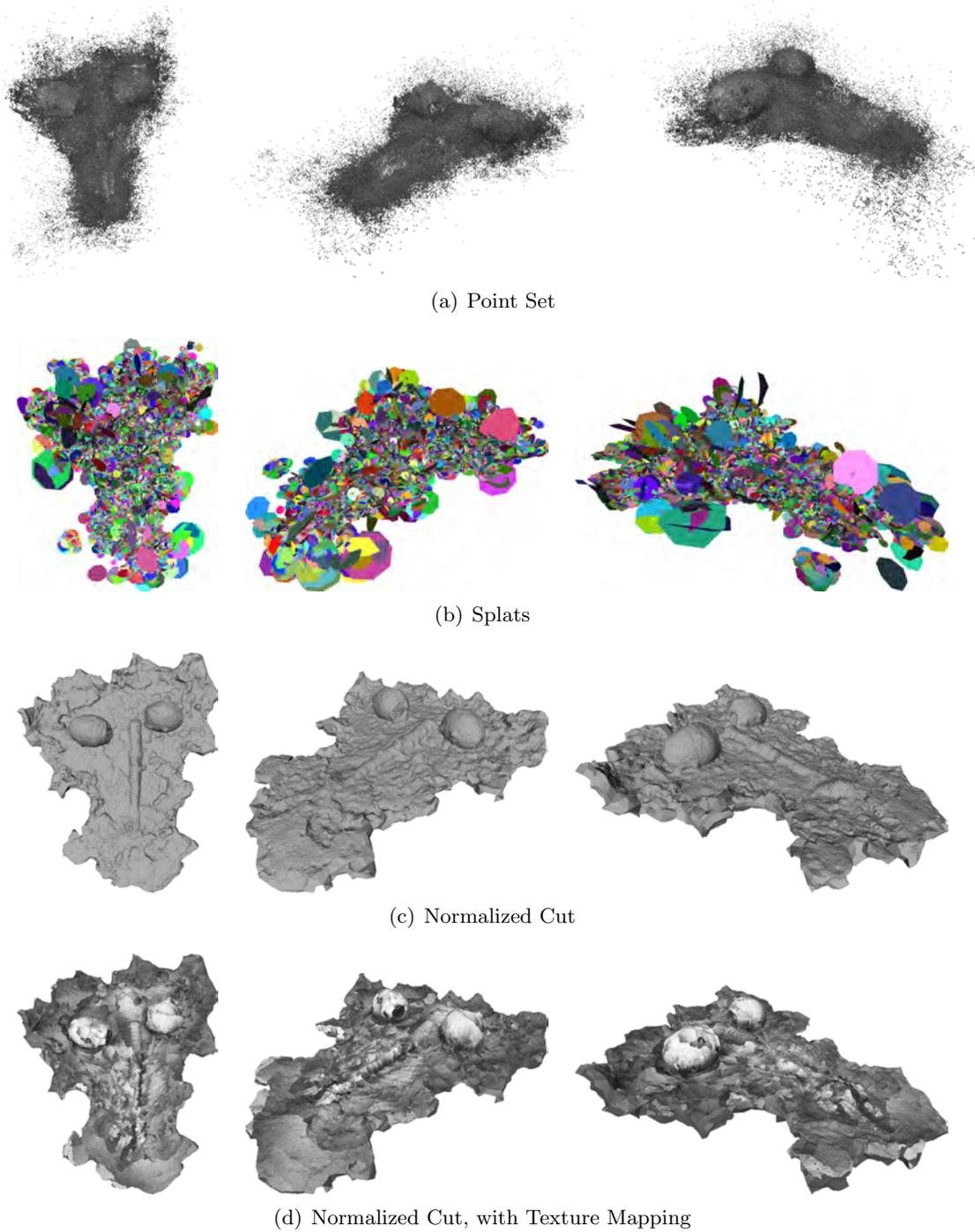
Figure 7.19: La Lune, second dataset. The point set in (a), and its splat representation in (b) show how this dataset reproduces the same level of corruption of the first dataset. The Normalized cut surface (c), and its texture mapped version (d), reveal two cauldrons located on either side of a cannon.
