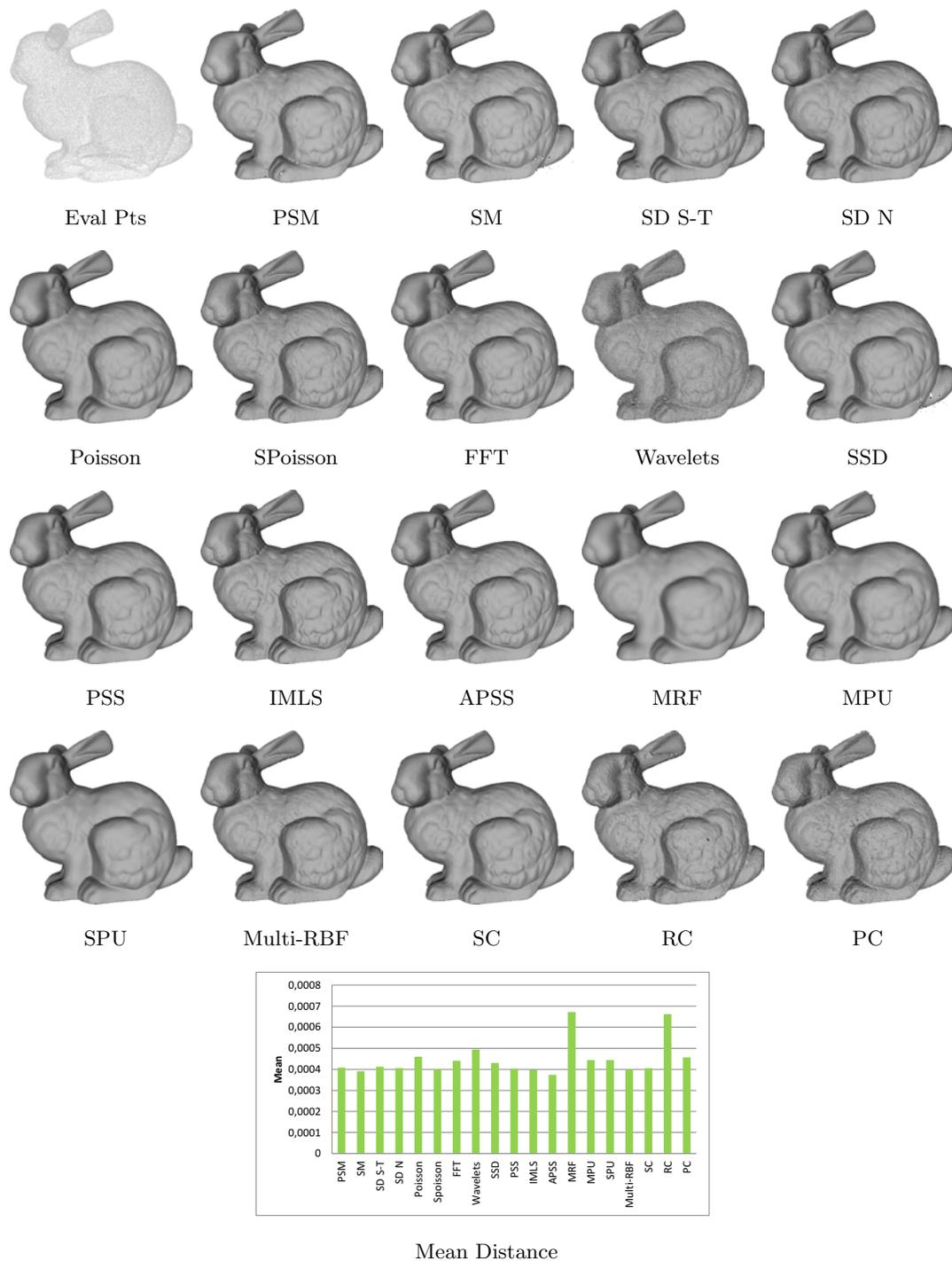
Figure 8.1: Real data tests, results for the Bunny dataset. Values with respect to the BBD.
