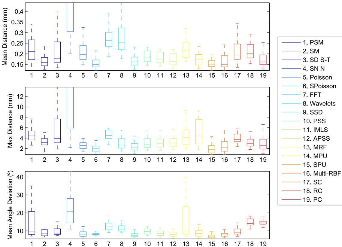
Figure 8.6: Benchmark by Berger et al.[22], results for the **Dancing Children** dataset. We show the mean and maximum (i.e., Hausdorff) distances, and the mean angle deviation for each method when applied to 48 synthetic scans generated using various scanning parameters.
