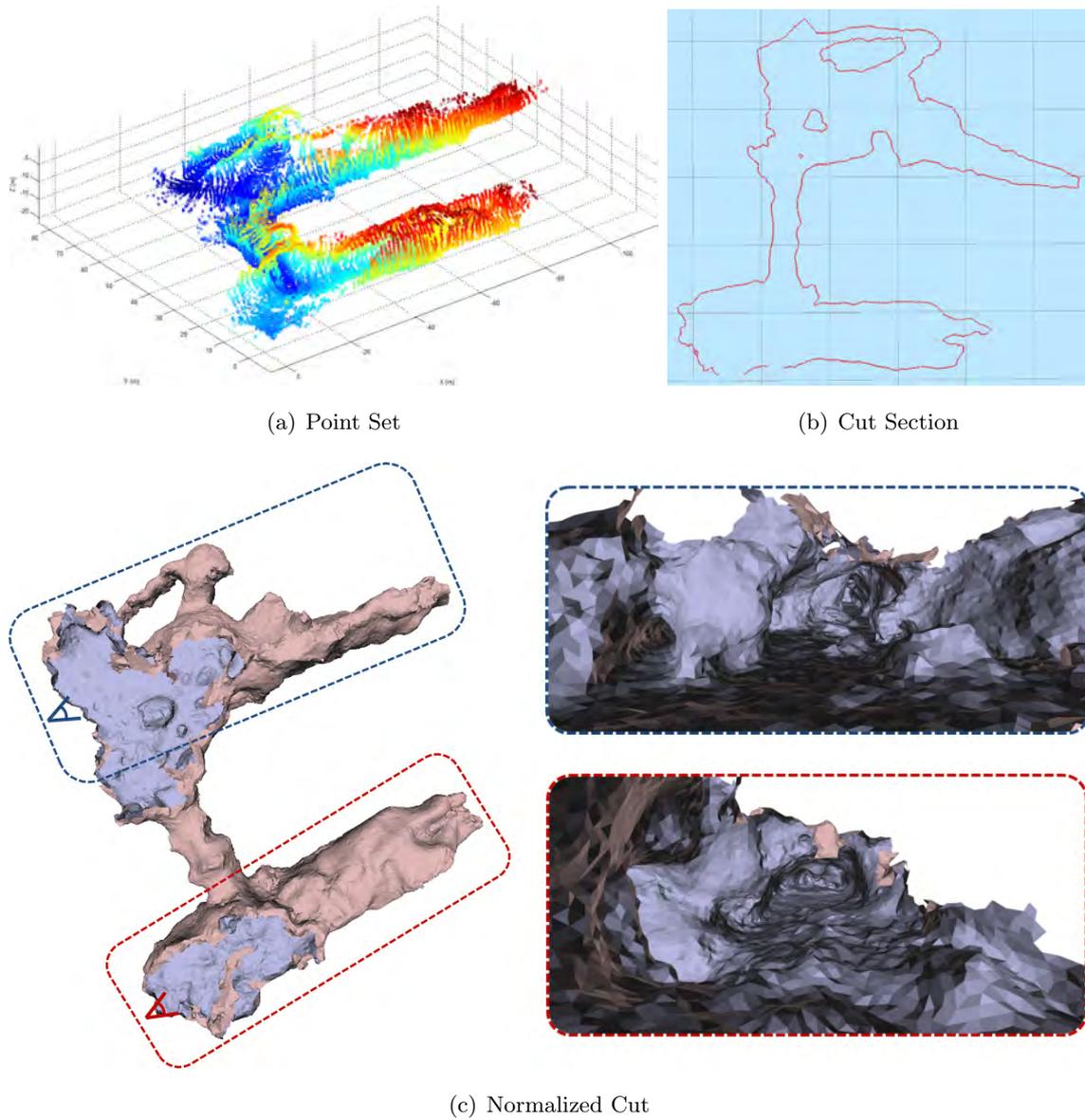
Figure 7.12: Profiling sonar survey of an underwater cave (a). In (c) one can see the reconstruction obtained by the Normalized cut algorithm, with close-ups of the two main tunnels highlighted. The view direction is also marked on the right part. Additionally, in (b) one can see a cross section of the cave to better understand the complexity of the area.
