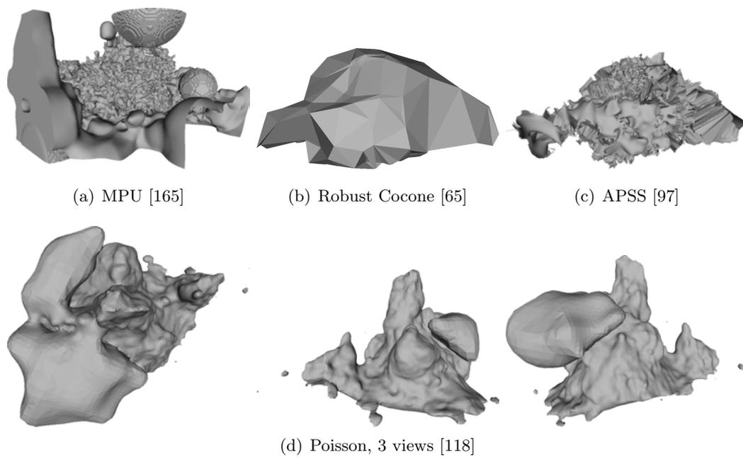
Figure 5.19: Results of some of the state-of-the-art surface reconstruction methods applied to the Tour Eiffel dataset. With the exception of Robust Cocone, all the methods tested require per-point normals, while our method does not. In all cases, we compute them using the method of [104] with a  $k = 100$ . Note how the original defect-laden point set prevents the reconstruction of a correct surface in (a)(b) and (c), while producing artifacts in (d).
