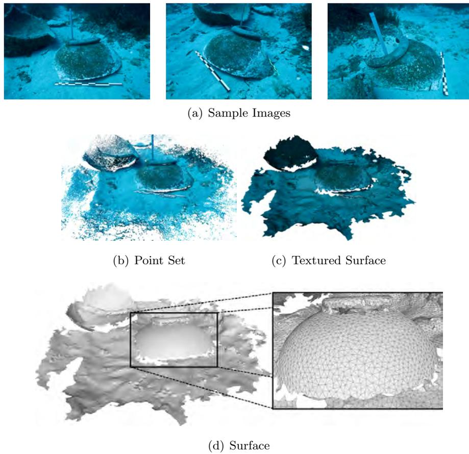
Figure 5.24: Pottery dataset. The first row (a) shows some input images (from a total of 39). We present the input point set (1,278,499 points) in (b), the reconstructed surface in (d) and its texture mapped version in (c). Note how, given less noisier conditions, the retrieved surface is smooth and faithfully represents the geometry of the observed object.
