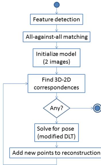
Figure 2.9: Pipeline followed by the incremental Structure-from-Motion approach used in this thesis.
