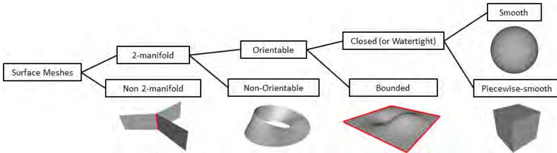
Figure 3.3: A sample of surfaces classified using the criteria described in section 3.2.2.
