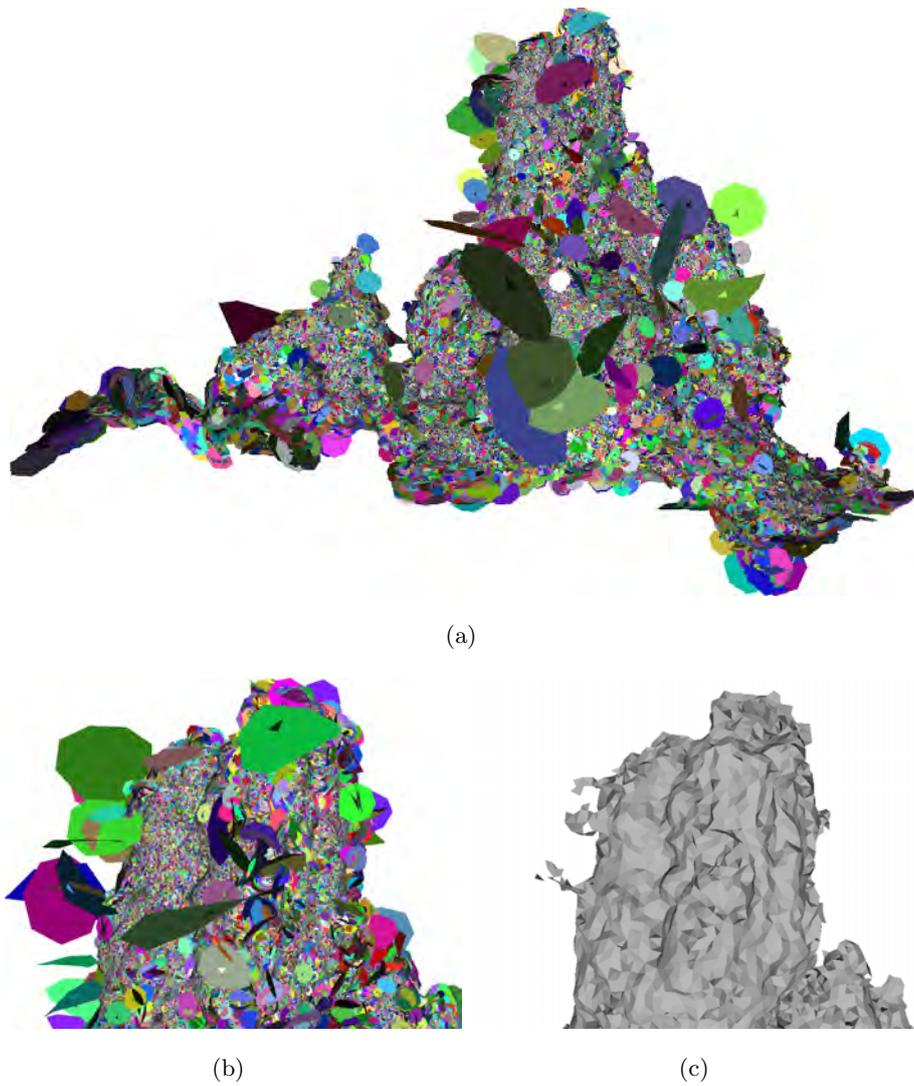
Figure 6.21: Splat representation (a), and close-up of the top part of the Tour Eiffel dataset, showing the splat representation (b) and the recovered surface (c). Note how the surface is almost completely recovered even with the erroneous splats generated by the outliers near high curvature areas.
