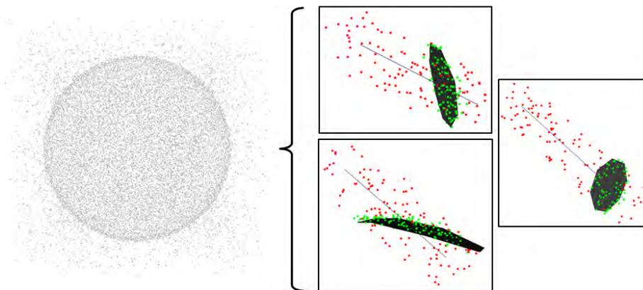
Figure 5.2: On the right are three examples of query segments required by the RDT algorithm to mesh the surface represented by the highly corrupted set of points on the left (a sphere), and the recovered local surfaces computed by our method used to solve the intersection computation. The results of our method applied to this point set can be found in Section 5.5.1.
