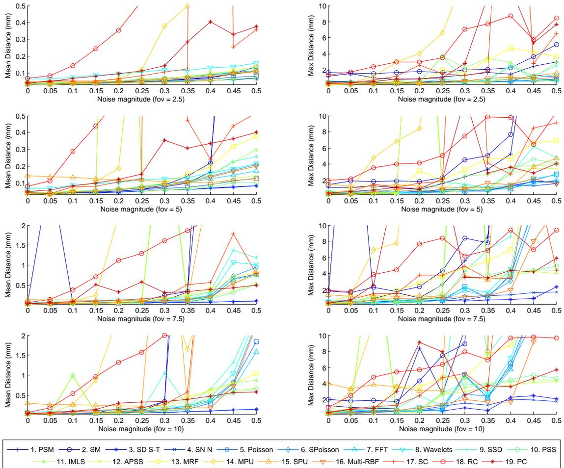
Figure 8.11: Close-up view of the individual results for the noise test on the **Max Planck** dataset. This restricted visualization allows us to observe the details of the results presented. Again, the laser beam’s field of view is incremented from top to bottom, and the line charts on the left show the mean distance results, while the ones on the right depict the maximum distance.
