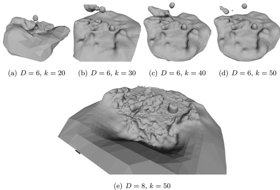
Figure 5.23: La Lune dataset, results using the Poisson method [118]. In each figure,  $D$  stands for the octree depth required for Poisson, and  $k$  for the number of neighbors to take into account during Hoppe’s normal computation method. Note in the top row how different  $k$  values during normal inferring modify the output of the Poisson method.
