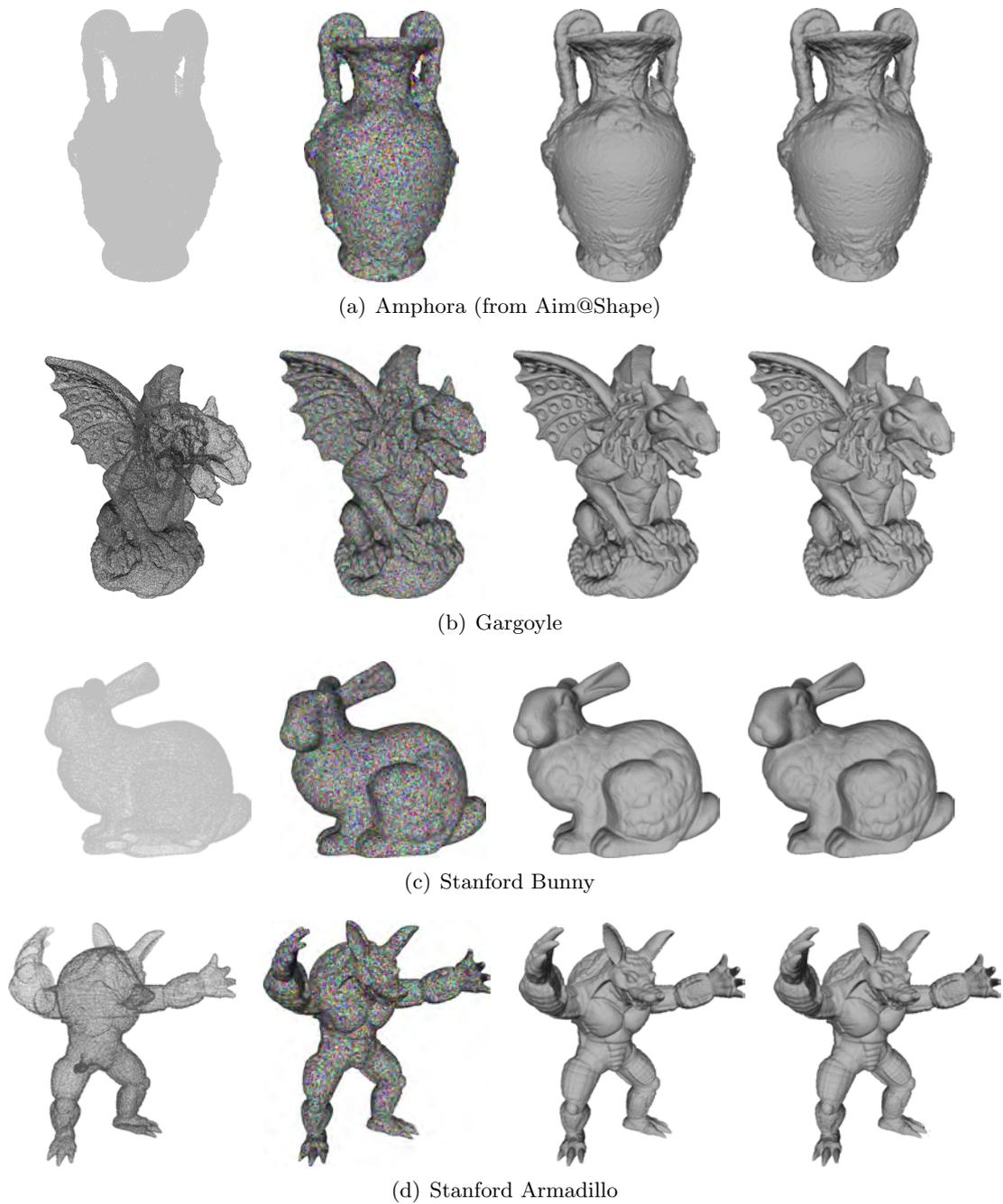
Figure 7.9: Examples of the methods' behaviour when applied to range scan datasets. From left to right, input points, generated splats, and the results of the S-T cut and Normalized cut methods. How both methods retrieve similar surfaces in all the experiments can be observed.
