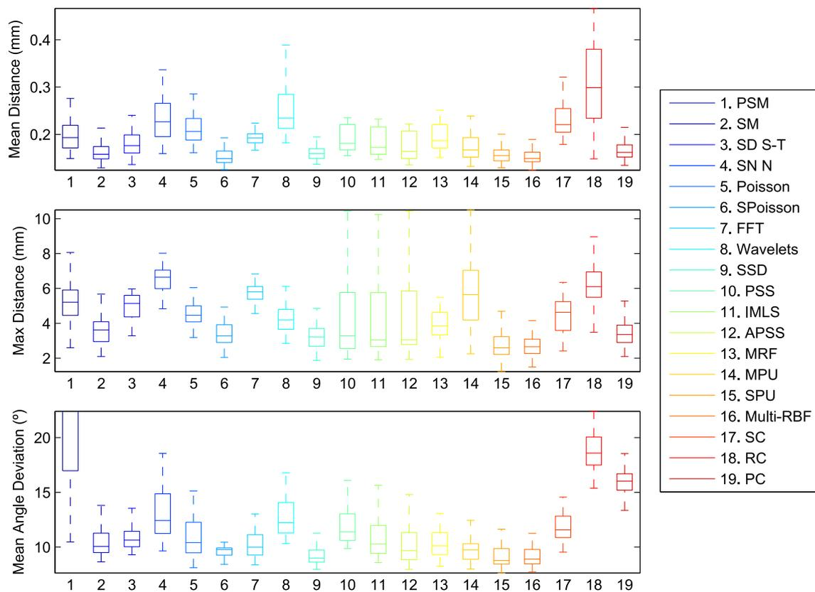
Figure 8.5: Benchmark by Berger et al.[22], results for the **Gargoyle** dataset. We show the mean and maximum (i.e., Hausdorff) distances, and the mean angle deviation for each method when applied to 48 synthetic scans generated using various scanning parameters.
