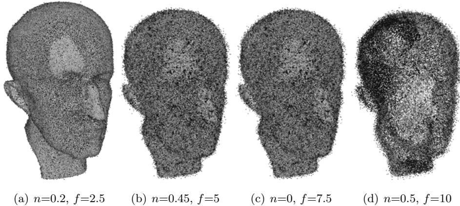
Figure 8.8: Four sample point sets of the Max Planck shape, from a total of 44. Under each figure, we detail the level of noise magnitude ( $n$ ) and laser's field-of-view size ( $f$ ). Normals are used to apply shadow casting to the model.
