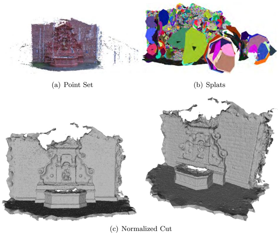
Figure 7.14: Fountain dataset, obtained using plane sweeping, obviously containing a larger number of aberrations than in the PMVS case visible in Figure 6.14 (page 198). The surface retrieved using our Normalized cut method is shown in (b).
