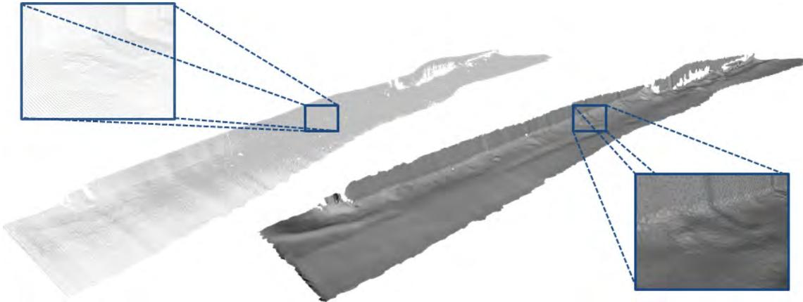
Figure 5.13: Multibeam sonar reconstruction (413,873 points). Instead of the standard downward-looking configuration, the transponder was installed laterally, giving rise to a full 3D dataset.
