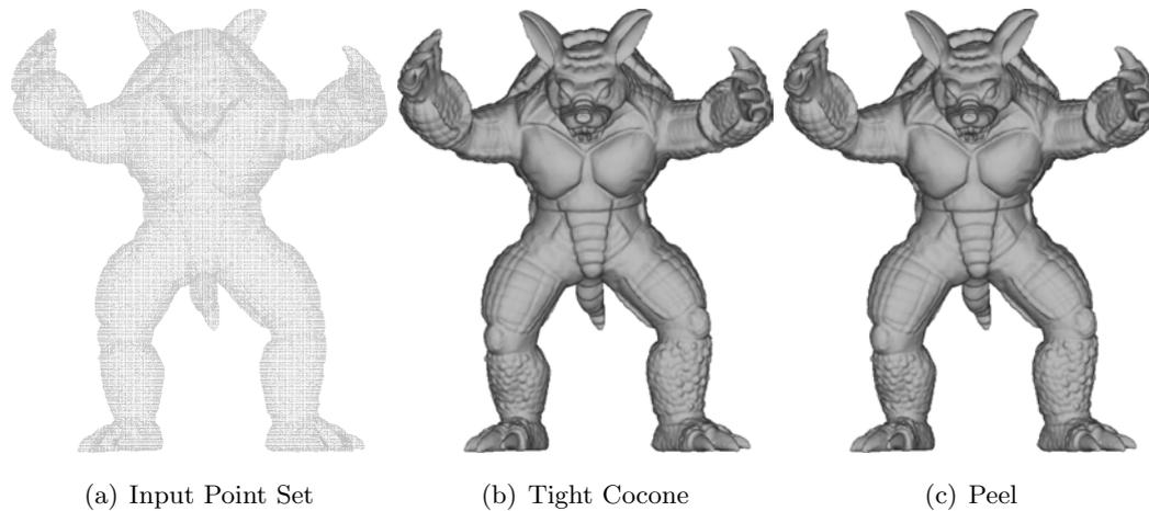
Figure 4.9: Examples of the behaviour of the Tight Cocone and Peel algorithms when applied to the Armadillo dataset.
