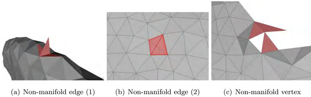
Figure 5.4: Non-manifold structures, highlighted in red.
