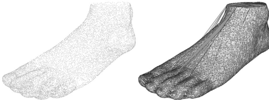
Figure 4.4: Gabriel triangles (right) of a given point set (left). Note how the majority are part of the surface of the object.
