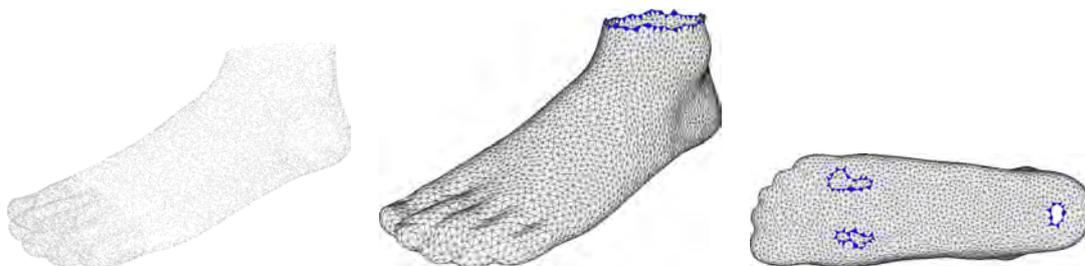
Figure 6.9: Foot dataset (10,010 points). The first column shows the point set. The second and third columns show two views of the model with boundary triangles depicted in blue.
