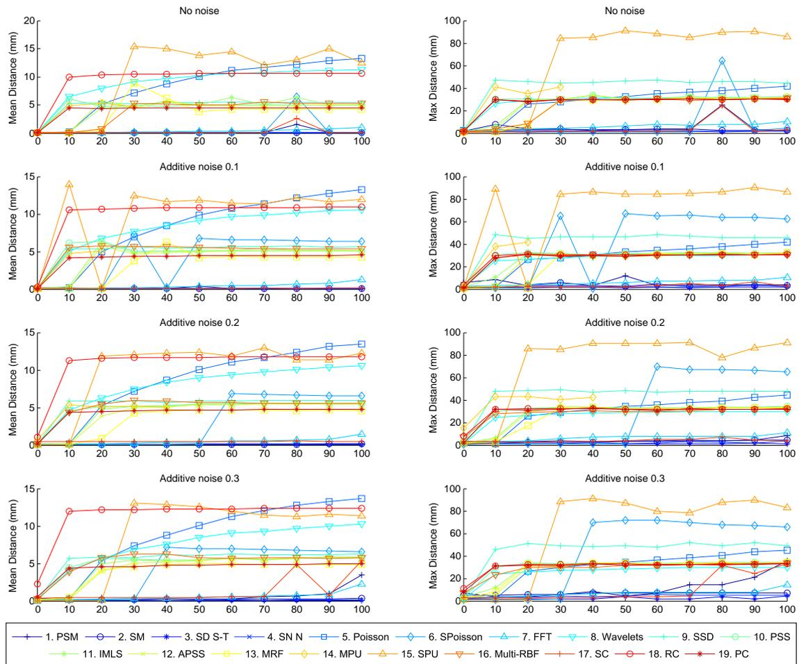
Figure 8.13: Results for the outliers test. Line charts on the left show the mean distance results, and on the right, the maximum (i.e., Hausdorff) distance. Big jumps in the mean/maximum measures clearly point out the break down point of the methods for a given level of noise and outliers.
