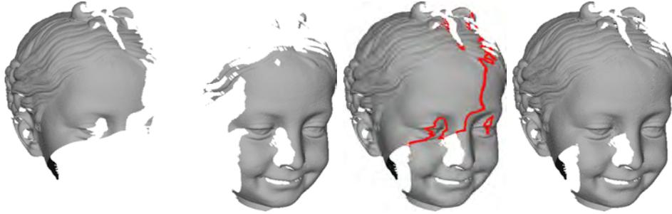
Figure 4.7: Zippered meshes, using the implementation of the variant proposed by Marras et al. [154]. The first pair of figures shows two separated range scans. The next pair of images shows the merged model, the first denoting in red the border where the zippering took place.
