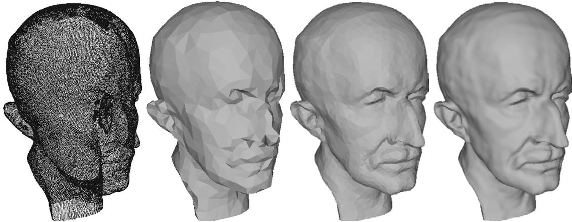
Figure 4.20: Spherical Cover method [168] applied on the Max Planck bust dataset (leftmost figure). The value of the parameter guiding the approximation quality ( $T_q$  in the original article) is increased from left to right, leading to an increasing level of complexity for the resulting surface mesh.
