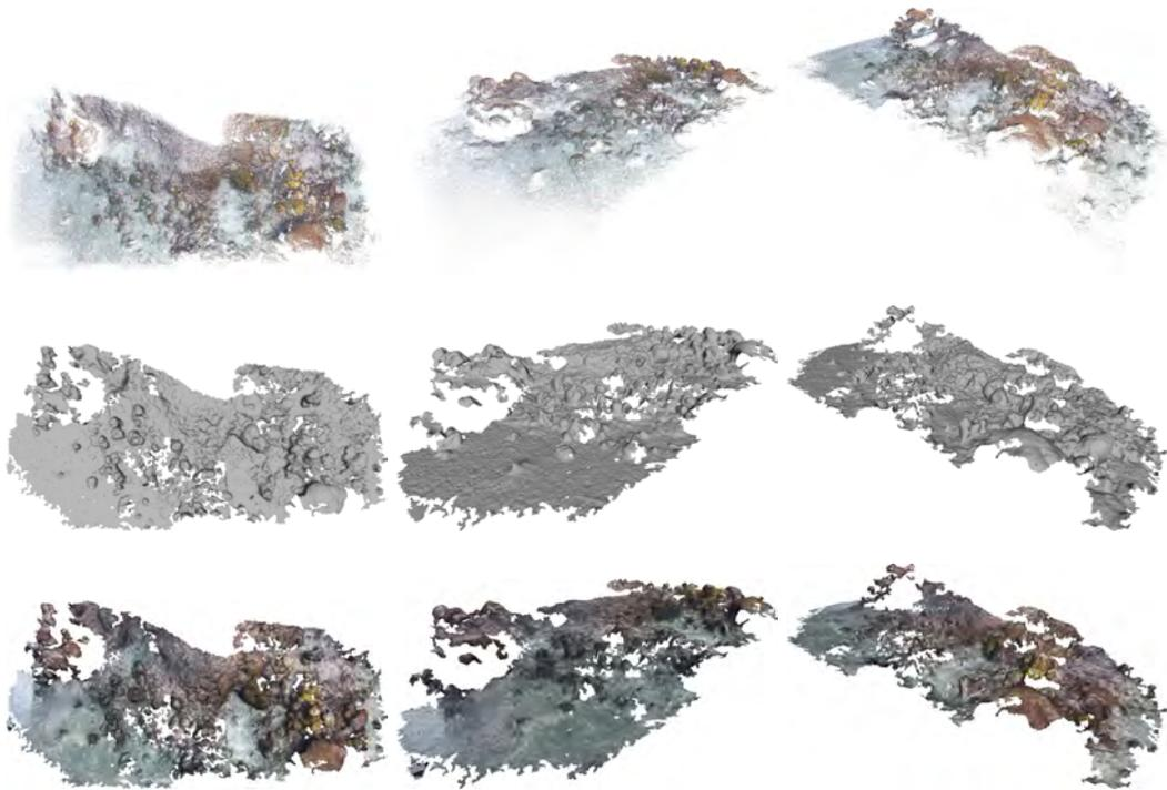
Figure 5.15: Coral Reef dataset reconstruction. From first to last row: point set (1,656,413 points), meshed surface, and textured surface.
