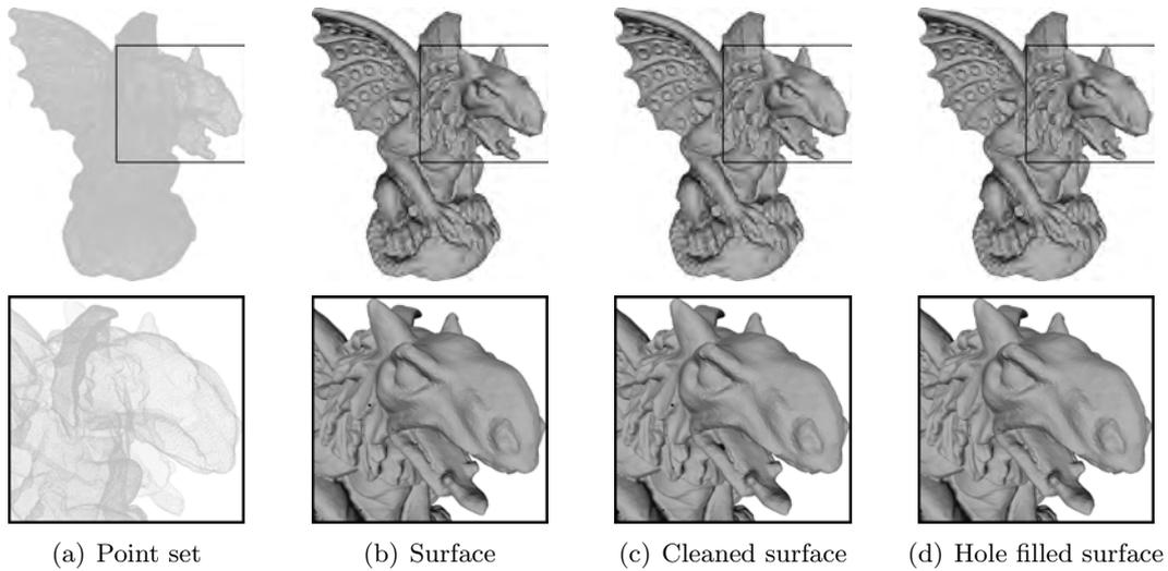
Figure 5.9: The application of our method to the Gargoyle point set (863,210 points) shown in (a) raises the surface in (b), where holes are directly visible as black spots. After the non-manifoldness cleaning step in (c), even more holes appear. By using the hole filling procedure, these small imperfections are corrected, as can be observed in (d).
