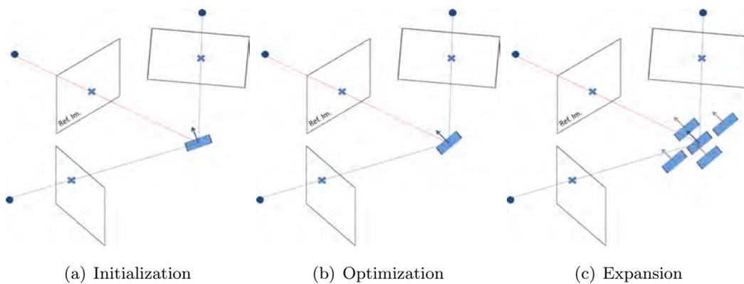
Figure 2.11: Greedy dense reconstruction process. At first (a), the initialization starts by triangulating the feature points. Then (b), a 3D patch position and orientation is optimized for photoconsistency across images. Finally (c), new patches are generated near the initial point on the tangent plane defined by the patch. New points/patches are optimized again and steps (b) and (c) are repeated iteratively, in this way, growing the points which form the reconstruction.
