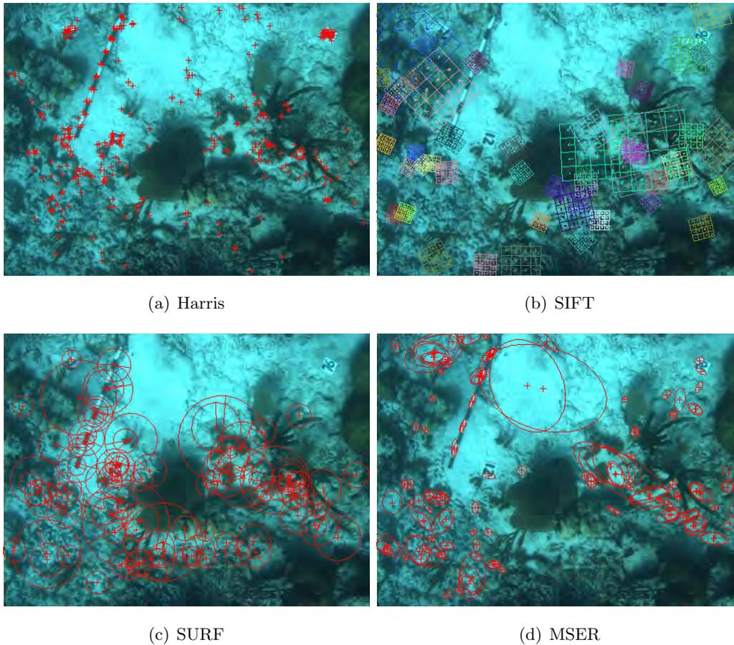
Figure 2.4: Examples of feature detection algorithms applied to an underwater image. The methods tested are those commented on the text: (a) Harris, (b) SIFT, (c) SURF, and (d) MSER. The number of features has been deliberately reduced to promote illustration clarity.
