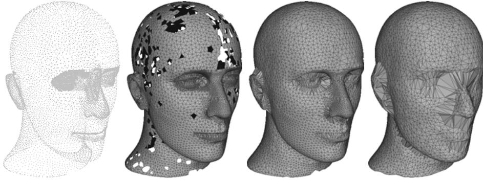
Figure 4.5: Behaviour of the Ball-Pivoting algorithm [23] for a changing value in the  $\rho$  parameter. The left-hand figure shows the input point cloud, and the value of  $\rho$  is increased starting from the second figure, from left to right. Note that, as was the case for the  $\alpha$ -shapes, an optimal  $\rho$  value may not exist for a given dataset.
