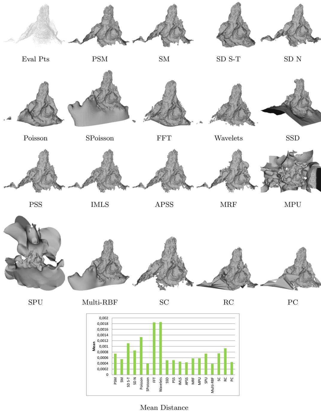
Figure 8.3: Real data tests, results for the Tour Eiffel dataset. Values with respect to the BBD.
