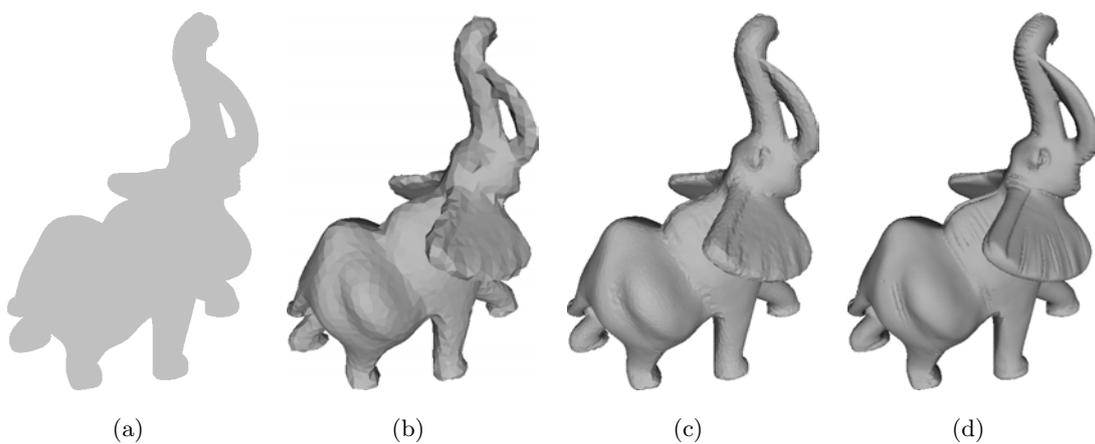
Figure 5.10: The Elephant dataset (1,537,283 points), shown in (a), is used as input for our method to create multiple surfaces, shown from (b) to (d), at increasing resolution.
