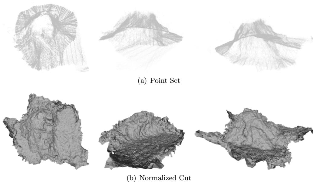
Figure 7.11: Underwater Mound retrieved with a multibeam survey (a), and the reconstructed surface using Normalized cuts (b).
