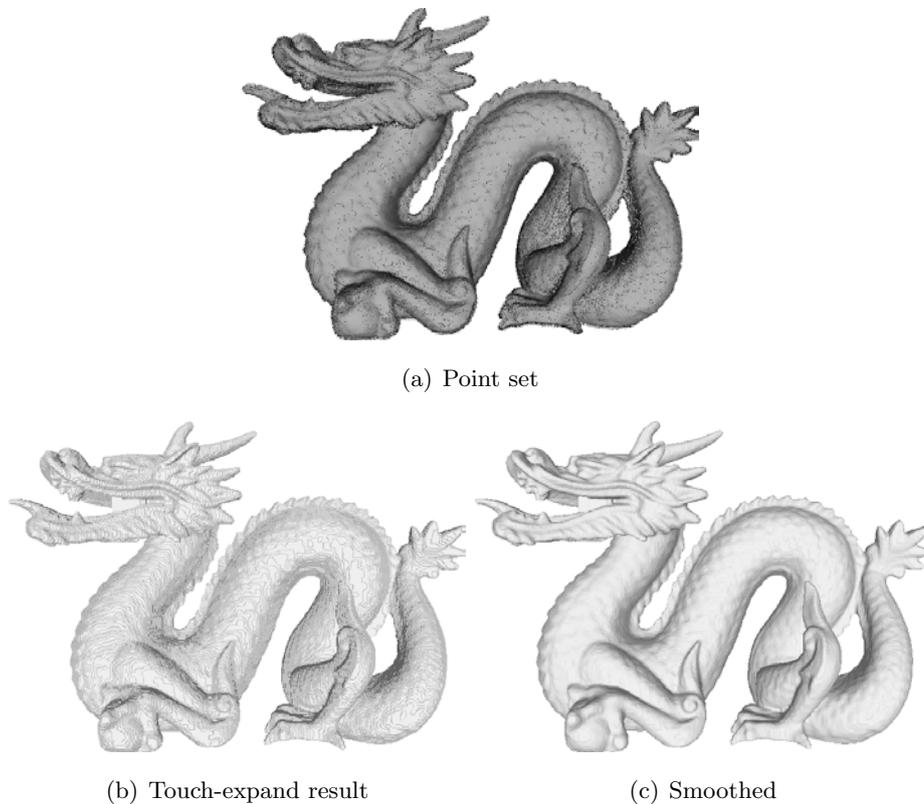
Figure 4.16: Touch-expand algorithm [135] applied to the Stanford Dragon dataset (figure in the first row). Note how the resulting surface presents a staircase effect, produced by the method being a binarization inside a regular voxel grid (lower left figure). As suggested in the original reference, some smoothing is needed to alleviate this aberration (lower right figure).
