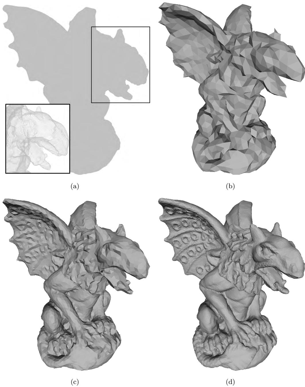
Figure 6.10: Different resolutions and quality of the final surface can be achieved by changing the parameters of the surface meshing without changing the splats approximation. (a) presents the point set (863,210 points), while (b), (c) and (d) show incremental levels of resolution with respect to the size of the triangles and the approximation bounds.
