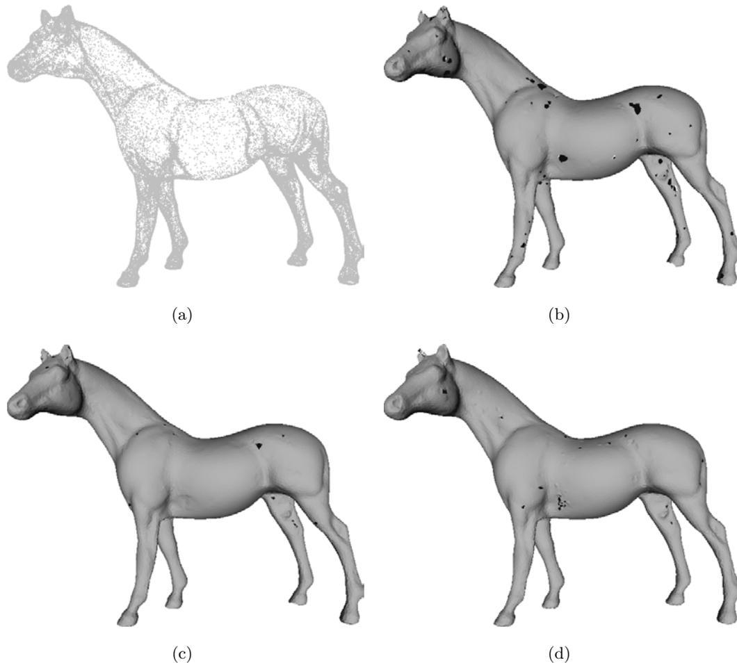
Figure 6.11: Horse dataset, (a) example of a very sparsely sampled point set, 100,000 points. We then show the results of our method for different values of the  $k$  parameter. (b) corresponds to  $k = 25$ , (c) to  $k = 50$  and (d) to  $k = 100$ .
