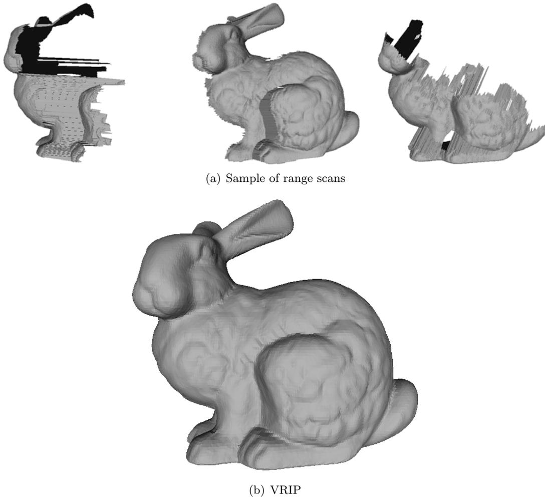
Figure 4.18: Sample of the VRIP [60]. The top row shows a sample of 3 range scans (from a total of 10) forming the Stanford Bunny dataset, while the second row shows the result of the algorithm.
