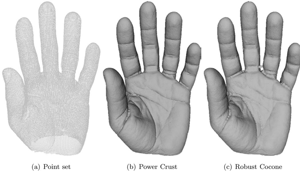
Figure 4.8: Sample of both methods presented inside the In/Out Separation category. Note how there are small differences between the Power Crust and Robust Cocone results (loss of small details and a bridge between fingers for Robust Cocone).
