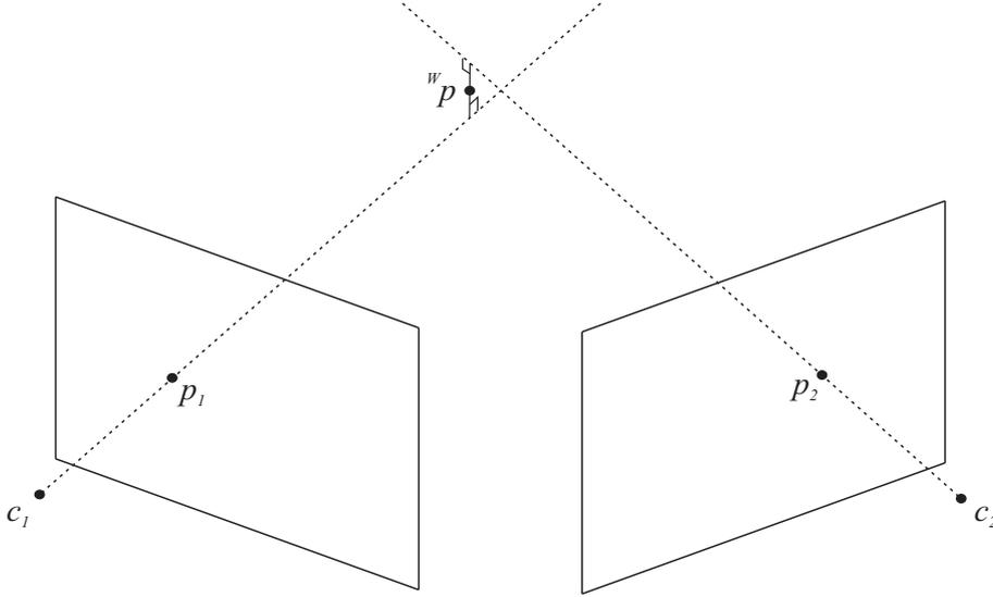
Figure 2.7: Stereo triangulation procedure. In this case, since the two lines-of-sight do not intersect, the final reconstructed point  ${}^W p$  is computed as the midpoint of the smallest segment joining the rays (i.e., the one orthogonal to both).
