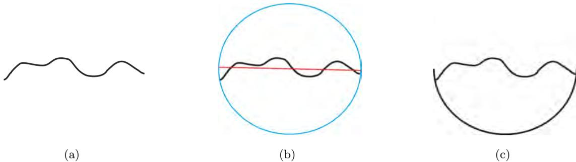
Figure 7.4: 2D Schematic of the extension for the S-T cut method to handle bounded surfaces. The curve in (a) is not closed, and consequently it does not define an inside or an outside. We compute a global frame using PCA, and use it to chop the surface into two spherical caps, as depicted in (b). One of the spherical caps is used to *virtually close* the surface as presented in (c), so that we can disambiguate the inside/outside computation.
