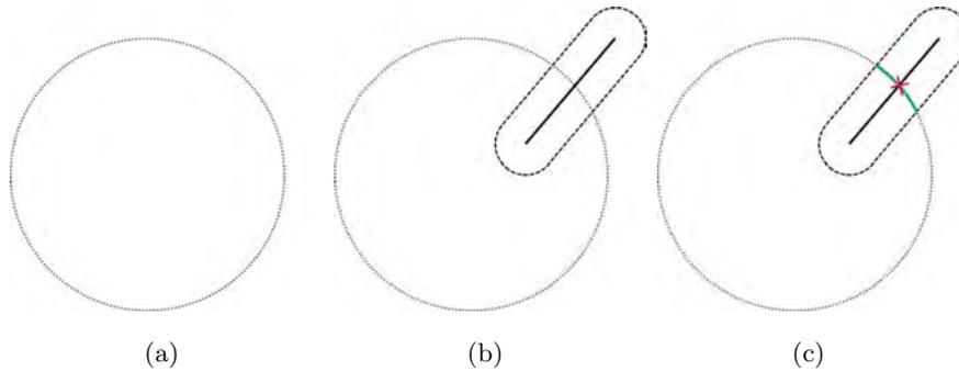
Figure 5.1: Schematic overview of the proposed on-line segment intersection query computation. (a) presents the input points, and (b) the query segment and its capsule neighborhood. As depicted in (c), a local surface is fitted to the points inside the capsule neighborhood and the intersection is computed.
