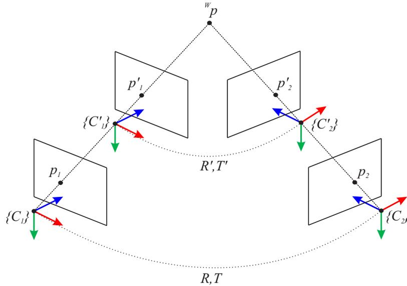
Figure 2.8: Scale ambiguity in SFM approaches. The same 3D point can be generated indistinctly by either  $C_1$ - $C_2$  or  $C'_1$ - $C'_2$ , where the two stereo systems differ by a scale factor.
