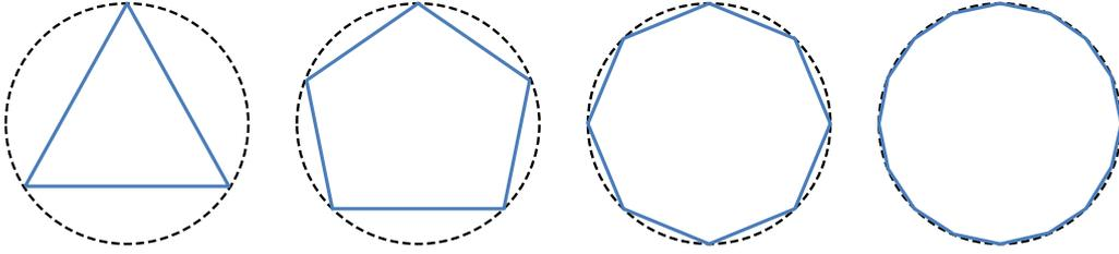
Figure 3.2: Piecewise-explicit representations of a circle, with increasing resolution from left to right.
