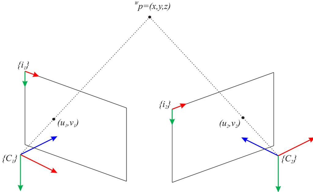
Figure 2.3: Stereo setup: two (or more) views disambiguate the 3D position of the point along the line-of-sight emanating from the camera’s optical center and passing through the 2D point projection.
