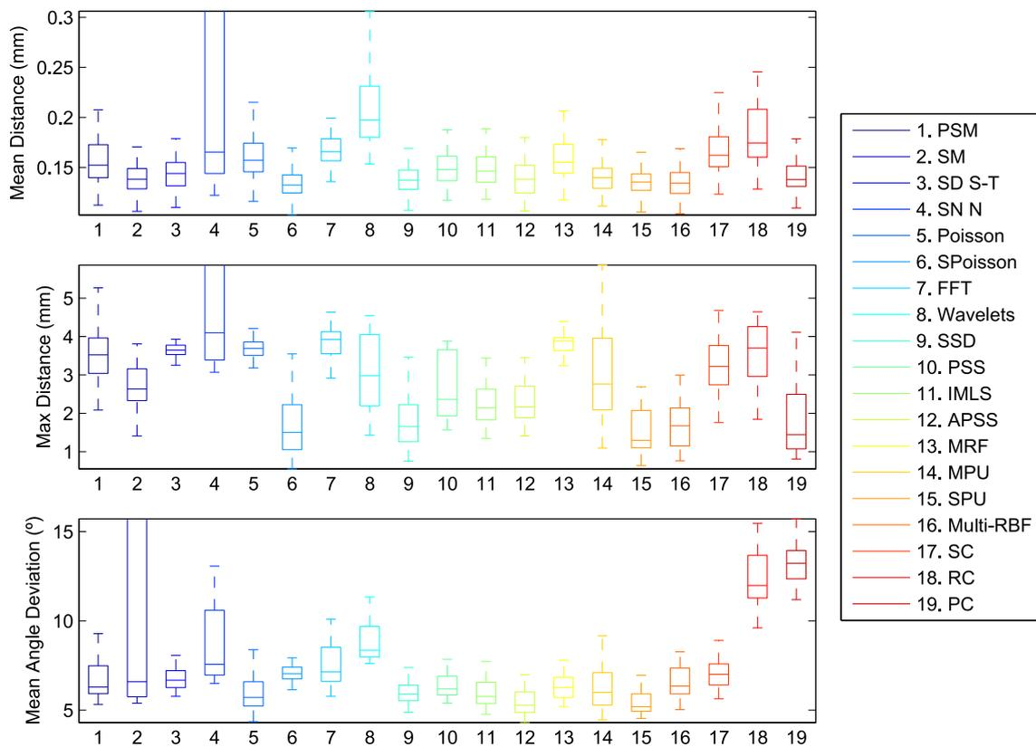
Figure 8.7: Benchmark by Berger et al.[22], results for the **Quasimoto** dataset. We show the mean and maximum (i.e., Hausdorff) distances, and the mean angle deviation for each method when applied to 48 synthetic scans generated using various scanning parameters.
