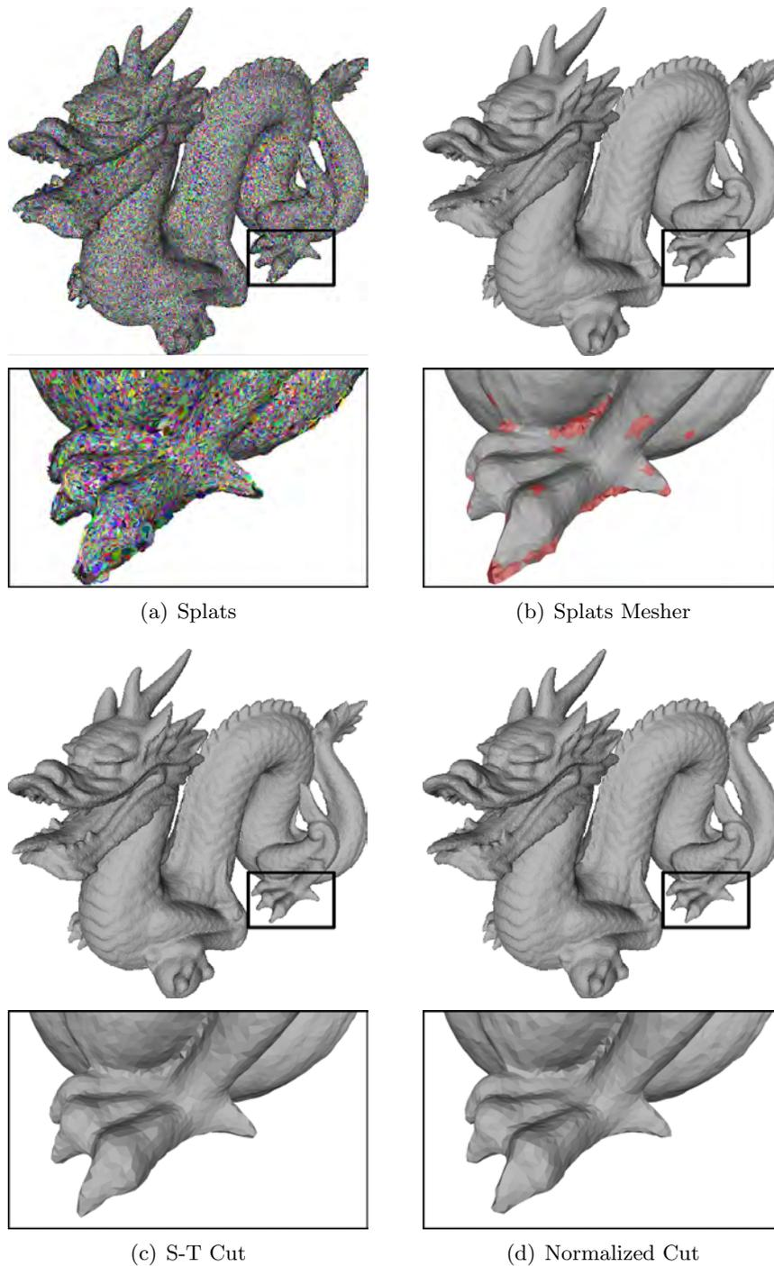
Figure 7.8: Using the same splat representation shown in (a), we present a comparison of the splats mesher (b) and the two methods proposed in this chapter – (b) for S-T cut, and (c) for Normalized cut. Note that in the lower part of (b), we have emphasized the triangles containing some non-manifold edges in red.
