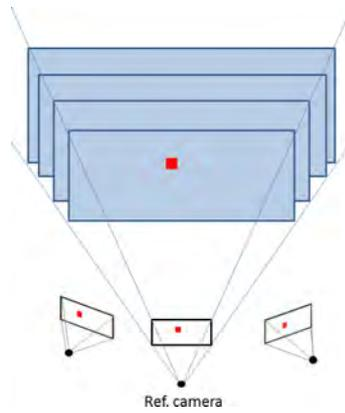
Figure 2.10: Depth map construction. Several candidate depths (blue rectangles) are tested, while each possible patch (red square) is given a similarity score based on its projection onto neighboring images.
