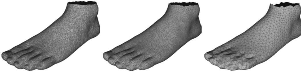
Figure 3.8: Sample of the behaviour of a surface mesher [30]. The original (irregular) mesh is on the left, and center/right show the results for two different parameterizations of the meshing algorithm, providing different resolutions for the input mesh. Note how the remeshed surfaces promote triangles closer to regular.
