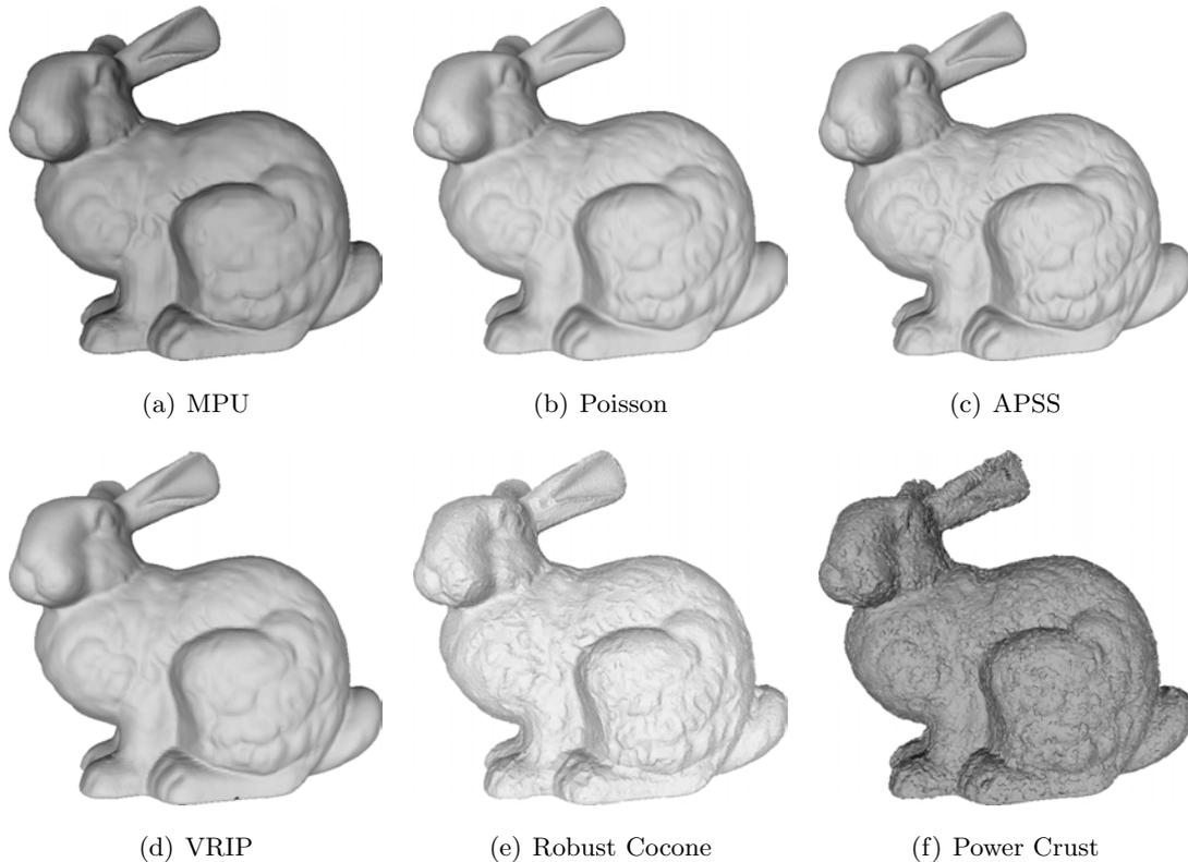
Figure 6.12: Reconstructions for the Stanford Bunny dataset using some of the methods from the state of the art. (a) Multi-level Partition of Unity [165], (b) Poisson [118], (c) Algebraic Point Set Surfaces [97], (d) Volumetric Range Image Processor [60], (e) Robust Cocone [65] and (f) Power Crust [13].
