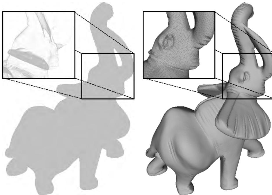
Figure 6.4: Elephant dataset: 1,537,283 points, both noise and outlier free. Left: input pointset with closeup. Right: reconstructed surface with closeup.
