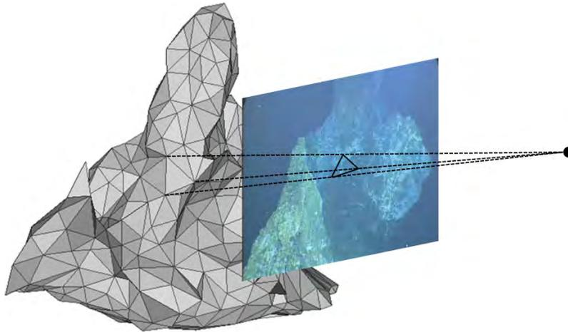
Figure 2.12: Texture mapping process, the texture filling a triangle in the 3D model is extracted from the original images.
