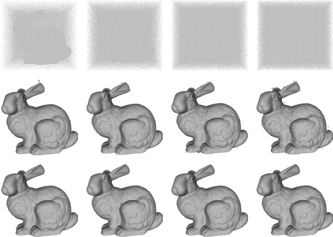
Figure 6.7: Robustness to outliers. The first row shows the outlier-ridden point sets. The percentages of outliers added, with respect to the number of points on the original point set, are 50%, 100%, 150% and 200%, added inside its bounding box (enlarged by 5%). The last 2 rows show the results when applying our method to its vertically corresponding point set. The second row uses  $\delta_r = 0.005BBD$ , while the third row uses a more restrictive  $\delta_r = 0.0025BBD$ .
