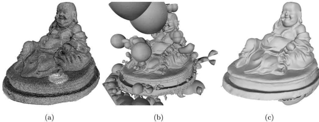
Figure 4.14: Comparison between the original MPU [165] and the smoothed version [161]. Note how the heavy noise of the input dataset (a), in both position and normal, leads to a bumpy surface with artificial components on MPU (b). Smoothing out the local contributions results in a continuous representation of the surface (c).
