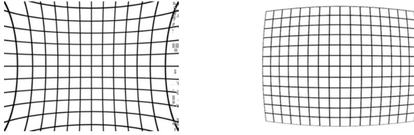
Figure 2.2: Common image distortion types introduced by optics on real-world cameras. On the left, pincushion distortion, on the right, barrel distortion. Note how the straight edges of a regular grid in the real world are imaged under both types of distortion.
