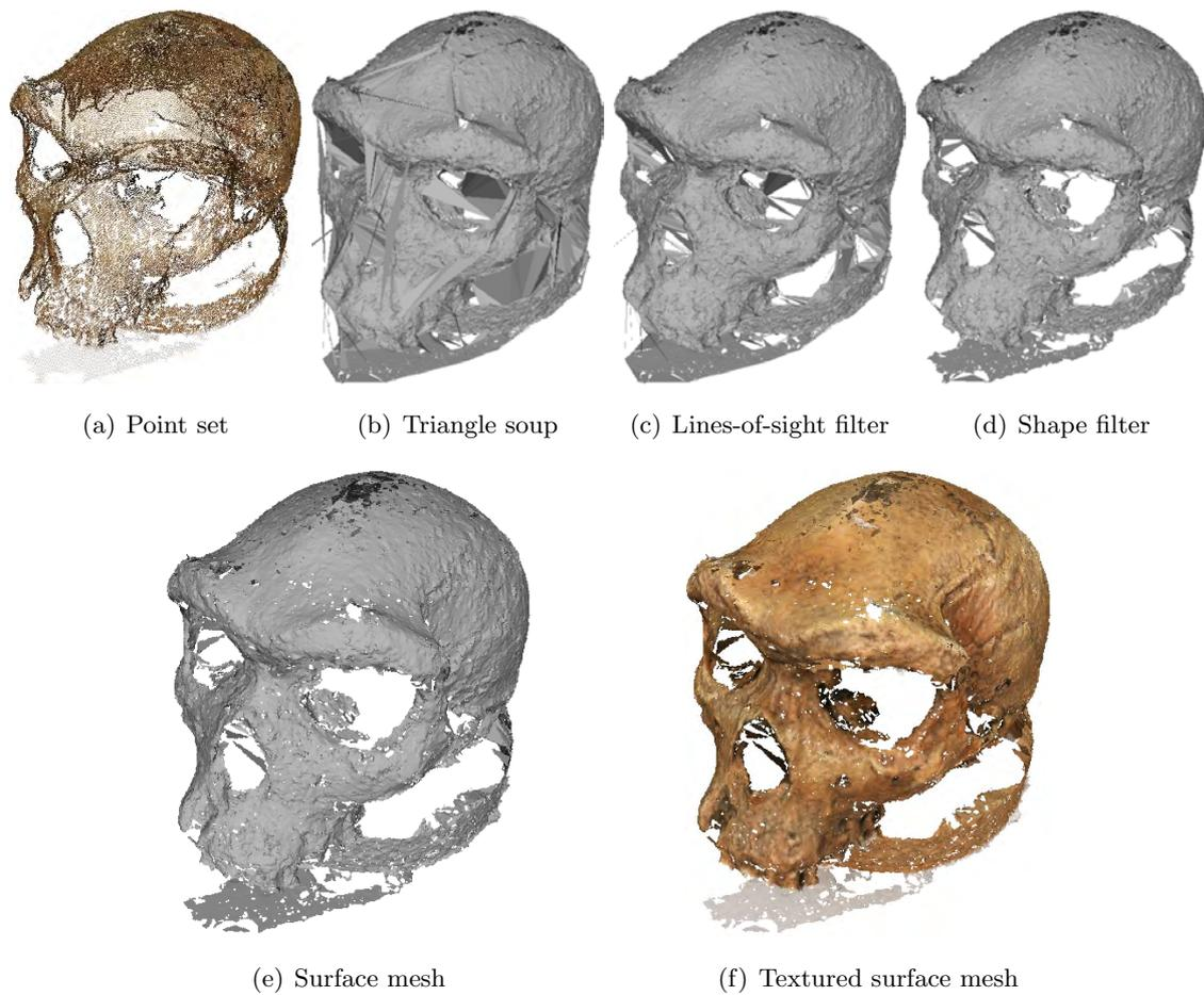
Figure 4.19: Lifted Constrained Delaunay method [180]. Figure (a) shows the point cloud. The initial triangle soup made by joining the constrained 2D triangulations in 3D is depicted in (b). This initial triangle soup is filtered using lines-of-sight (c) and shape constraints (d). This last triangle soup (d) is used to obtain the final surface through Delaunay refinement, resulting in the surface in (e) - with its textured version in (f).
