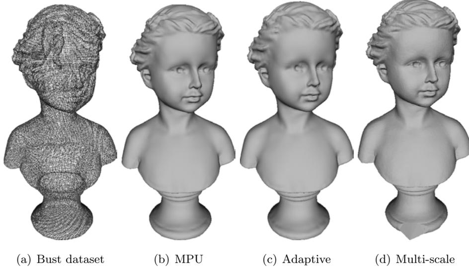
Figure 4.13: Results of the reconstruction of the Bust dataset (a) for three similar methods: MPU [165] (b) and the adaptive [167] (c) and the multi-scale [166] (d) version of MPU+RBF.
