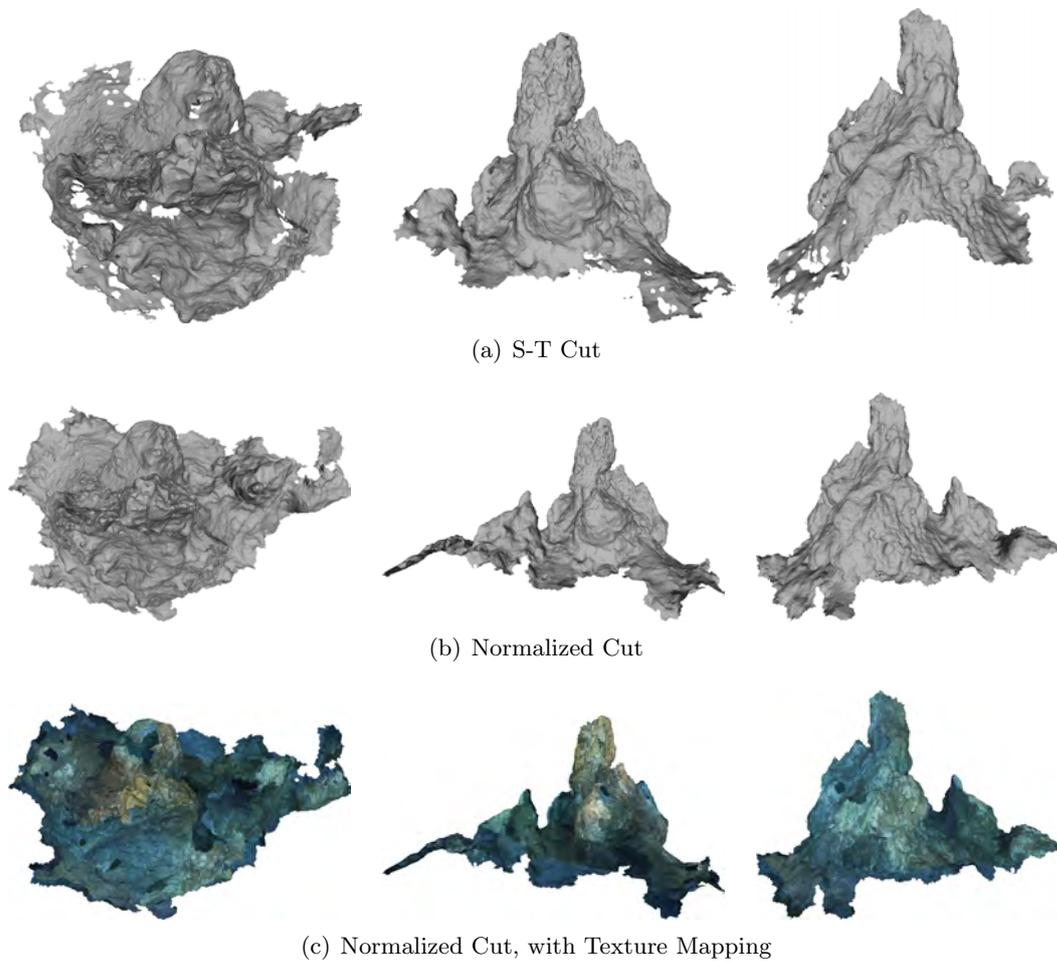
Figure 7.17: Results for the Tour Eiffel dataset. From left to right: top, front and back views of the reconstructed models. We show the results of the S-T cut (a) and the Normalized cut (b) algorithm, along with its texture mapped version (c).
