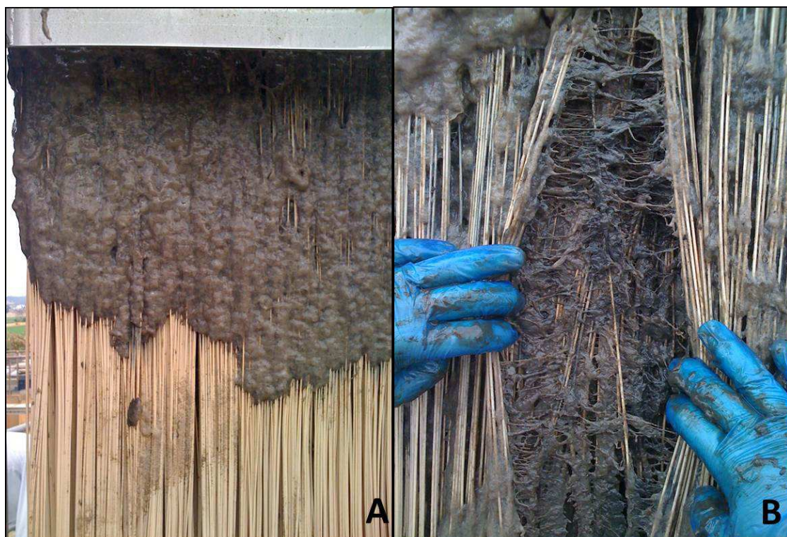
Figure 6.5. Pictures of the ragged membranes. (a) Top of the cassette (b) inside the cassette.
