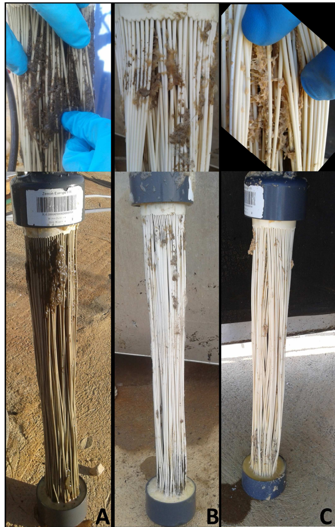
Figure 7.7. Pictures of membrane: (a) before recovery cleaning, and after recovery cleaning by NaClO (b) and by ClO 2 (c).
