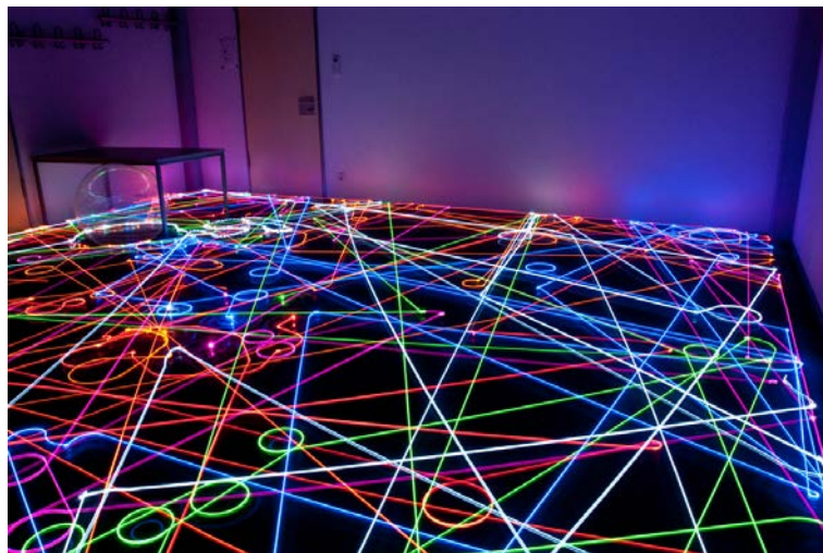
Figure 4: Long-exposure photo of the randomized coverage path traced by a team of Roomba cleaning robots using LED light sources in a dark room. Image credit: Tobias Baumgartner, Marcus Brandenburger, Tom Kamphans, Alexander Kroeller and Christiane Schmidt of the IBR Algorithm Group at Braunschweig University of Technology.
