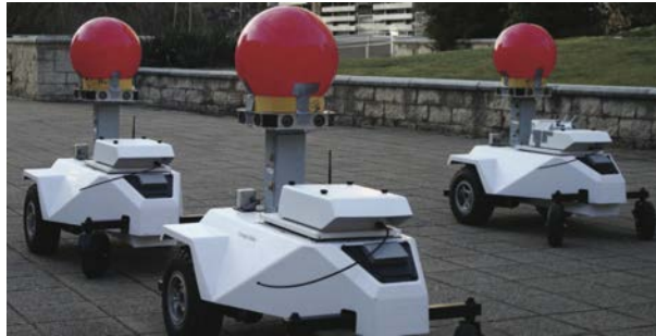
Figure 30: Team of three robots used for experimental evaluation of the leap-frog localization and coverage strategy. Image credit: Stephen Tully.
