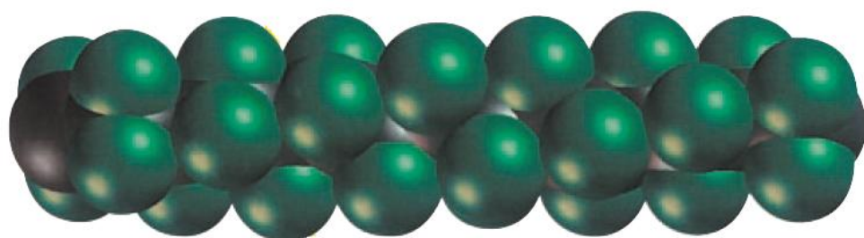
Molecular structure of conventional, unmodified PTFE
