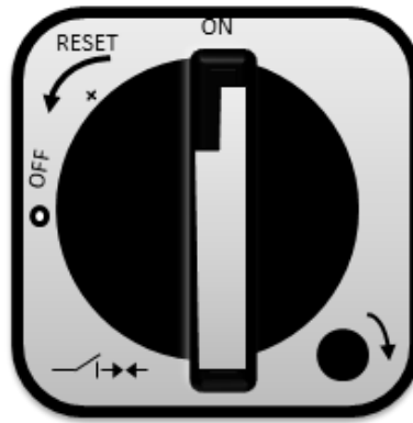
Figura A. 2. Interruptor general
