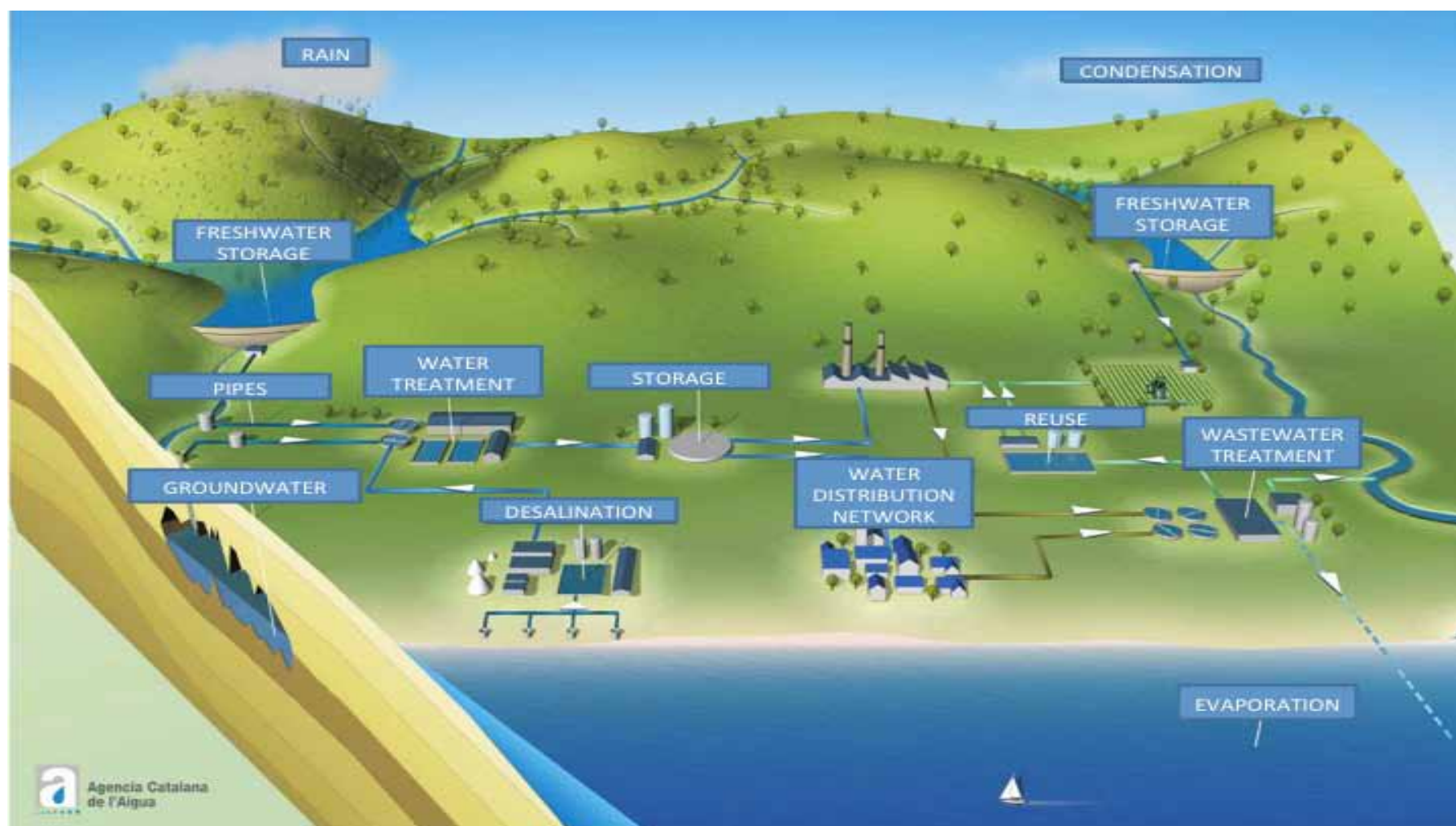
▼ Figure 1.2.1. A diagram of the urban water cycle, proposed by la the Catalan Water Agency.
