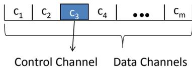
FIG. 22.1. In-band Control Channel
