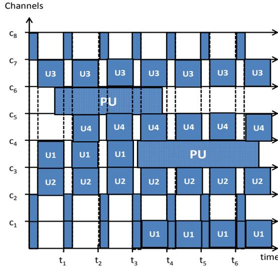
FIG. 33. Time slot utilization by both Primary Users (PU) and Cognitive Radio Users (U1, U2, U3, U4) in time
