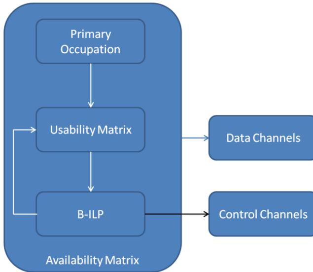
FIG. 39. Control messaging and data channel selection for the DMFOCM strategy
