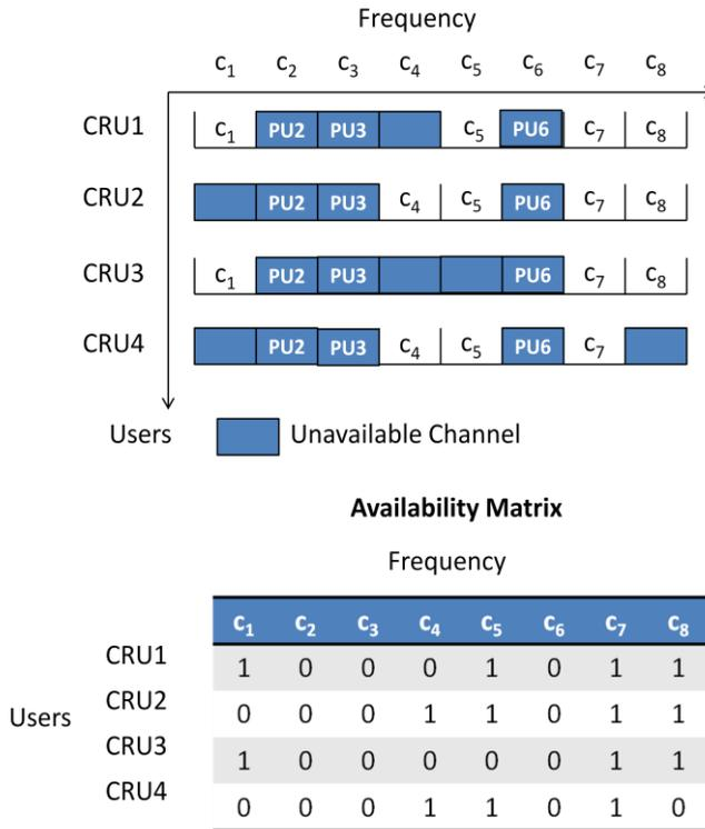
FIG. 18. Frequency Slot Utilization by both PUs And CRUs (In Time)
