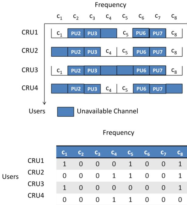
FIG. 19. Frequency Slot Utilization by both PUs And CRUs
