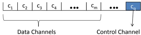
FIG. 22.2. Out-band Control Channel
