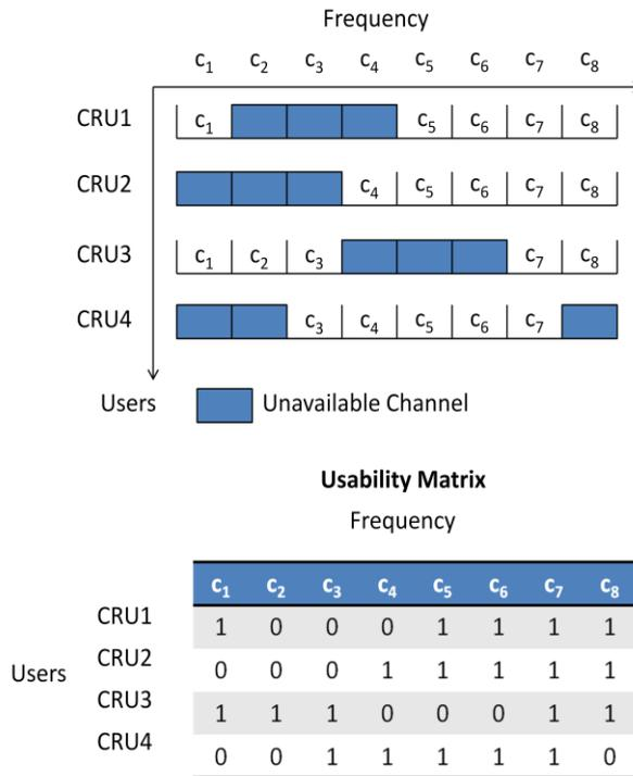
FIG. 17. Frequency Slot Utilization by CRUs
