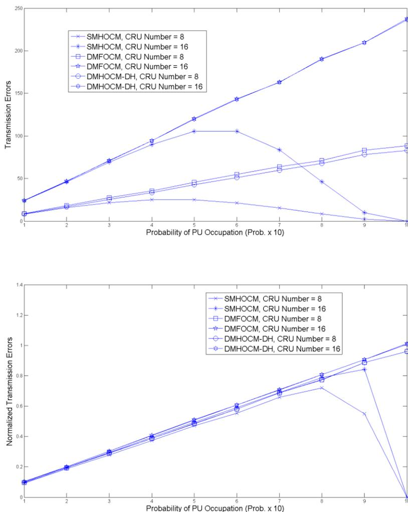
FIG. 46. Transmission errors for the SMHOCM, DMFOCM and the DMHOCM-DH strategies
