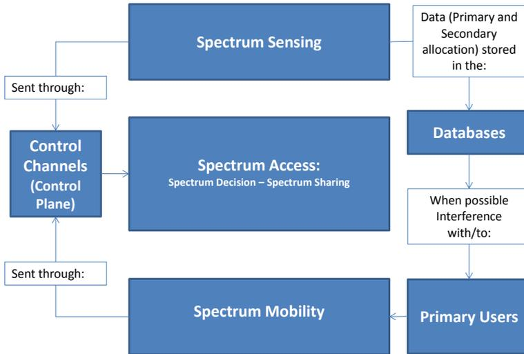
FIG. 21. Spectrum Functions and Control Plane
