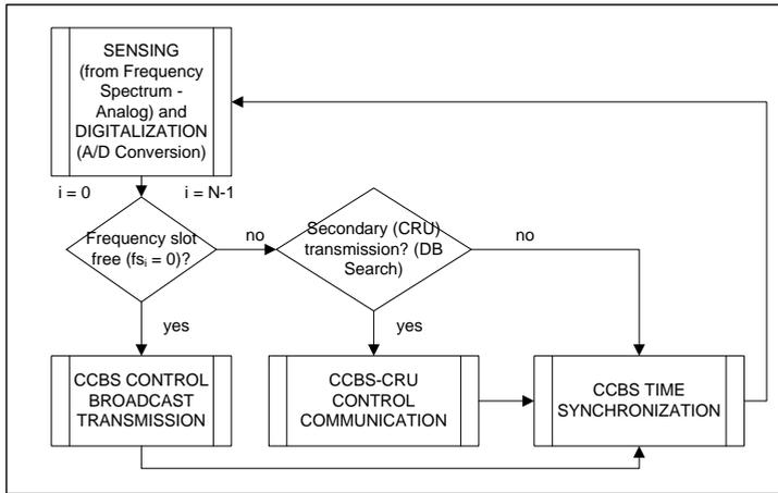
FIG. 27. CCBS Algorithm per each frequency slot  $i$  ( $f_{si}$ )
