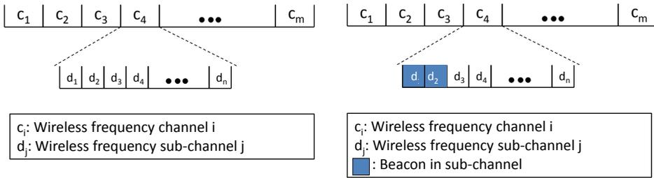
FIG. 31.1. Wireless Frequency Channel-Subchannel Division    FIG. 31.2. Beacons in Wireless frequency sub-channels
