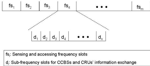
**FIG. 26.** Frequency slot and sub-frequency slot division of the spectrum
