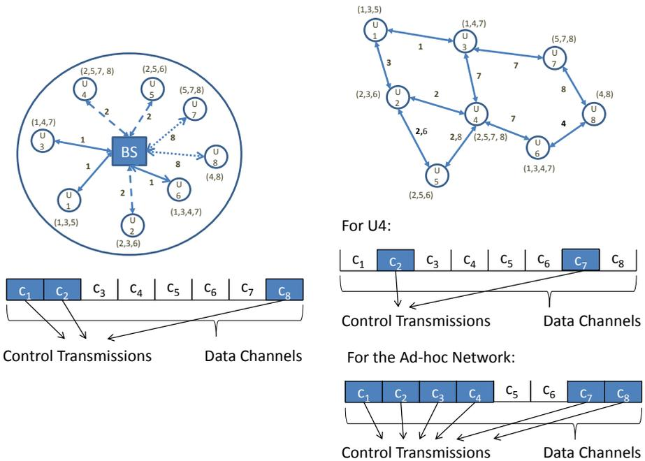
FIG. 24. Minimum Channel Problem for Centralized and Ad-hoc CRN
