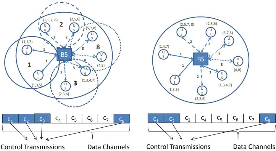
**FIG. 23.** Minimum number of channels for a clustered MCM
