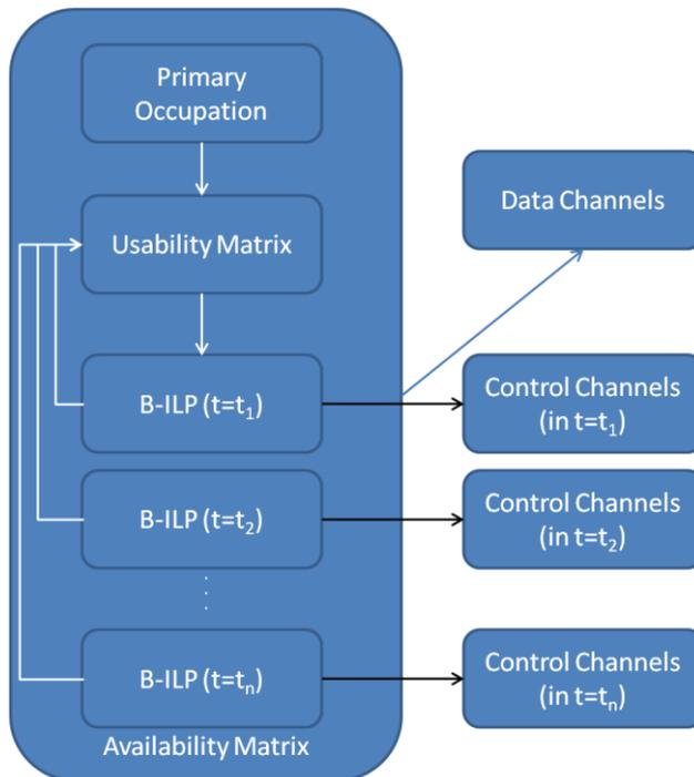
FIG. 40. Control messaging and data channel selection for the DMHOCM-DH strategy
