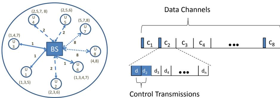
FIG. 32. Shared and multiple control messaging (Frequency-division)
