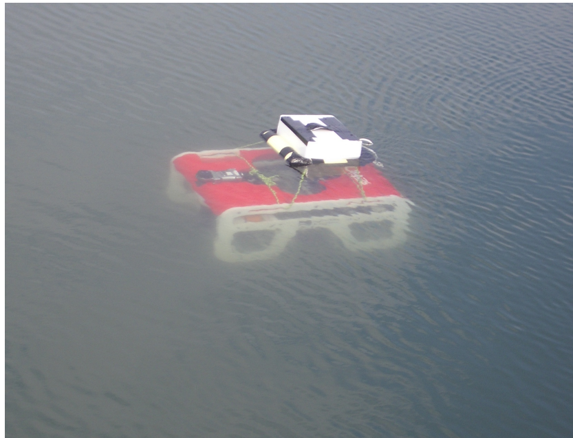
Figure 57: The Ictineu AUV with a surface buoy equipped with a DGPS.
