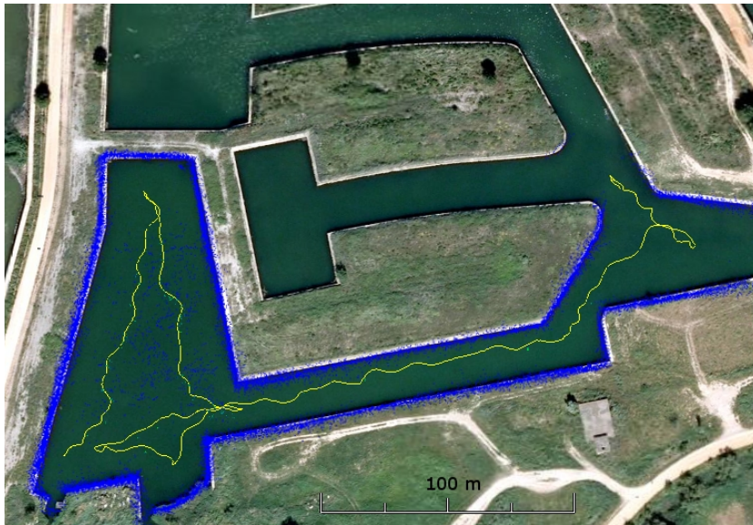
Figure 58: DGPS trajectory with range data plotted on the orthophotomap.
