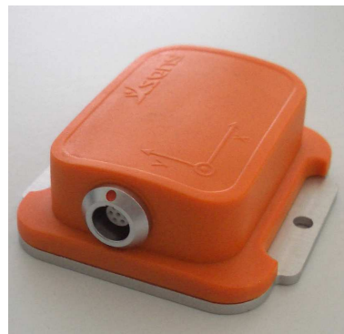
Figure 52: DVLs used in this research project.
