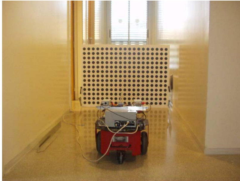
Figure 6.3: Stereo camera over a mobile robot.
