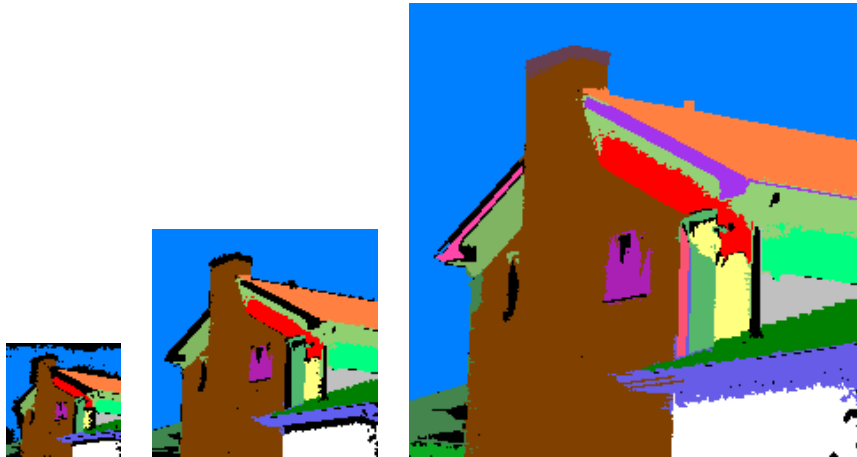
Figure 3.24: Sequence of segmentations by pyramidal structure. Coarse segmentation is successively refined at next level of the pyramid until the full resolution image.
