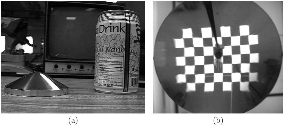
Figure 2.8: Special mirror designed for perspective projection. (a) The special mirror designed by A. Hicks. (b) Imaged obtained with the mirror of Hicks suspended above a chessboard. Courtesy of A. Hicks, Drexel University, Philadelphia.
