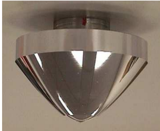
Figure 2.9: The special mirror designed by J. Gaspar. The mirror generates both vertical and horizontal constant resolution. Courtesy of J. Gaspar, Instituto de Sistemas e Robótica, Lisboa.
