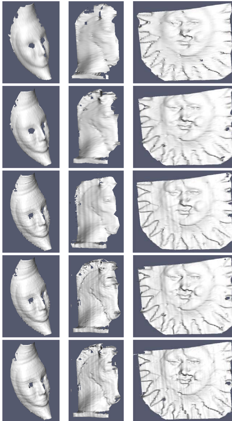
Figure 3.8: Reconstruction results of the test objects. The first row corresponds to the peak-based pattern; second row: hybrid pattern and the M + m strategy; third row: edge-based; fourth row: hybrid pattern and the E + M strategy; sixth row: hybrid pattern and E + M + m strategy.
