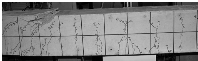
Figure B-101. Crushing of concrete for C2-212-D1-A.
