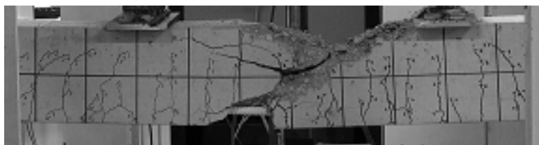
Figure B-151. Crushing of concrete for C2-316-D1-A.
