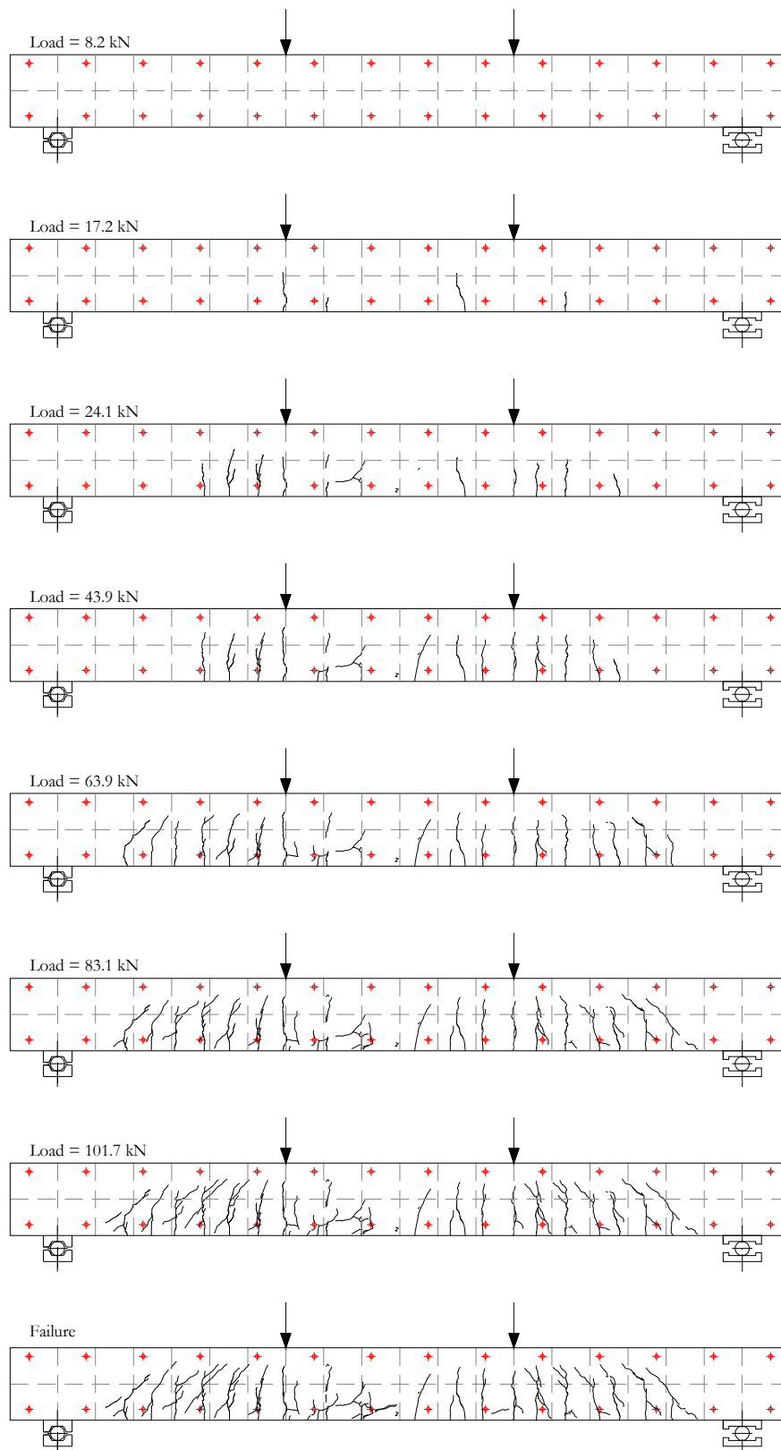
Figure B-136. Crack pattern (C2-216-D1-A).
