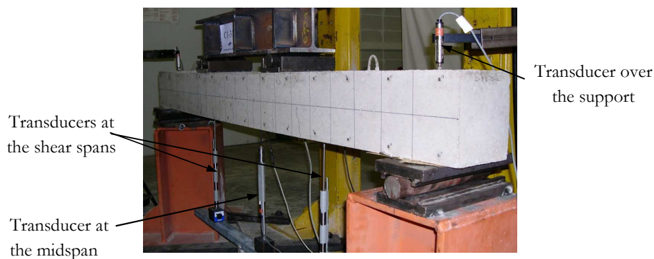
Figure 3-6. Arrangement of the vertical transducers used for the C1 and C3 tests.
