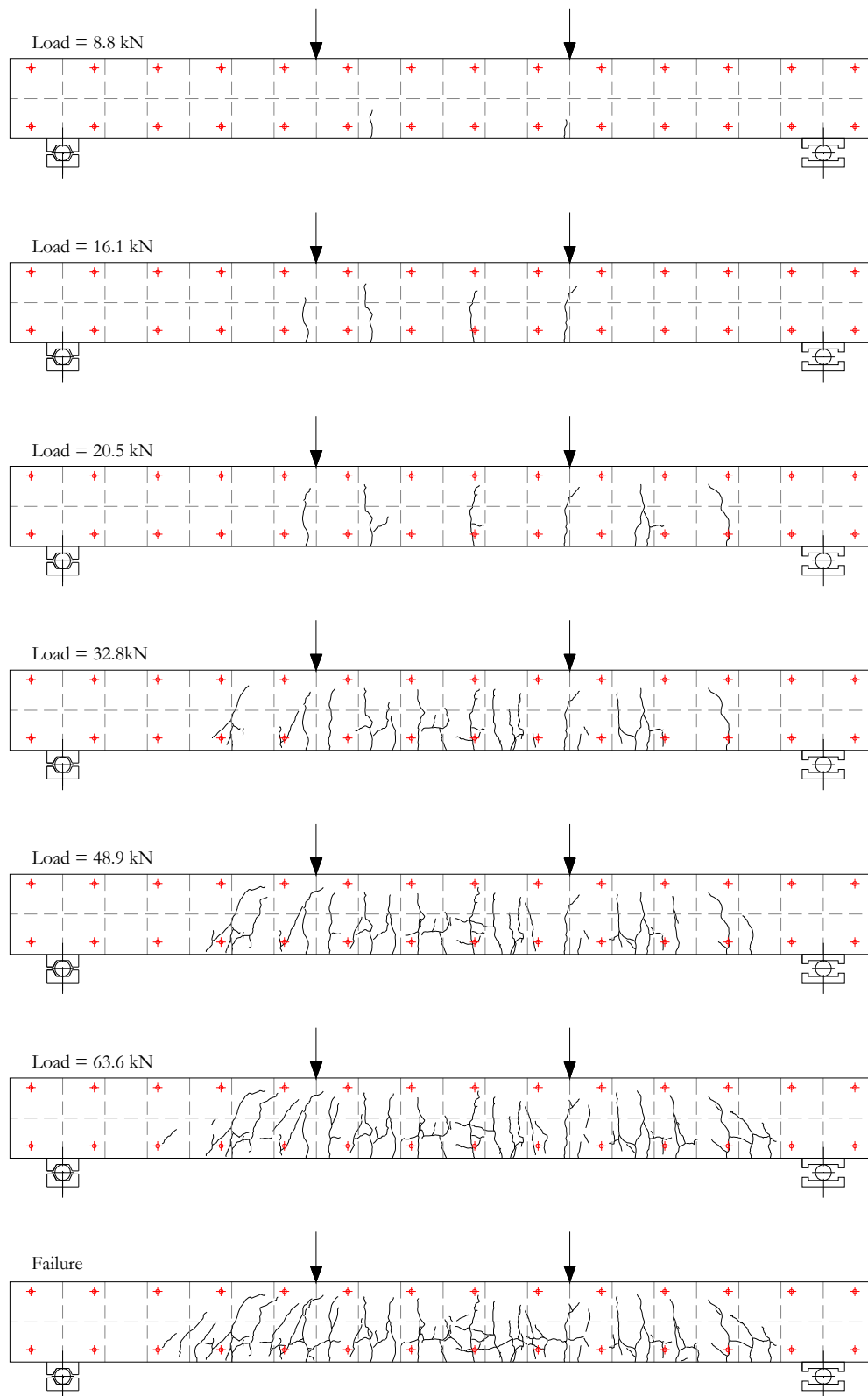
Figure B-123. Crack pattern (C2-212-D2-A).
