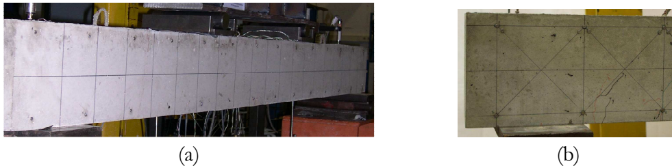
Figure 3-10. (a) Demec points for mechanical extensometer in C1 beam series (b) Detail of additional diagonal Demec points in C3 beam series.
