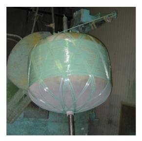
Figure 3.7: Filament winding tanks and its production technique.
