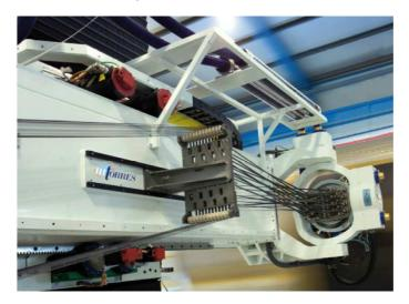
Figure 3.8: Mtorres Fibre placement machine.
