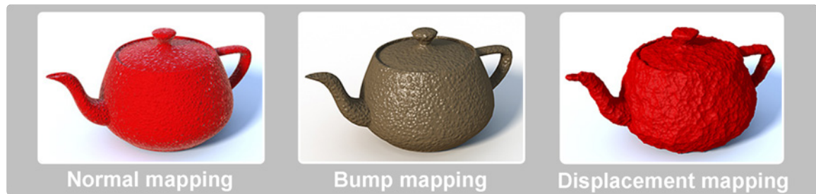
Figure 2.14: Comparison between detail mapping techniques (bump mapping, normal mapping and displacement mapping) applied on the Teapot model.
