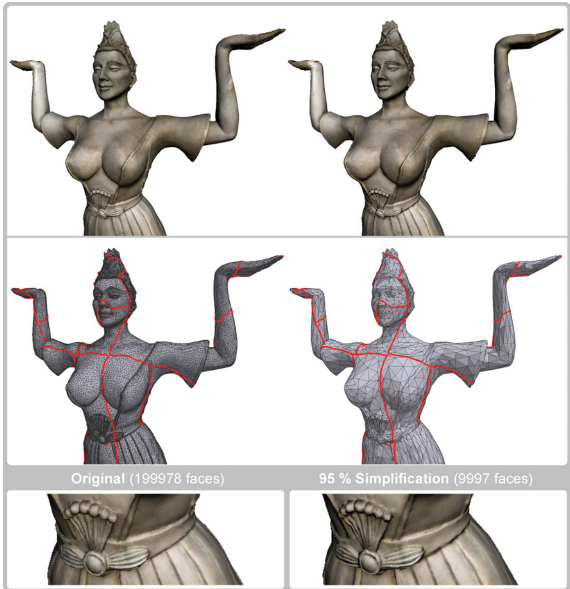
Figure 3.14: Imperia model simplified by our approach with texture and normal maps. Observe that, in both global and close-up views, the visual appearance is preserved from the original one to the simplified one. Chart boundaries (in red) have been simplified without producing artefacts.
