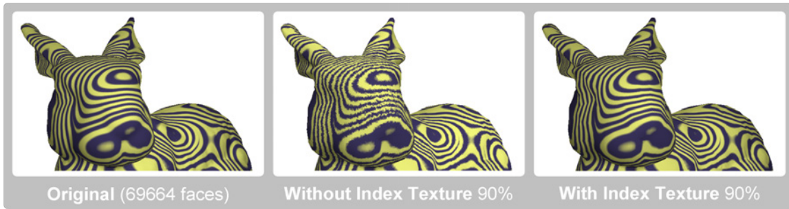
Figure 3.7: Blurring artefacts disappear when using an index texture during the simplification process.
