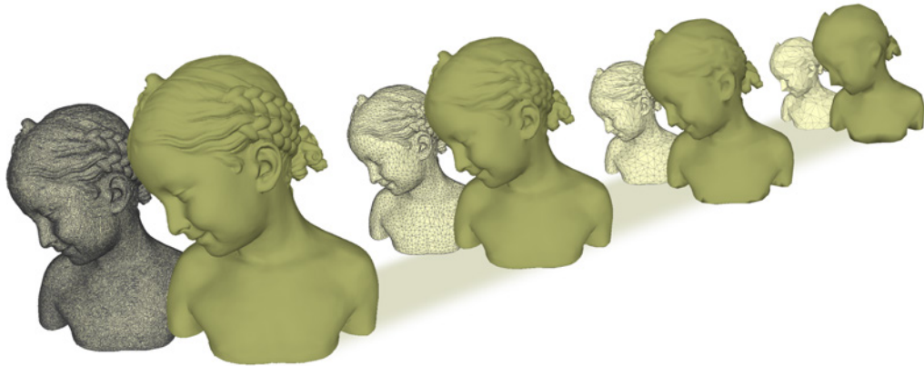
Figure 2.19: Levels of detail (LODs) of the Bimba model used to reduce the rendering cost of small, distant, or unimportant geometry.
