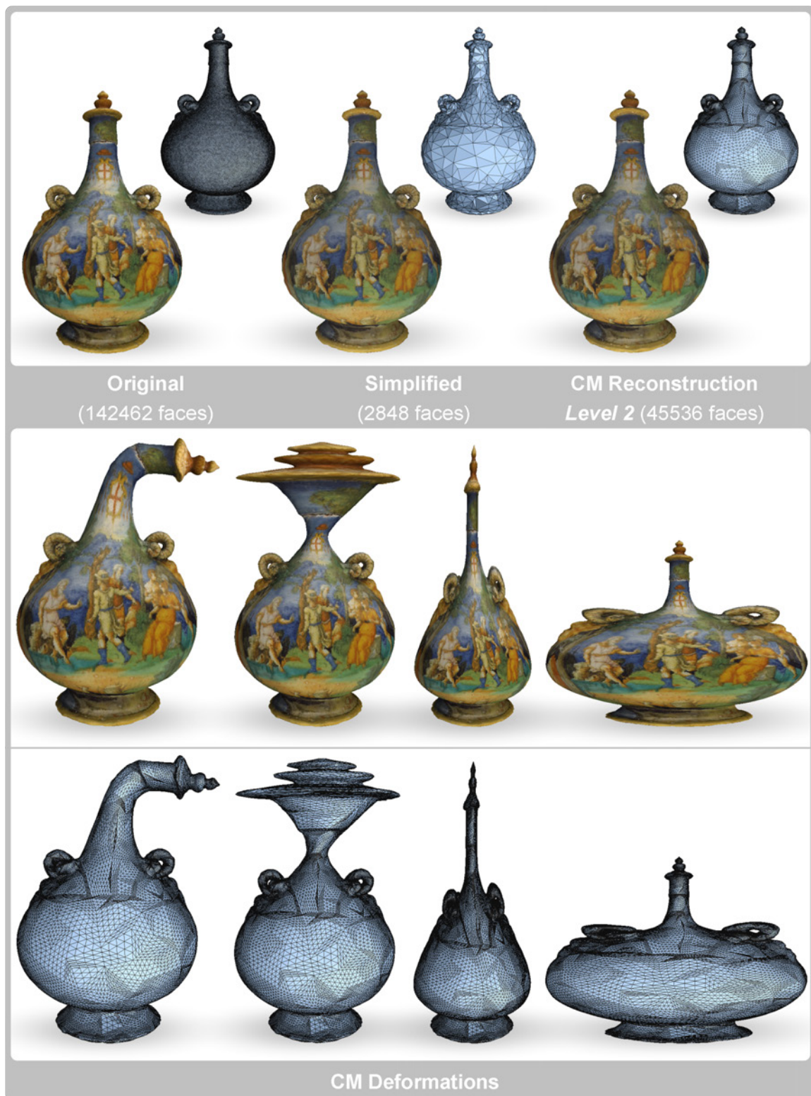
Figure 6.1: Set of deformation results from a CM of the Vase model reconstructed at level 2.
