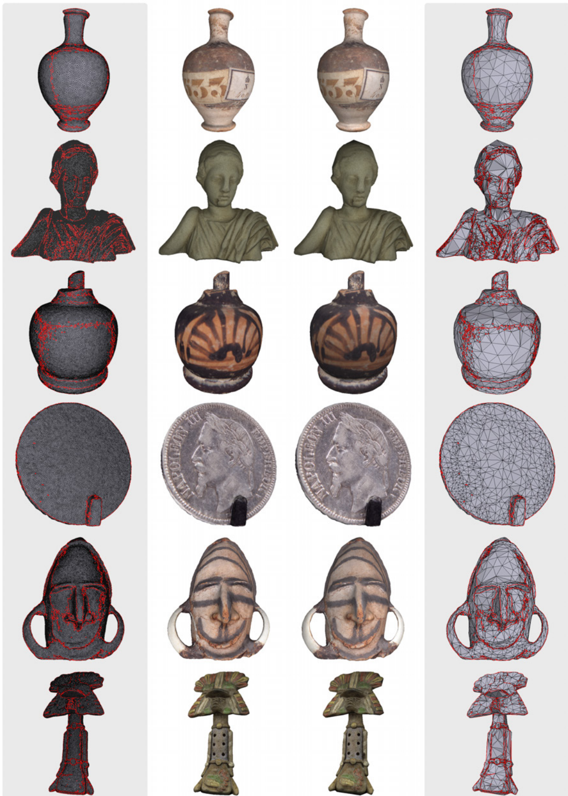
Figure 3.16: Simplification results obtained for a set of multi-chart textured models. From left to right, the two first columns correspond to the original models while the next two columns correspond to simplified models. The grey background columns illustrate the wireframes with chart boundaries depicted in red.
