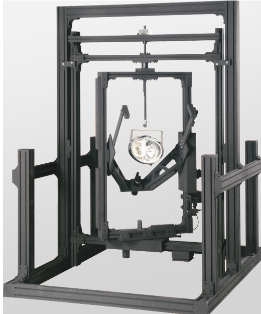
Figure 3.1: Gonio-photometer RiGO [Rad] used to capture the rayset from the light source
