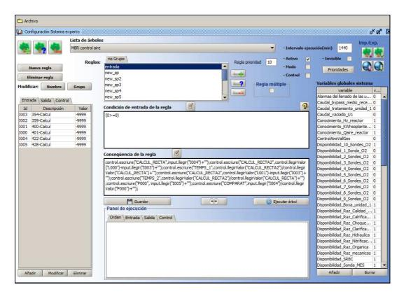
Figure 8.2. Control system screen shot: entry variables (left) and rule condition/consequence panels (centre).
