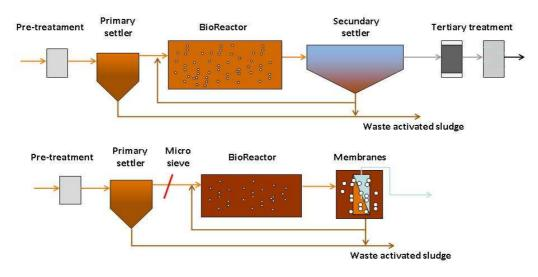
Figure 3.1. Simple scheme of a conventional activated sludge system with tertiary treatment (top) and a membrane bioreactor system (bottom).
