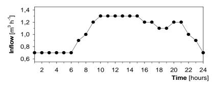
Figure 6.1. Daily flow pattern of variable flux entering the MBR pilot plant and treated during the project.
