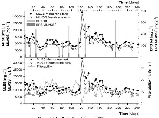
Figure 6.14: MLSS, filterability and EPS evolution.
