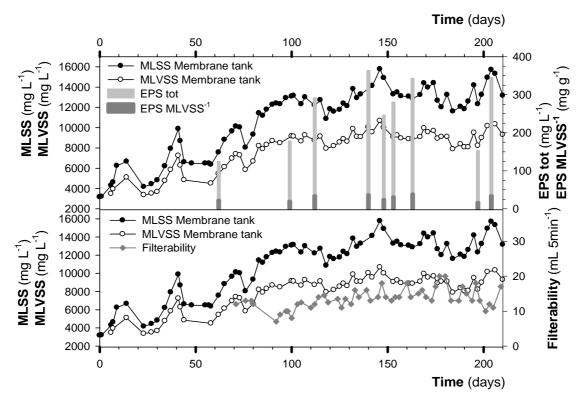
Figure 6.8. MLSS, filterability and EPS evolution.
