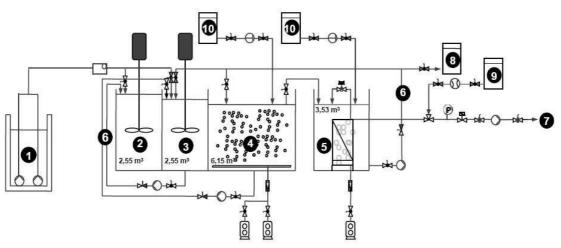
Figure 5.2. Pilot plant scheme: 1. Influent pumps; 2. Anaerobic tank; 3. Anoxic tank; 4. Aerobic tank;
