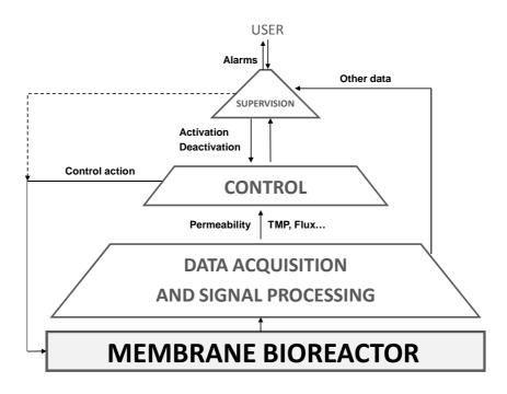
Figure 7.1. Multilevel structure of the control system.
