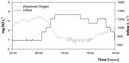
Figure 6.4. Dissolved oxygen profile in the aerobic chamber and inflow profile.
