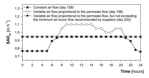
Figure 6.7. Different air flow patterns in operation during the study.
