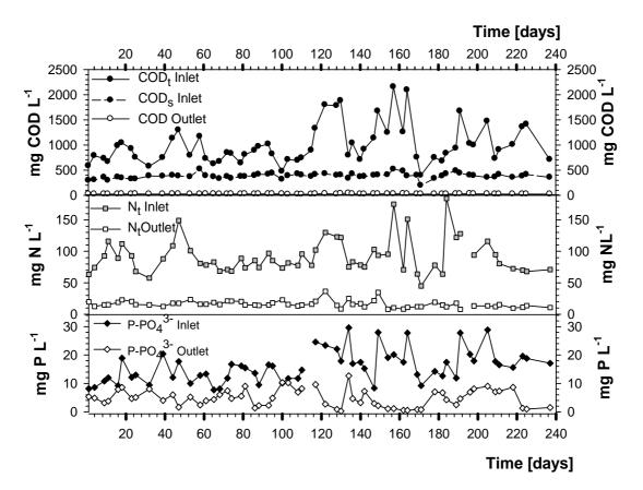
experimentation. Nonetheless, an average P removal efficiency of 65% was achieved. Figure 6.10 shows BNR performance during the entire experimental run.
