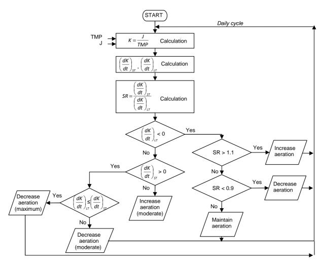
Figure 7.3. Decision tree for the aeration control algorithm.
