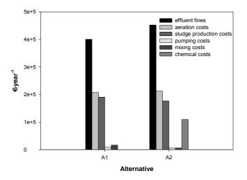
Figure 5.9. Breakdown of the operating costs (X<sub>3</sub>) for the most promising alternatives.
