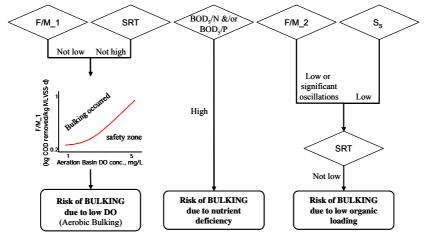
Figure A4.1. Flow diagram developed to evaluate the risk of filamentous bulking.
