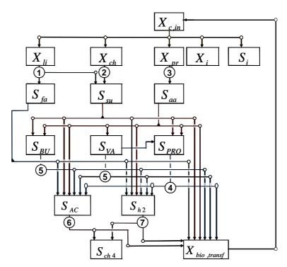
Figure 3.5. Representation of the biochemical reactions in the anaerobic digestion model (ADM1): (1) acidogenesis from sugars, (2) acidogenesis from amino acids, (3) acetogenesis from LCFA, (4) acetogenesis from propionate, (5) acetogenesis from butyrate and valerate, (6) aceticlastic methanogenesis and (7) hydrogenotrophic methanogenesis (from de Gracia *et al.*, 2007)
