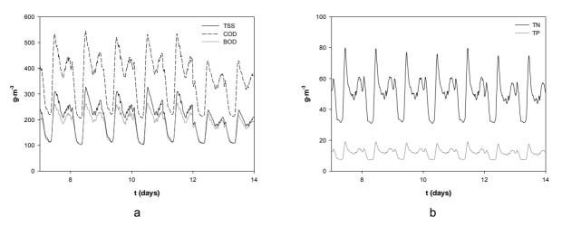
Figure 5.2. Influent wastewater organic matter (COD and BOD<sub>5</sub>) and TSS a) and nutrients (N,P) profile.
