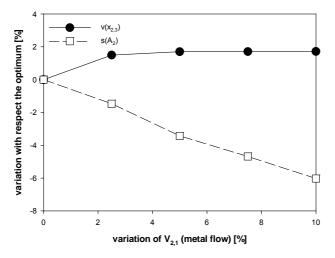
Figure 5.11. Trade-offs between the multiobjective function  $s(A_2)$  and the normalized value of criterion robustness  $x_{2,3}$ .
