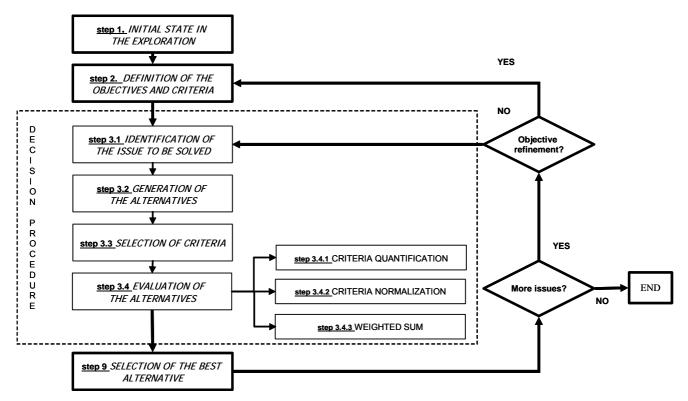
Figure 4.1. Flow diagram of the first block of the conceptual design method (see text for explanations)
