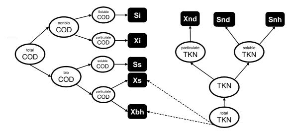
Figure 7.3. Illustration of the influent fractionation procedure and the assumed parameters in the fractionation
