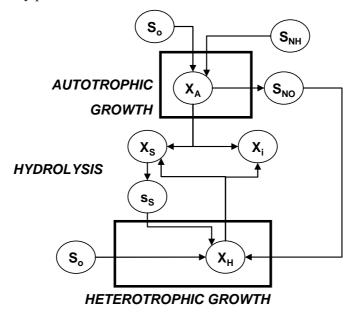
Figure 3.1. Substrate flow for autotrophic and heterotrophic biomass in ASM1 (Gernaey et al., 2004)
