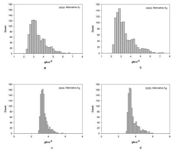
Figure 7.5. Histograms of the effluent TKN variation when alternative  $A_1$  (a),  $A_2$  (b),  $A_5$  (c) and  $A_6$  (d) are evaluated under ASM parameter uncertainty
