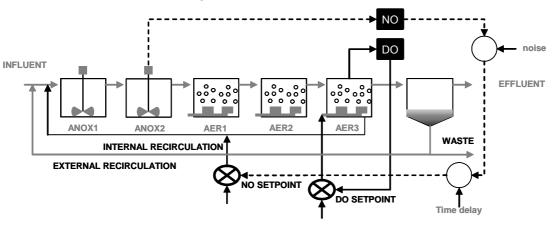
Figure 4.7. Schematic representation of the activated sludge plant with controllers
