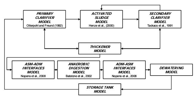
Figure 3.4. Schematic representation of the different models at plant wide level
