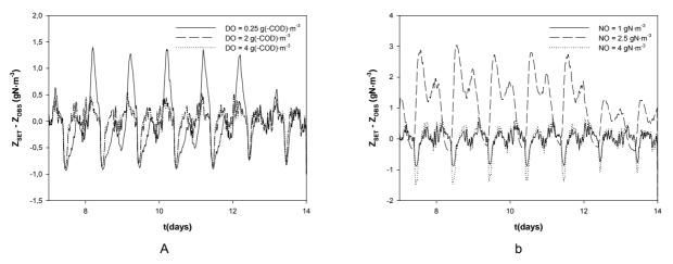
**Figure 4.10**. Dynamic profiles of the difference between the nitrate in the second anoxic reactor ( $Z_{OBS}$ ) and the desired set point ( $Z_{SET}$ ) for different set point combinations a) when the NO set point is constant (NO = 1 g N·m<sup>-3</sup>) and DO is changed and b) when the DO set point is constant (DO = 2 g (-COD)·m<sup>-3</sup> and NO is changed
