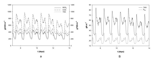
Figure 7.2. Influent wastewater a) organic matter (TSS, COD and BOD<sub>5</sub>) and b) nitrogen (TKN and ammonium) profile
