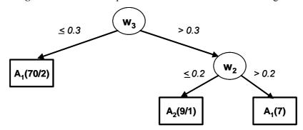
Figure 5.8. Classification tree generated with the data matrix generated during the weight sensitivity analysis.
