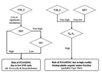
Figure A4.2. Flow diagram developed to evaluate the risk of filamentous bulking.
