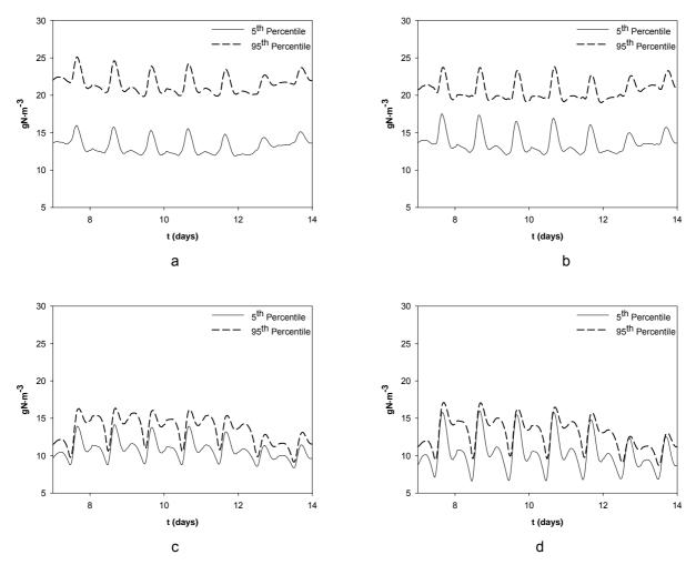
**Figure 7.8.** Dynamic uncertainty ranges for TN during the evaluation of alternative  $A_2$  (a),  $A_3$  (b),  $A_4$ (c) and  $A_6$  (d) under ASM parameters uncertainty. The TN profiles corresponding to the 5<sup>th</sup> and the 95<sup>th</sup> percentile resulting from the Monte Carlo simulations are shown.
