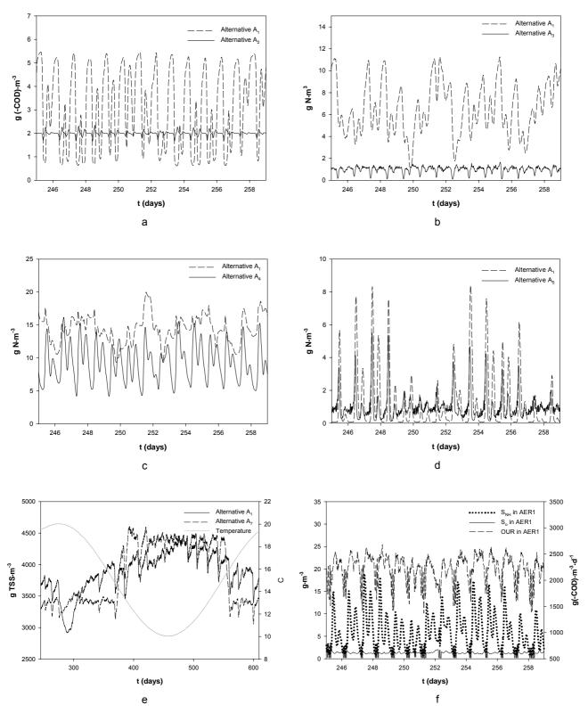
**Figure 6.4.** Behaviour of the different controllers studied: (a)  $S_o$  controller, (b)  $S_{NO}$  controller by means of the manipulation of  $Q_{intr,}$  (c)  $S_{NO}$  controller by means of manipulation of  $Q_{carb}$ , (d)  $S_{NH}$  controller, (e) TSS controller and f) OUR controller
