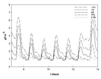
Figure 5.5. Evolution of the total phosphorus concentration in the effluent for the different scenarios: alternative  $A_1$  analysing the variable ( $V_{1,1}$ ).
