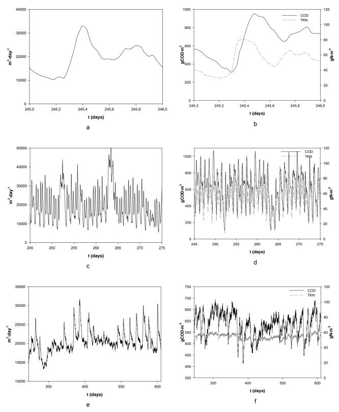
**Figure 6.3.** Influent wastewater flow (a,c,e) and components (b,d,f) for one day, (a,b) for one month (c,d) and for one year (e,f)
