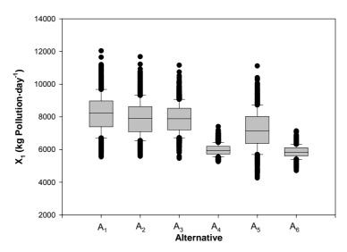
Figure 7.4. Effluent quality index (X<sub>1</sub>) variation using a multiple box plot representation.
