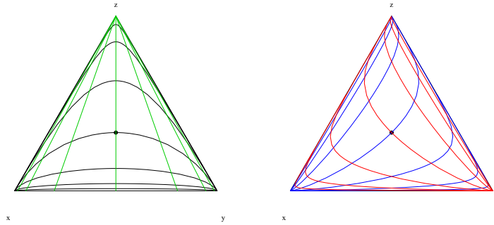
Fig. 3.2. Orthogonal grids of compositional lines in \mathcal{S}^3 , equally spaced, 1 unit in Aitchison distance (Def. 3.7). The grid in the right is rotated 45^\circ with respect to the grid in the left.
