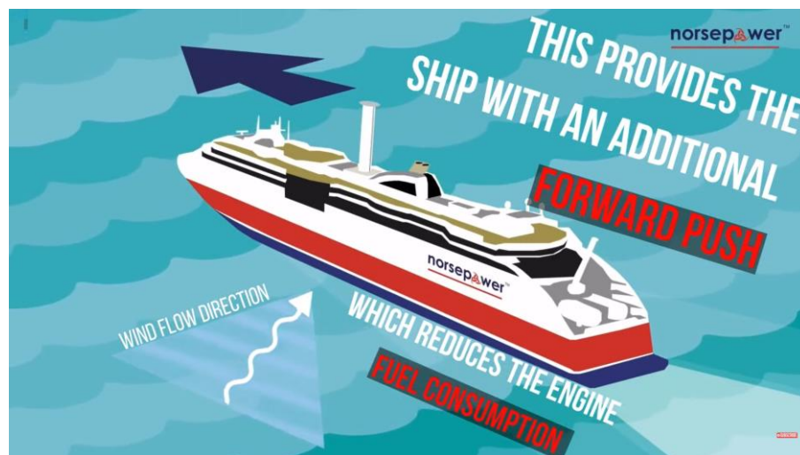
Figura 10: Funcionament del rotor Flettner (Font: https://www.youtube.com/@marineinsight )
