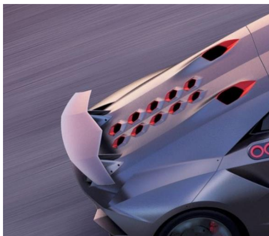
Figura 7: Perforacions hexagonals Lamborghini Sesto Elemento (Font: https://www.lamborghini.com/ )
