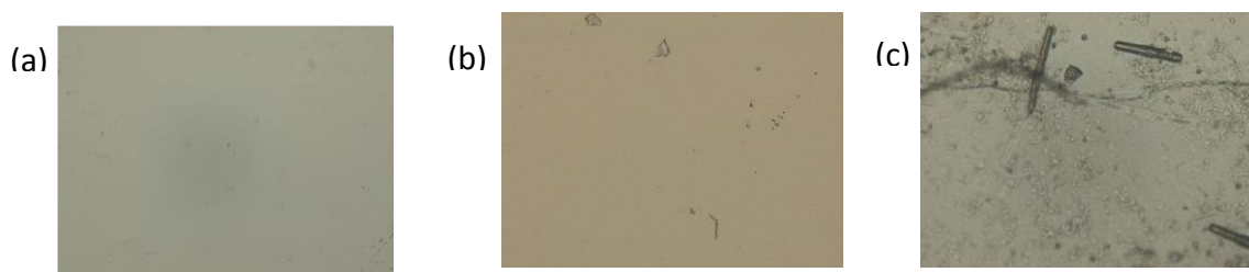
Figure 3.13. Optical microscope images (10x) of the PIM surface (a) before deployment, (b) after 7 days, and (c) after 37 days of deployment
