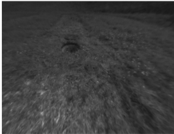
Figure 5.11: Output of the first detection algorithm showing failure to detect the occluded manhole
