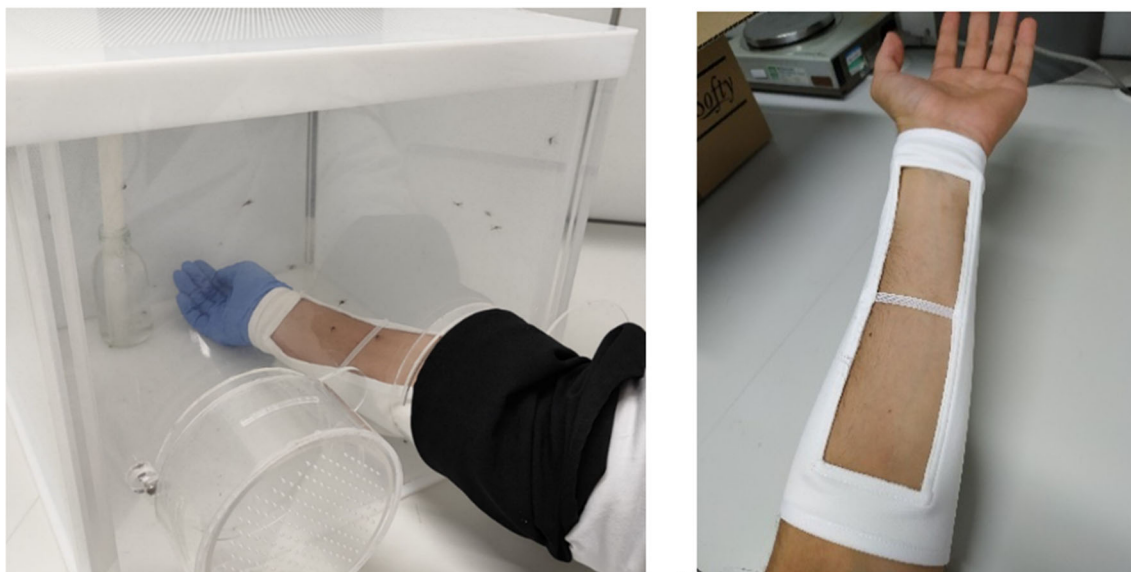
Figure 1. Sleeved arm-in-cage test (0.040-m 3 ) where 100 cm 3 of skin was exposed.
