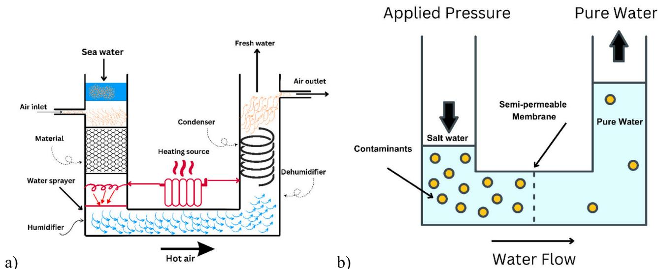
Fig. 3. a) Thermal based system and b) Membrane based system.
