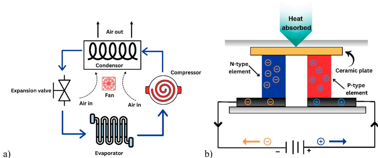
Fig. 5. a) Vapor compression system and b) Thermoelectric cooling system.
