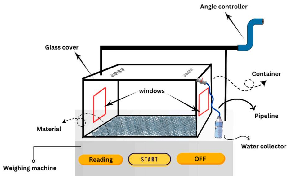
Fig. 9. Water harvesting by fiber-reinforced box setup (Reprinted with permission from (Kumar and Yadav, 2015) Copyright AIP Publishing).
