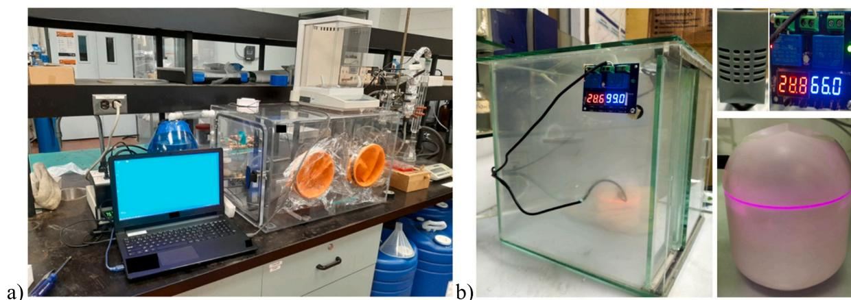
Fig. 10. Custom-made Automated Environmental Chamber (Reprinted with permission from (Legrand et al., 2021). Copyright American Chemical Society, and b) Atmospheric water harvesting plant (Ehtisham et al., 2024).
