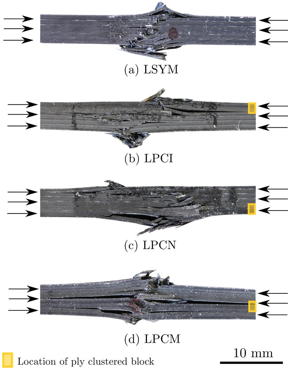
Figure 13: High resolution macro photos of the specimen edges showing the final CAI failure state of all four laminates (location of the clustered block is shown by the yellow box).
