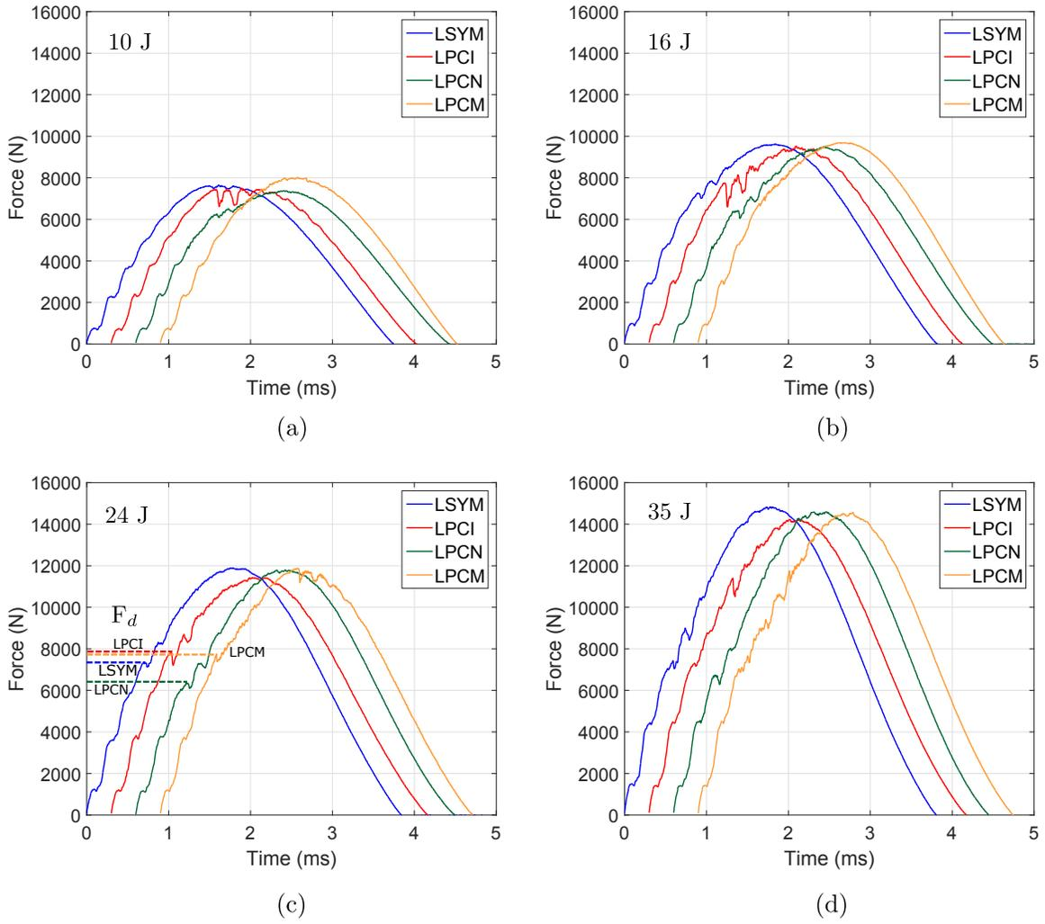
Figure 3: Impact force-time response curves of all laminates for all impact energies (Note that the responses of LPCI, LPCN and LPCM are offset by 0.3, 0.6 and 0.9 ms from LSYM, respectively, for proper comparison)
