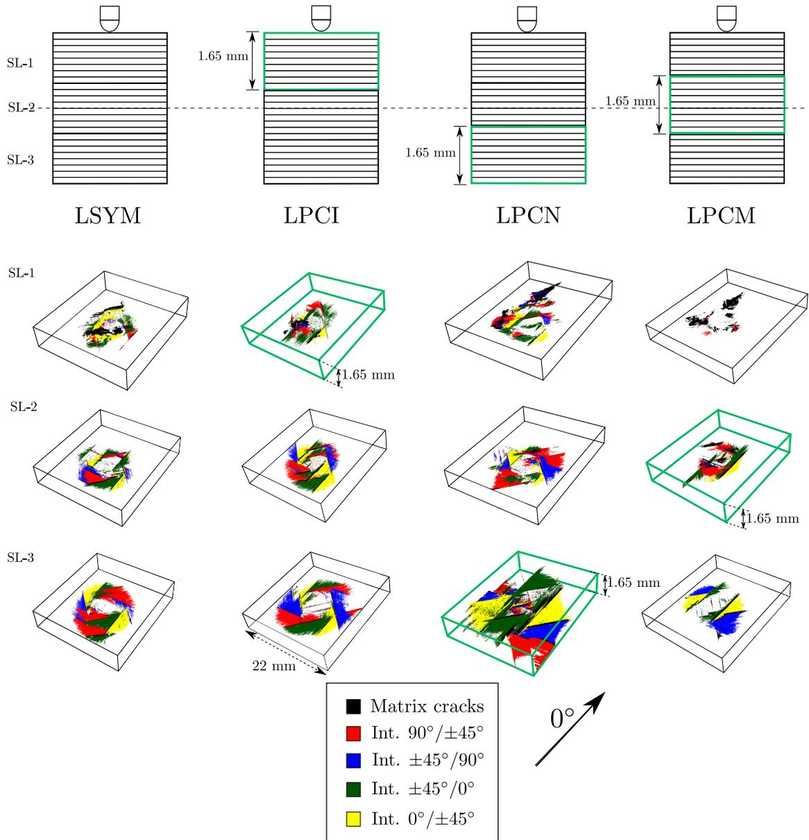
Figure 9: A 3D extruded illustration of the damage obtained from the post-processed  $\mu$ CT slices of the 10 J impact. Each laminate is divided into three sub-laminates and the sub-laminate containing the clustered plies of each unsymmetrical laminate is marked by a green box.
