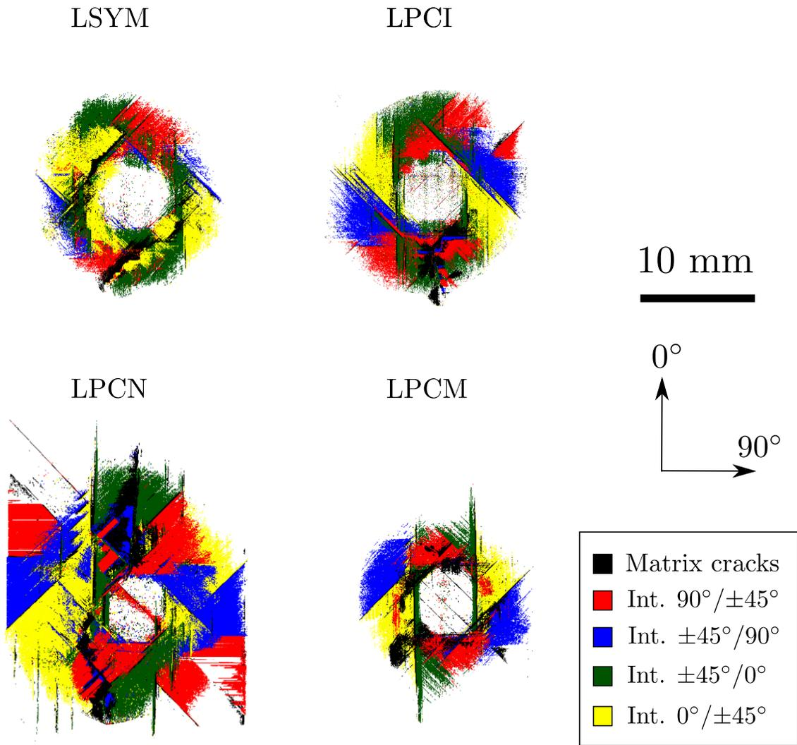
Figure 8: Projected damage footprint of all the laminates obtained from the post-processed  $\mu$ CT slices of the 10 J impact. Delaminations at different interfaces and matrix cracks are represented using colour codes as given in the legend and the represented field of view is 22 mm for all the laminates.
