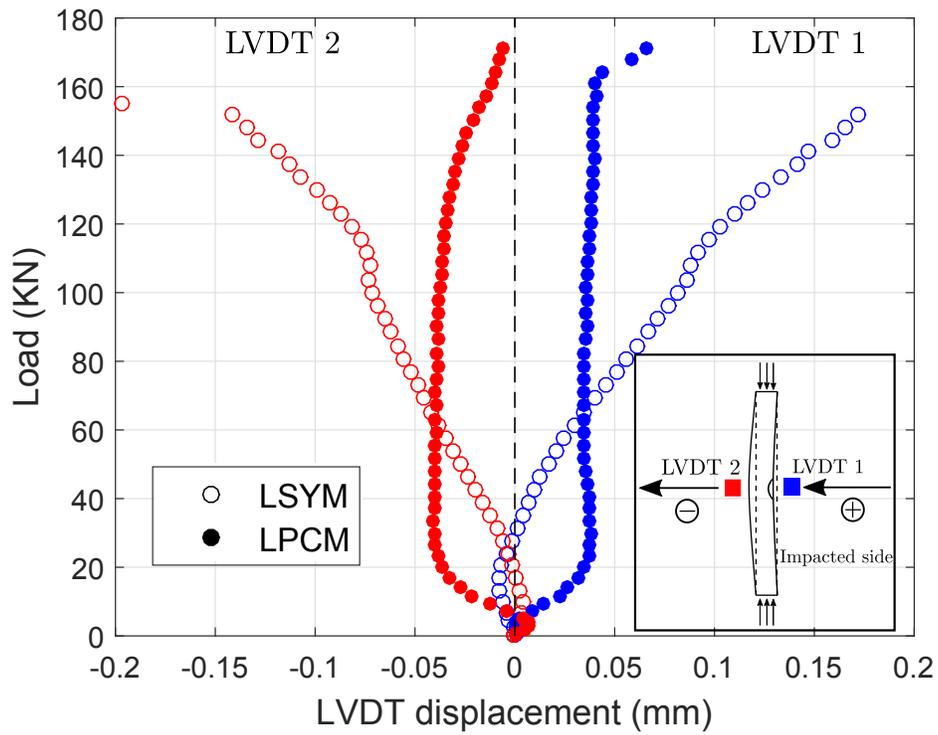
Figure 14: Out-of-plane displacements recorded by the LVDTs placed at the impacted and non-impacted face laminate centres during the CAI loading of a 16 J impact for LSYM and LPCM laminates (Note that blue indicates LVDT 1 placed at the impacted side and red indicates LVDT 2 placed at the non-impacted side. Outwards buckling (shown by the black arrows in the sub-figure) is indicated by positive values of LVDT 1 and negative values of LVDT 2).
