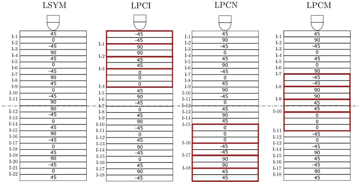
Figure 1: Illustration of all the laminates used for the study: LSYM, LPCI, LPCN and LPCM, where LPCN is obtained by flipping upside down LPCI. Note that T (top), B (bottom) and M (middle) refer to the location of the clustered block in the through-the-thickness direction of the laminate.
