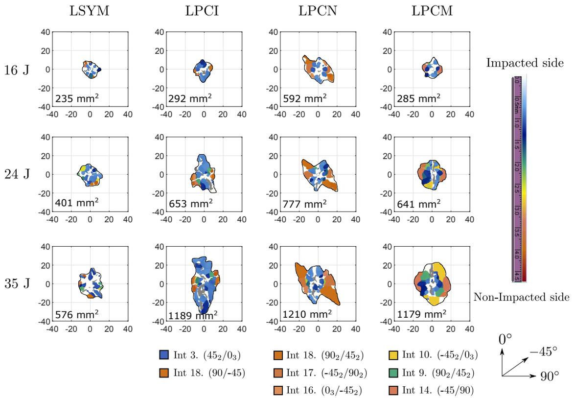
Figure 10: C-scan images of all four laminates inspected from the impacted side for the impact energies 16, 24 and 35 J. Projected delamination area is marked in the bottom left corner of each box and the field of view represented is 80 x 80 mm with the impact point as the centre.
