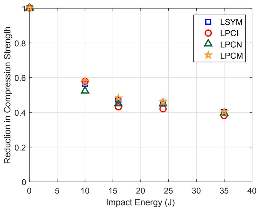
Figure 12: Normalized reduction in the compression strength due to the impact induced damage for all the impact energies.
