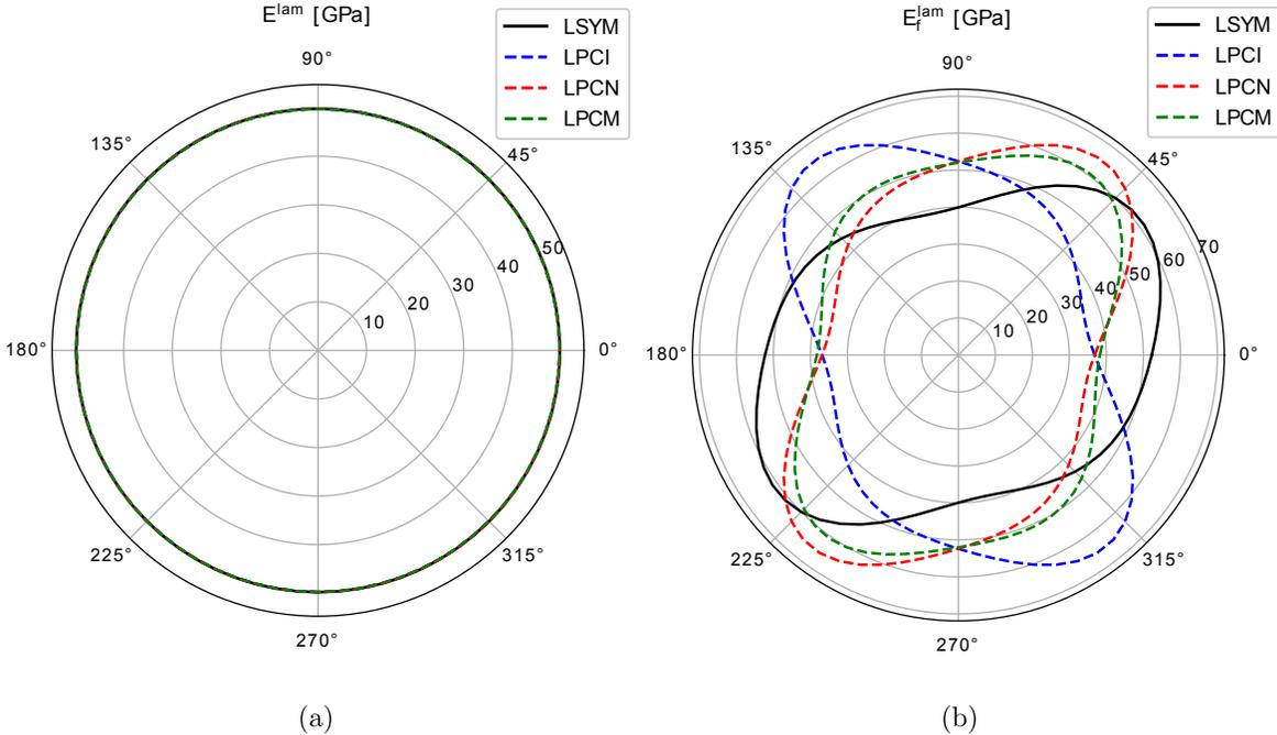
Figure 2: Polar plot representation of the (a) in-plane stiffnesses and (b) bending stiffness of all the laminates.
