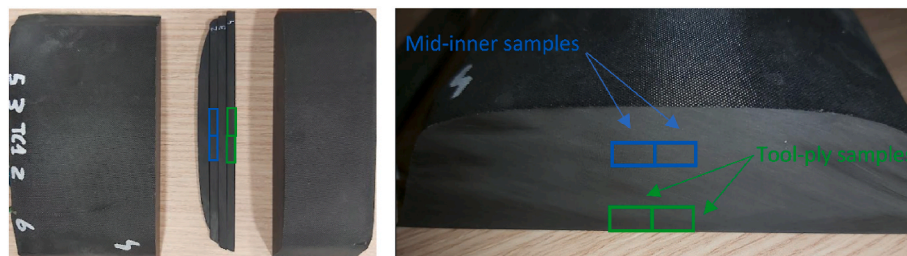
Fig. 3. Location of the samples extracted to determine T_g by DSC.
