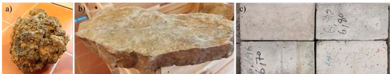
Figure 1. Different stones investigated: (a) volcanic stones from Garrotxa; (b) sedimentary stones from Empordà; and (c) concrete parallelepipedal units.
