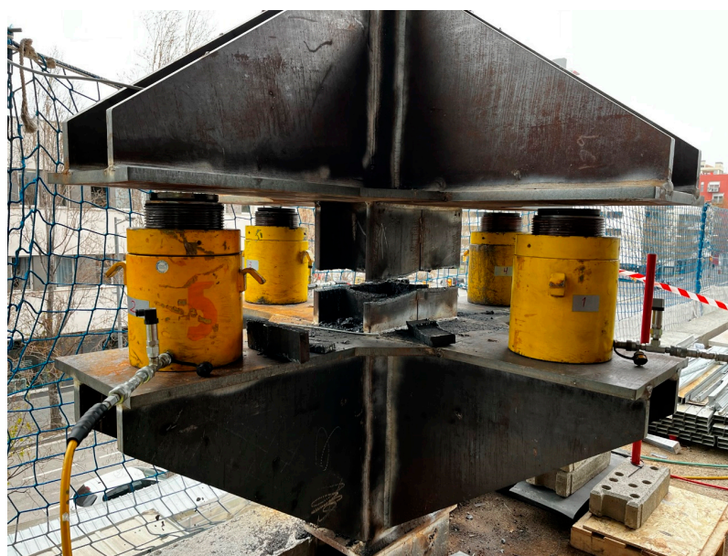
Figure 6. Image of the system after the pillar is cut and separated from the system. In the top head of each piston, a space is visible. The transducers were removed before this photo was taken.
