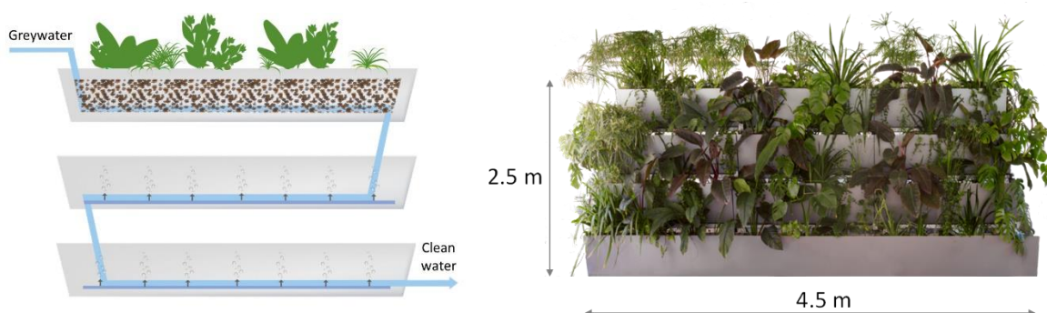
Figure 2. a) Schematic overview of the vertECO technology (patent number AT516363), all stages are planted and filled with LECA. b) Picture of the system installed in Hotel Samba. Images retrieved from Alchemia-nova website ( https://www.alchemia-nova.net/products/verteco/ ).
