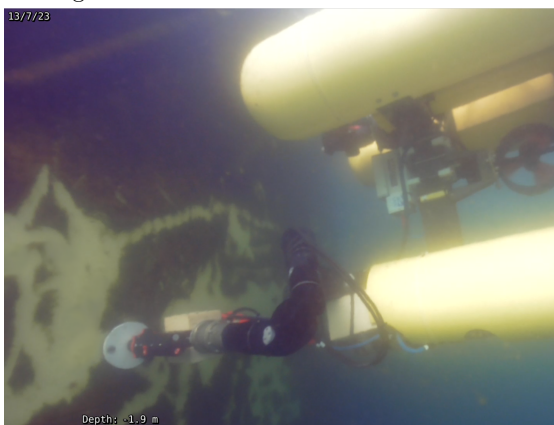
(c) The robot performs cleaning while coupled with the structure.
