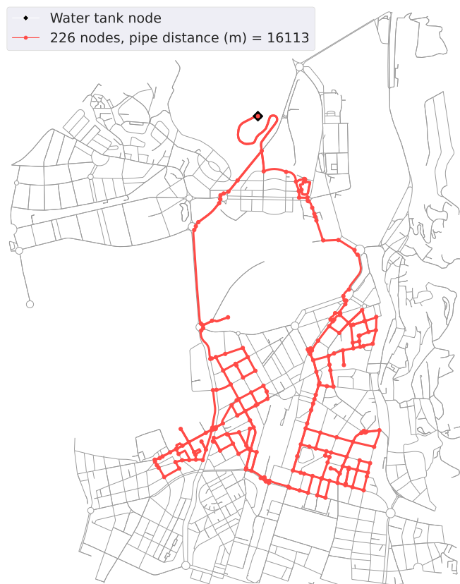
Fig. 2. Visualization of the ‘resilient-by-design’ €1,500,000 reclaimed water network in Girona (highlighted in red) overlaying the Girona street graph (in grey).
