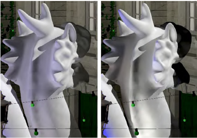
Figure 15: Irradiance filtering can lead to light leaks in certain situations on dynamic objects, as shown in these details from the Bistro scene. Left: A blue tint is visible on the dragon's body and slightly on the back of its head due to irradiance filtering from neighbouring voxels that have visibility to geometry from the dragon's blue body part, shown in Figure 1. Right: Disabling irradiance filtering avoids this issue but may lead in some cases to some extra-darkening.
