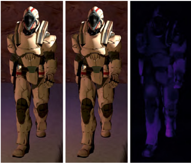
Figure 6: Details from a different viewpoint for the Rocks scene with a voxelization resolution of 128^3 . Left: Using a 5^3 neighbourhood for dynamic voxels, running at 124 fps with 721 dynamic visible voxels. Centre: Scene without any neighbourhood for dynamic voxels, running at 137 fps with 61 dynamic visible voxels. Right: Difference image between the two images using NVIDIA's FLIP [ANAM*20] tool.
