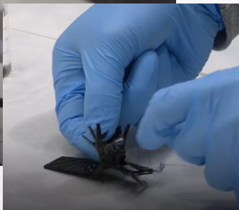
Recycling process of carbon-fibre composite materials with vitrimer matrix
