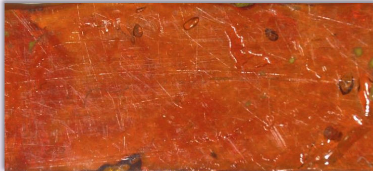
Self-healing process after 1 h, 160 °C, and no external pressure
