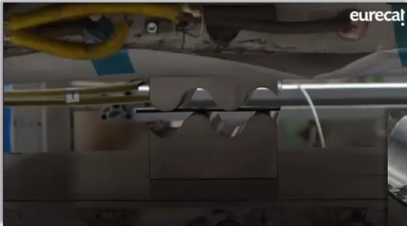
Re-shaping of carbon-fiber composites through hot-pressing
