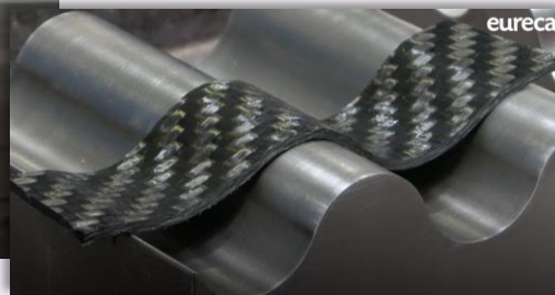
Re-shaping of carbon-fiber composites through hot-pressing
