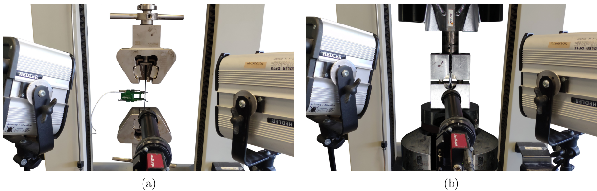
Figure 4.1.: Experimental setup of the transverse tensile (a) and compressive (b) tests.
