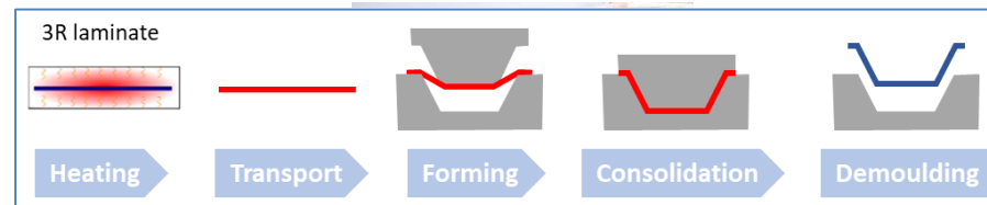
Omega-profile thermoformed with 3R-laminate at IVW
