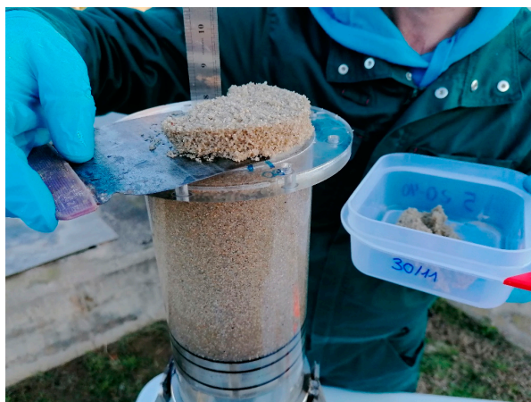
Figure 3. Removal of the bed slices after an experiment carried out in the WWTP.
