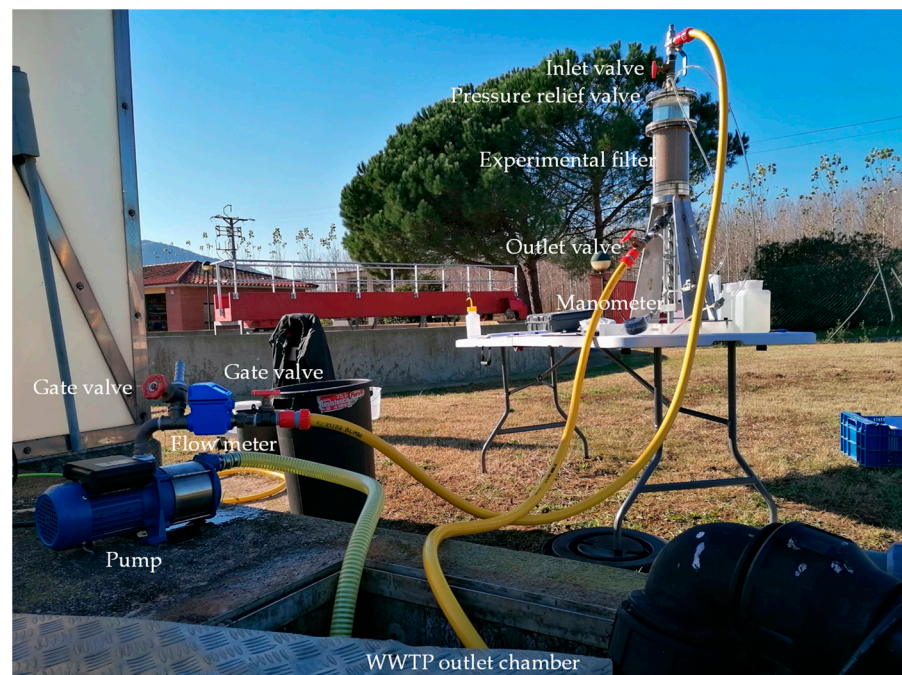
Figure 2. Experimental setup prepared for filtration mode tests placed at the wastewater treatment plant.
