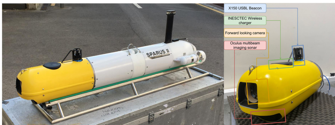
FIGURE 1 On the left, photography of the Sparus II AUV with the ATLANTIS project configuration. On the right, payload developed by Iqua Robotics that includes X150 USBL Beacon from Blueprint Subsea (Blueprint Design Engineering Ltd, n.d.b), Wireless charger prototype from INESC TEC, forward-looking camera from Iqua Robotics, and an Oculus M-Series from Blueprint Subsea (Blueprint Design Engineering Ltd, n.d.a).
