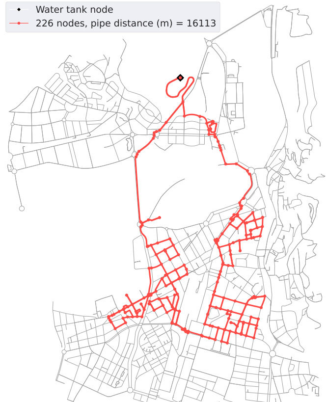
Fig. 2. Visualization of the ‘resilient-by-design’ €1,500,000 reclaimed water network in Girona (highlighted in red) overlaying the Girona street graph (in grey).
