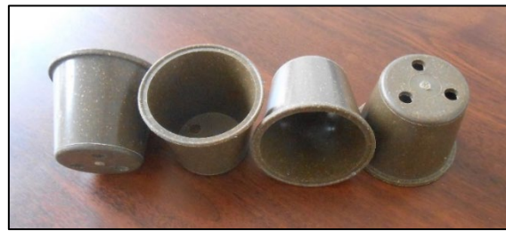
Figure 11. Example of flowerpot injected from the PHB-DFBF-30 composite material.
