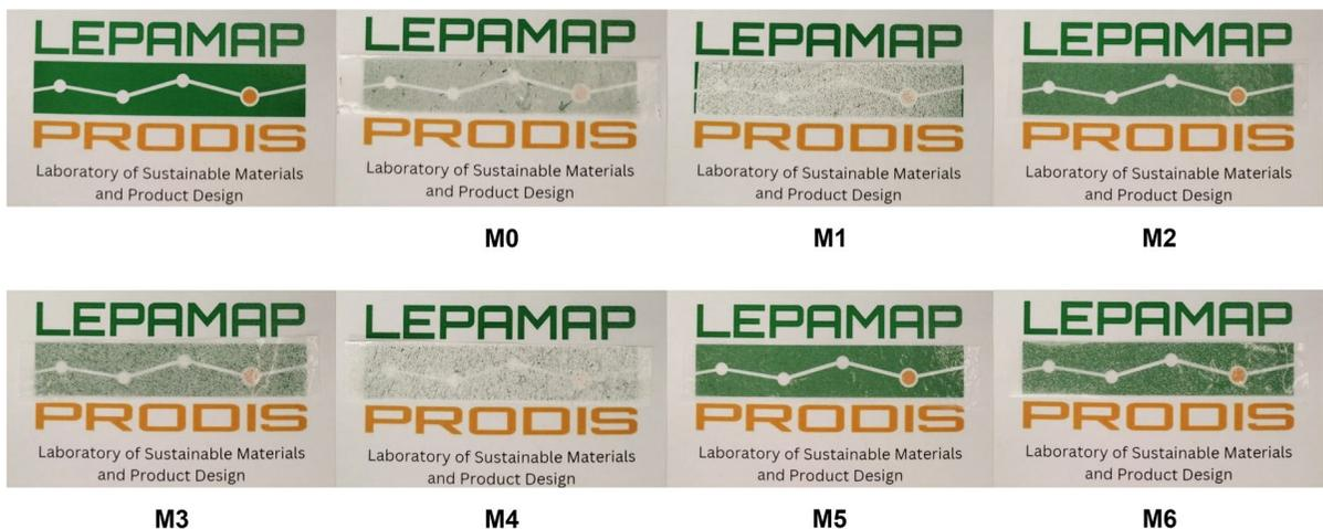
**Fig. 2** Photographs of the membranes placed on a piece of paper. The paper used is also shown
