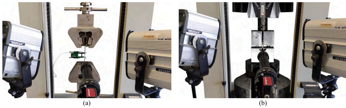
Fig. 1. Experimental setup of the transverse tensile (a) and compressive (b) tests.
