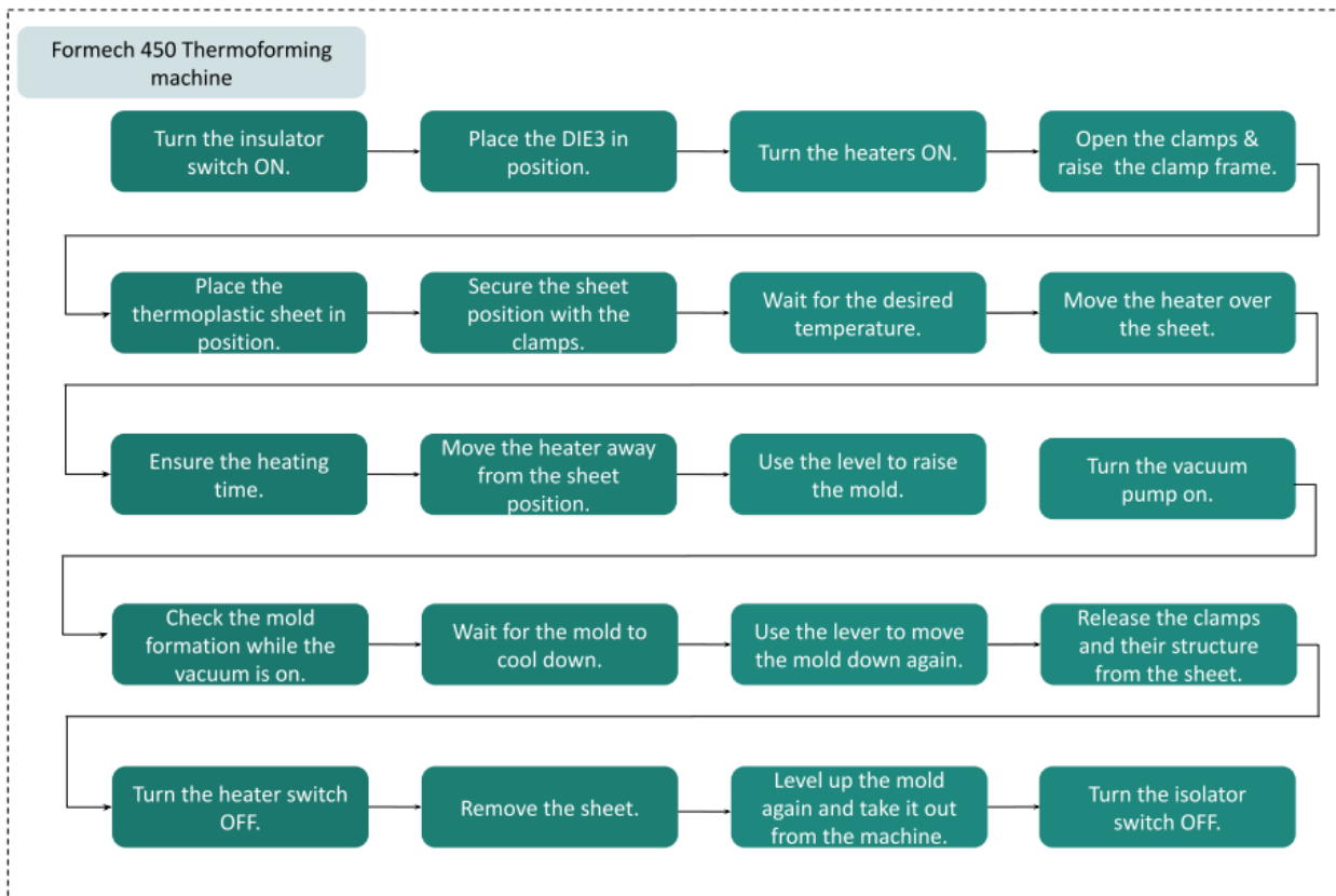
Process diagram 1. Thermoforming process
