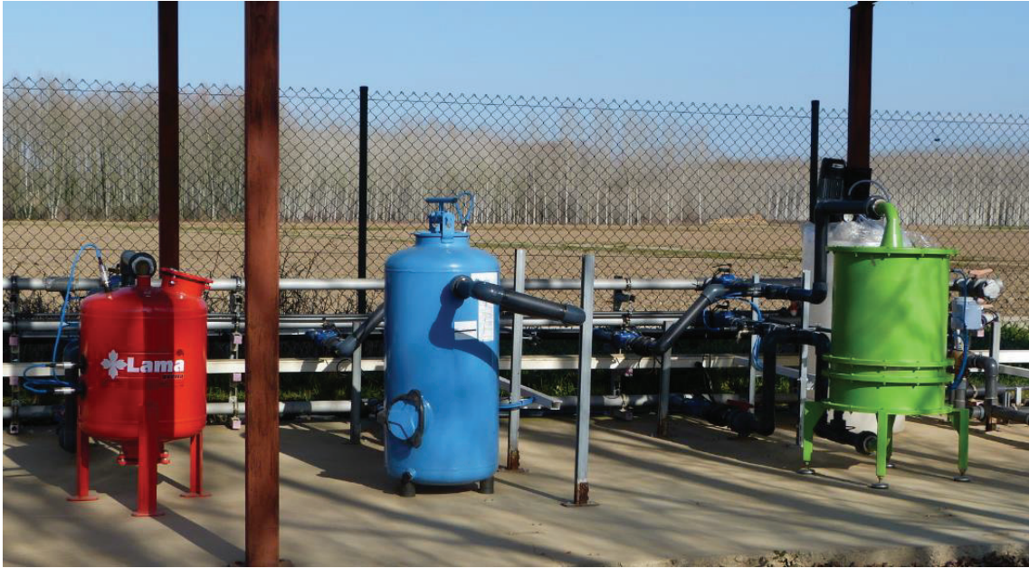
Fig. 1 - Picture of the experimental set-up with the three filter designs: (a) red: arm collector; (b) blue: inserted domes; and (c) green: a porous media prototype.
