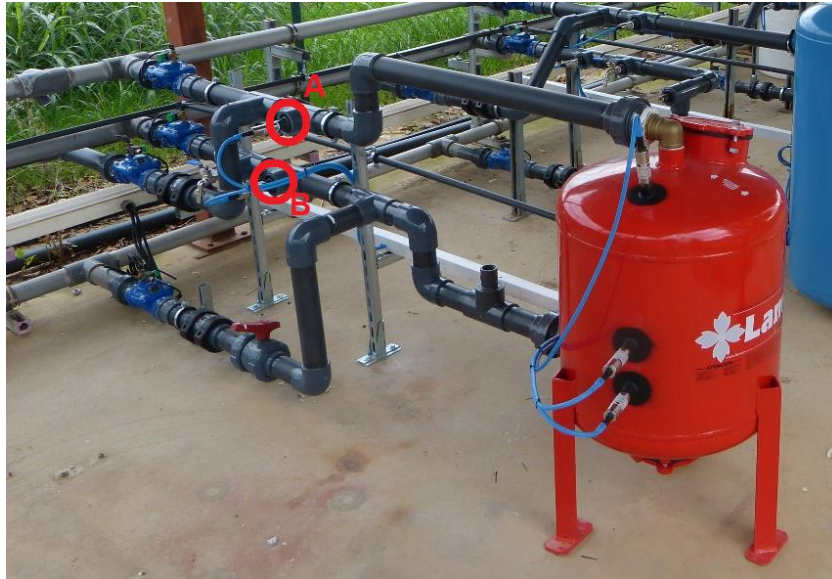
Fig. 1 - View of the experimental setup. A and B indicate the location of the pressure transmitters before and after the filter, respectively, in filtration mode.
