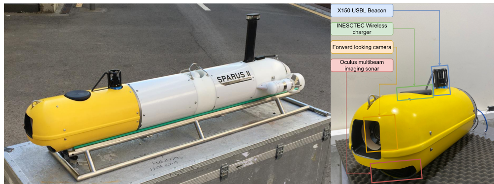
Figure 1: On the left, photography of the Sparus II AUV with the ATLANTIS project configuration. On the right, payload developed by Iqua Robotics that includes X150 USBL Beacon from Blueprint Subsea (Blueprint Design Engineering Ltd, b), Wireless charger prototype from INESCTEC, forward-looking camera from Iqua Robotics, and an Oculus M-Series from Blueprint Subsea (Blueprint Design Engineering Ltd, a).
